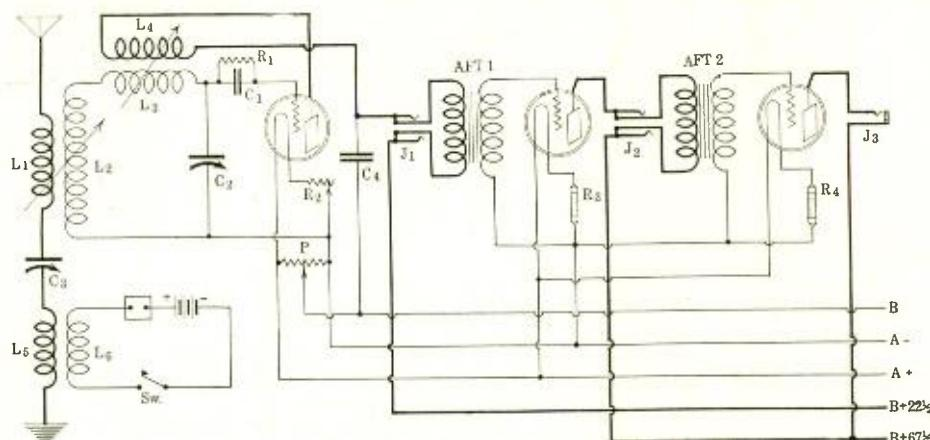
FIG. 1, showing the electrical diagram of the Marconi Receiver. Note the buzzer tester in the extreme left of the diagram. This part of the set is optional.
