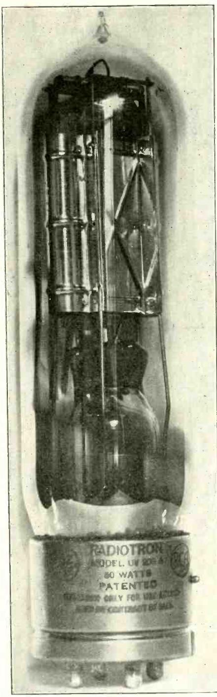
FIG. 1, showing the new UV203A, which only takes 3.25 amperes on the filament, although a 50-watt tube.
