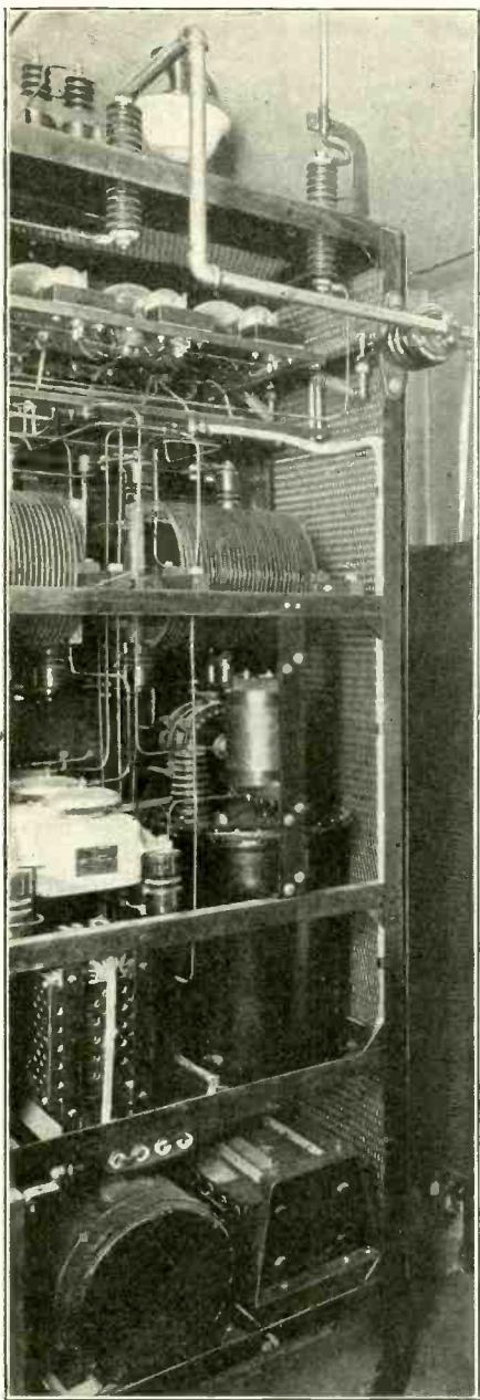
FIG. 4, the back of the 500-watt phone transmitter at WRC. Note the inductances in the fourth rack and heavy insulators on the top of the transmitter, also the large condensers in the third rack.
