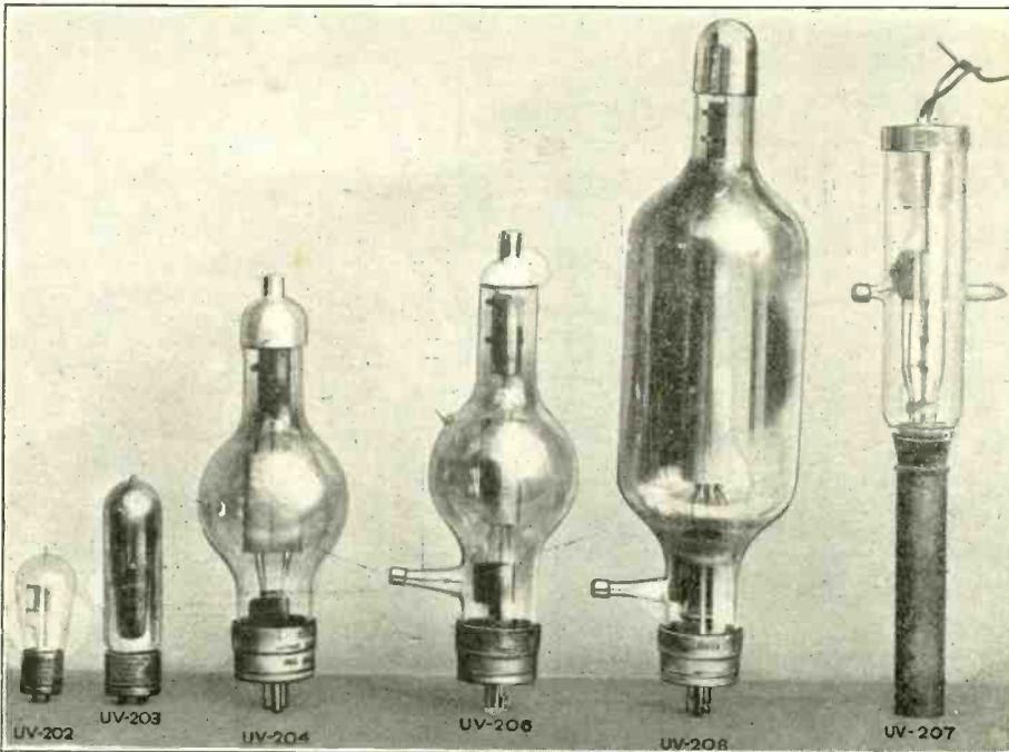
FIG. 3, showing the six different sizes of tubes used in commercial and amateur circles. The UV202 is the 5-watter, UV203 is a 50-watter (old style, filament ampeers, 6.50); UV204, a 250-watter; UV206, a 1,000-watt tube; UV208, a 5,000-watt tube. The UV207 is a water-cooled tube, with an output of 20 kilowatts.
