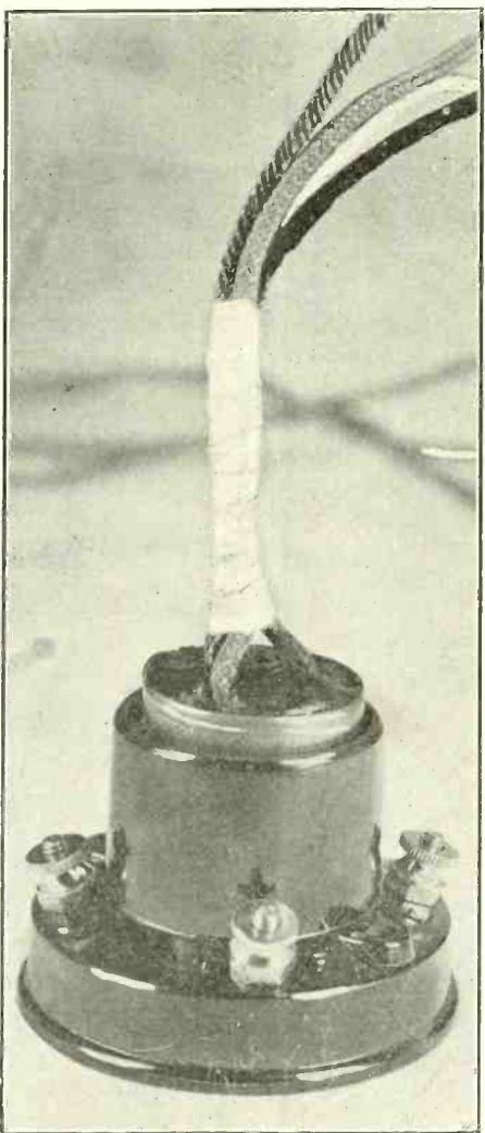
FIG. 5, the finished product, a serviceable battery connector. Vari-colored battery cable may be used to advantage for easier distinction of the leads.
