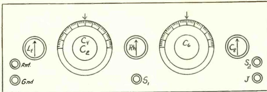
FIG. 2, the suggested panel layout of Anderson's 6-tube Super-Heterodyne.
