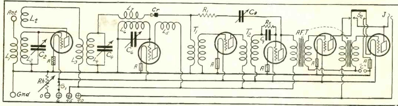
FIG. 1, the circuit diagram of the Baby Super-Heterodyne, using two audio stages.
