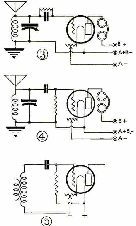
CORRECT ways of including the gridleak in a detector circuit.
