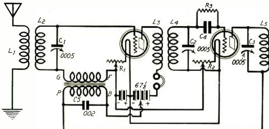
FIG. 94—The Transcontinental Reflex, two tubes operating as three. L1 and L3 are 10-turn coils wound over L2 and L4, respectively. L2 and L4 are 60-turn coils wound on a 3" form. L1 and L2, are in inductive relationship to each other as are L3 and L4. However, keep the coils L1 and L2 at a distance from L3 and L4. Short leads, high quality apparatus and good workmanship will assure you of fine results.
