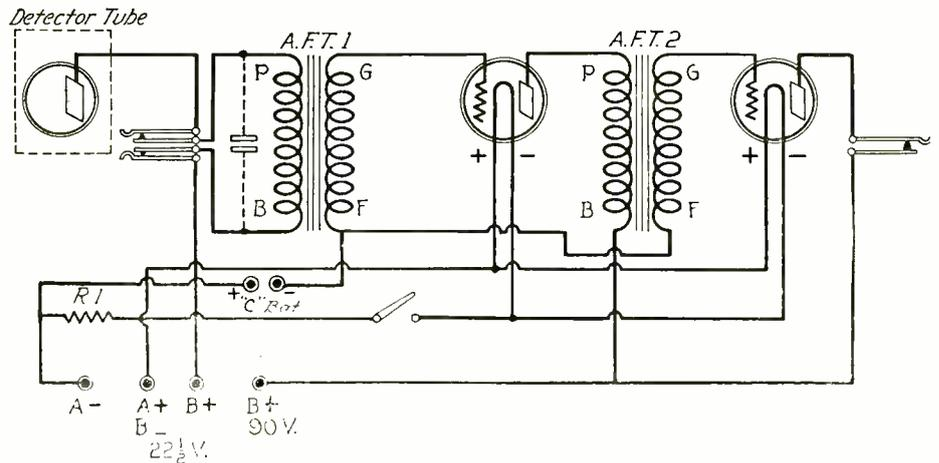
**AUDIO-FREQUENCY** amplification makes already-detected signals much louder. Two stages of transformer-coupled AF, added to any circuit (except a simple crystal set) will operate a speaker. Note how the C battery is connected. This battery is discussed in Gelula's article.
