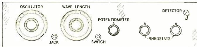
**FIG. 2**, panel layout for the 6-Tube Reflexed Super-Heterodyne.
