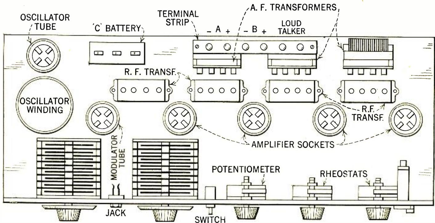
FIG. 3, assembly plan of Benson's Super-Heterodyne, with the parts designated.
