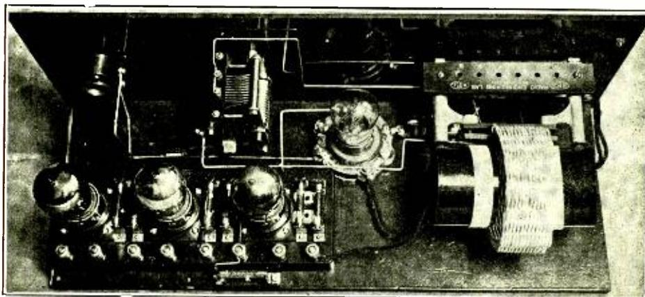
FIG. 2, the completed circuit. The tuning coil is at left and has two variable factors, the adjustable primary and the tickler coil. The large winding is the fixed secondary, tuned by the variable condenser at right. The detector tube is at left. At right is the 3-stage resistance-coupled amplifier.
