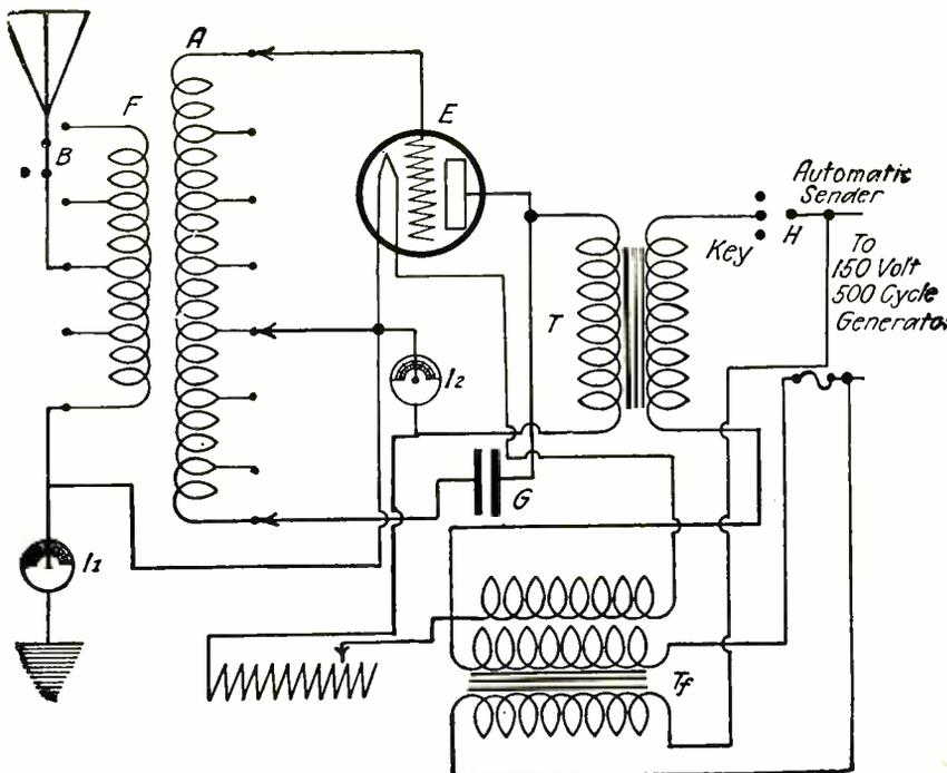
FIG. 95—Small but efficient 5-watt CW transmitter. F is a 15-turn coil wound on a 5" diameter form, tapped every third turn. A is the secondary, wound within the primary coil, and has 36-turns tapped every fourth turn. G is a 1 mfd. power condenser. T is a telephone transformer. A Ford spark coil will fill the purpose if you find it difficult to purchase a modulation transformer. A step-up transformer may take the place of the generator called for, if you have AC lighting mains.
