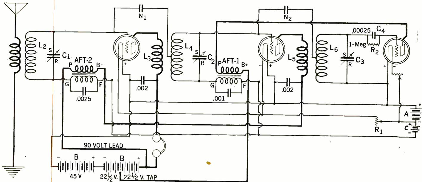
THE 3-TUBE REFLEXED NEUTRODYNE, comprising two stages of tuned RF, detector and two audio stages. As the detector output is reflexed to the second tube, whose output is reflexed to the first tube (extreme left), the inverse duplex method is employed. This makes the reflexed stages share equally the RF and AF loads. The circuit is not only for the novice to try.
