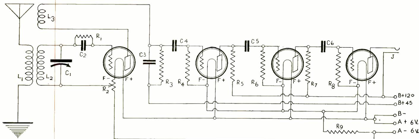
FIG. 1, wiring of the DX detector circuit, with three stages of resistance-coupled audio-frequency amplification. The coupling resistors, R3, R5, R7, are 100,000 ohms. R4, R6 and R8 are gridleaks having respective values of 1,000,000, 500,000 and 250,000 ohms. C3 is .002 mfd., C4, C5, C6 are .006 mfd. The author used the ready-made unit.
