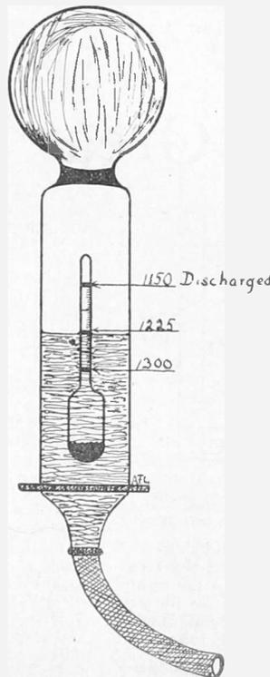
FIG. 2—Showing how to read the hydrometer. The rubber tube is placed in the storage cell and some of the electrolyte drawn into the glass tube.
