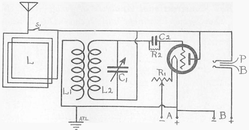
ABSORPTION LOOP (Fig. 1) used on 1-dial set. L is the loop, S1 a switch, L1L2 the tuning coil, C1 a 23-plate variable condenser, C2 a grid condenser, .00025 mfd., with leak (R2) mounted thereon; R1 is a carbon-pile or compression rheostat. A 4½-volt C battery would be used as the A battery for 199 or 299 tube. The plate voltage then should be 45 instead of the usual 22½ volts.
