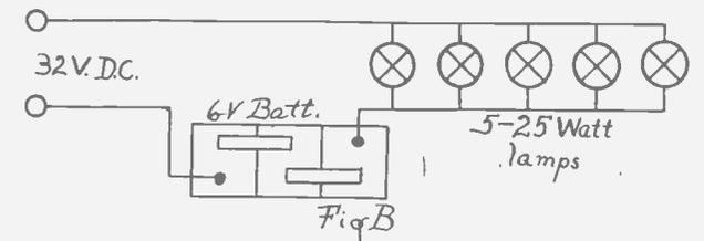
FIG. 3A—Circuit for charging the battery at home off a 110-volt direct current line. After 12 hours on the line one bulb is taken out, and one each 2 hours thereafter. This reduces the charging rate. Altogether the battery should stay on the line about 20 hours. Fig. 3B is almost identical except that it is for charging the battery on a 32-volt farm lighting generator. Always put positive to positive and negative to negative when charging.
