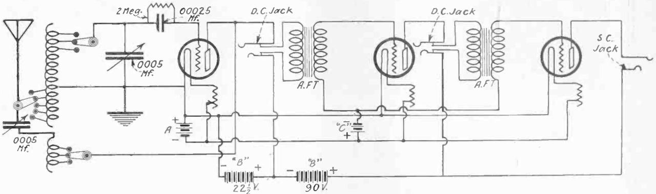
FIG. 32—Reinartz hook-up with two stages of AF amplification. One 4½-volt C battery is used for both audio stages. Excellent loud speaker volume may be had from local and distant stations with this circuit.
