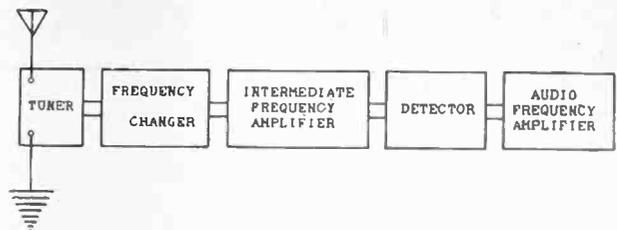
FIG. 1—How the usual type of Super-Heterodyne handles a signal, requiring two tubes for the frequency changer or eight tubes in all.
