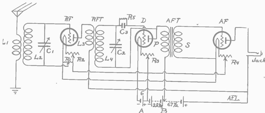
THE ULTRA-AUDION CIRCUIT, with one stage of tuned radio-frequency amplification, detector and one stage of audio-frequency amplification, designed for volume, and bringing in locals on a speaker.
