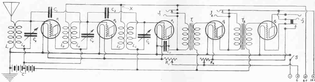
CIRCUIT NETWORK (Fig. 1) of the Simplified Neutrodyne that uses a grid-bias in the detector.  $L_1L_2$  is the tuning coil.  $L_3L_4$  and  $L_5L_6$  are the radio-frequency transformers for the two stages of such amplification.  $C_1$  and  $C_3$  are the neutralizing condensers. "Most stable and most reliable" is what J. E. Anderson, noted radio authority, says of this circuit. Five tubes are used, A1, A2, A3, A4 and A5, the last two being for audio-frequency amplification.
