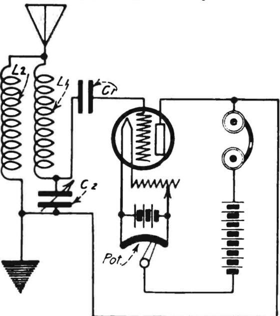
Fig. 3. Modification of Circuit 1. L1 can be a transformer but must be placed in inductive circuit with C2, which is a coil of 175 turns.
