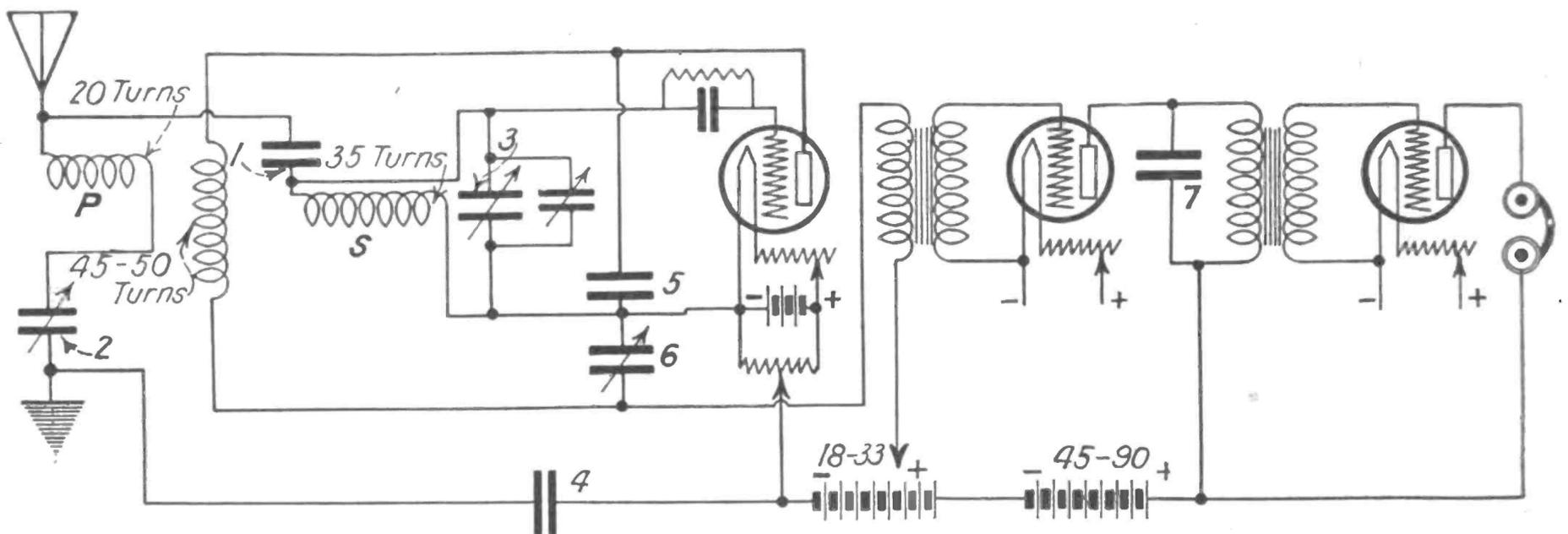
Fig. 1. Schematic diagram of the set described by H. Spencer Lewis in the accompanying article. The filament leads for the second and third tubes are left open to show that each of the tubes is supplied from separate batteries. This is done to prevent any back-coupling through the battery leads.
