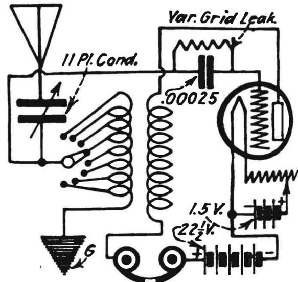
Diagram of circuit with which L. R. Dickens had accomplished marvellous results. It is a single circuit receiver using the rotor for a tickler.
