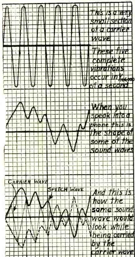
Schematic diagram showing carrier waves.
