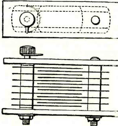
Schematic diagram showing how condenser is made.
