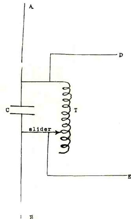
Figure 2.—A periodic filter. C, a capacity of .001 microfarads. T, a simple tuning coil. A, B, D, E, are terminals.
