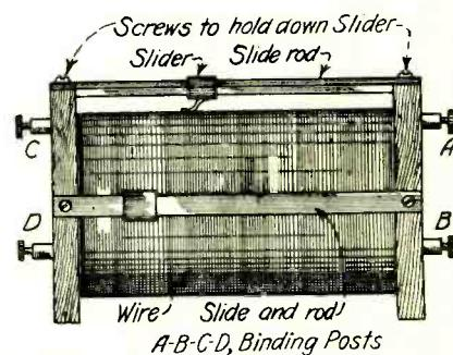
Figure 4.—A two-slide tuning coil. Particular attention should be given to the layout of both sliders, slide rods, and binding posts. Suggested by George W. May. Drawn by S. Newman.
