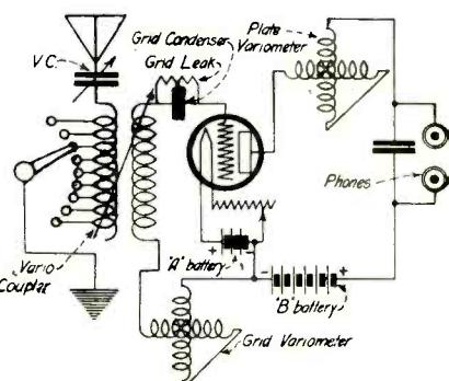
Figure 3. Schematic diagram of the wiring of the completed set. Suggested by George W. May. Drawn by S. Newman.
