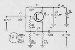
The output of the one-transistor circuit can be connected to input of an amplifier.
