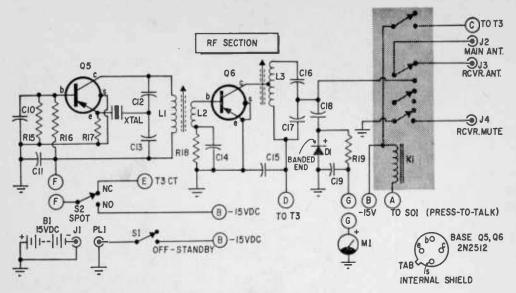
The usual high-frequency wiring techniques must be used when wiring this section of unit.
