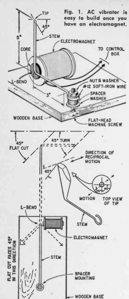
Fig. 2. Shape and position of stem point is the most important part of construction.
