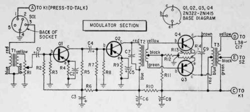
Modulator is only an audio amplifier. The main difference is in T3 secondary winding.
