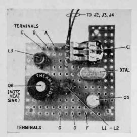
Top view of RF section (above) and the bottom view (below) have fewer components to squeeze into available space. Point-to-point wiring is used in RF stage to keep all lead lengths as short as possible thus keeping all stray capacitances lower.
