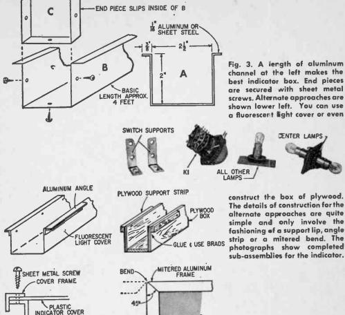
RED PLASTIC INDICATOR COVER construct the box of plywood. The details of construction for the alternate approaches are quite simple and only involve the fashioning of a support lip, angle strip or a mitered bend. The photographs show completed sub-assemblies for the indicator.
