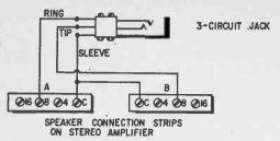
Fig. 7. Too much power from speaker output can quickly ruin these stereo headphones.
