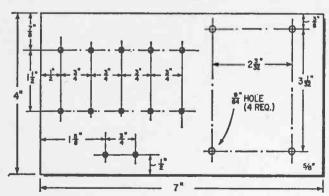
Fig. 3. Front-panel layout is for a 4- by 7-inch sloping-front cabinet. The four 9/64-inch holes on the right must be marked and drilled accurately to mate with tapped spacers. Tubular-type spacers allow more sideplay but assembly becomes a bit more difficult.
