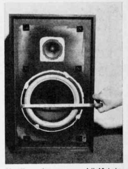
SC-440's woofer measures a full 12 inches with tweeter measuring in at 31/4 inches. Sizes indicate that this is not a "vest pocket" loudspeaker system—enclosure is actually larger than some so-called bookshelf speaker units.
