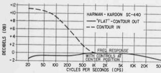
The SC-440 frequency response tested better than manufacturer's claims indicating maker's specs are true and not "dreamed up" to sell sets. With contour added over 11 db of bass boost is added to audio.
