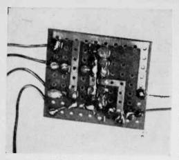
Underside of board shows solder connections between components and copper foil.
