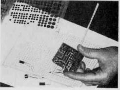
Following layout sheet, resist pattern is applied to perforated phenolic board that has been precut to size indicated on layout sheet (left). Circuit is now doublechecked. An error can still be changed. Even components should be inserted or positioned to see if they can fit the allotted space on circuit board.
