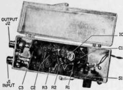
Wired out flat on a perf-board, the IC preamp fits into a plastic case. Unit is complete except for battery which is externally connected.
