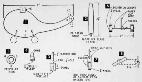
Fig. 7. Whirly-Bird construction details above and finished unit at right. Both top and rear rotors spin rapidly when the 'Bird is positioned correctly on the stem.
