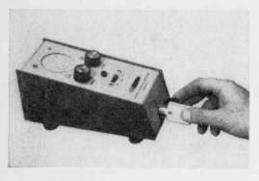
Ratio and speed controls are concentric, thereby insuring proper and consistent dot-space ratio at all keying speeds.
