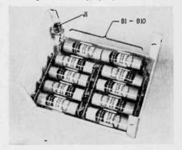
Batteries mounted in cover provide the 15volts DC. Keep contacts clean and secure.
