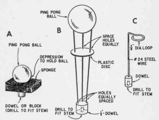
Fig. 10. Three Spin-A-Sphere adapters are different ways of doing the same thing. Any light-weight ball may be used although ping-pong ball is the easiest to find in stores.
