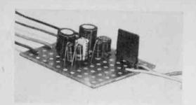
It's hard to believe that the neat little Transi-Match (above) grew from a handful of papers and a piece of perforated phenolic board (top, right) contained in a kit for making experimental printed-circuit-boards. Circuit is first transferred to polka dotted layout sheet then resist is applied to board and unwanted copper etched away.
