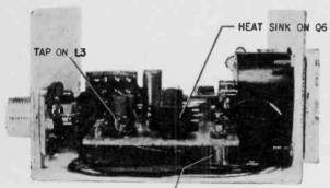
Top view of completed 6-meter transmitter is shown above and the front panel view is at its left. Beware of using miniature microphone jacks—they are delicate and can be difficult to replace in an emergency. Be sure to place heat sink on Q6 before applying power to unit.
