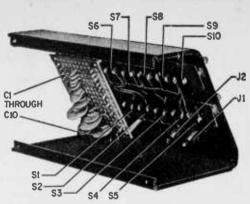
Fig. 5. Unit can be half as wide if capacitor board is mounted to cover the switches.
