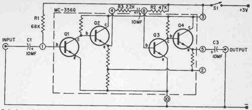
Only four of the six transistor elements in Motorola's MC356G are used in preamp's circuit.
