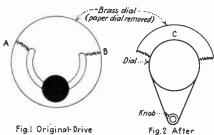
mented to the shaft. Remove the paper dial from the set by taking out the round brass clip holding it in place. Cut the slotted brass disc at A & B, shown in diagram, wrap piece of dial cable around the drum portion of dial as shown in 2. Solder in place at spot marked C and wrap two turns around spool on shaft. Splice or solder ends at C, replace paper dial and the job is done.
