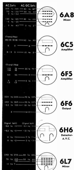
Here's a new RADIO RETAILING service chart idea designed to speed up location of set trouble 95% of all receivers using the tubes illustrated apply voltages within the limits shown
