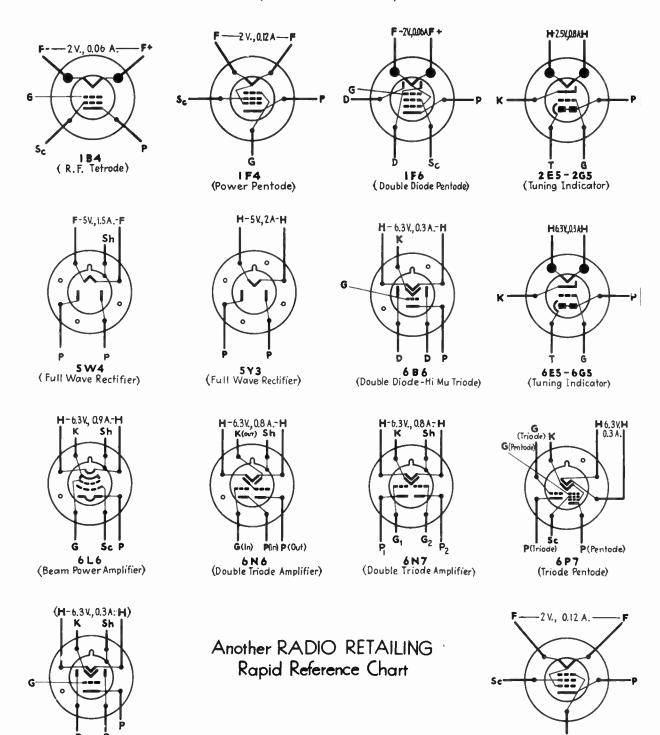
6 R 7 (Double-Diode Triode) 950 (Power Pentode)
