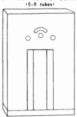
Average drain 95 Watts Average Cost 5 10-cent per hour LARGE AC TABLE MODEL
