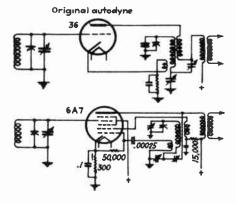
cloth covered wiring ... Substitute 6A7 for 36, employing new circuit diagrammed. The same oscillator coil is used, but the various windings employed differently. Slight retrimming of all condensers associated with circuit is all that is necessary whon revamping has been done.
