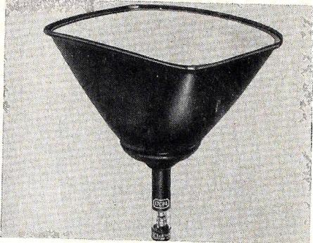
19 inches. (The 16AP4 was 22 $\frac{1}{4}$  inches long.) The tube incorporates a frosted filter-glass face plate for improved viewing, said to eliminate annoying room reflections as well as halation and reflection within the faceplate itself. A single-field ion trap is employed, as well as magnetic deflection and focus. Tube Department, RCA Victor, Harrison, N. J.—RADIO & TELEVISION RETAILING.
