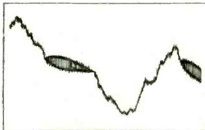
Fig. 1—Undesirable oscillation may occur anywhere on the program waveform as a bulge.
