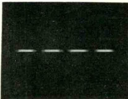
Fig. 2—Intensity modulation may be due to a defective CRT. It shows up best at low sweep rates and at reduced brightness levels.
