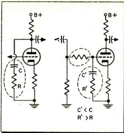
Fig. 5—High frequency response can be improved by shifting RC network from plate to grid when a grid resistor is added.
