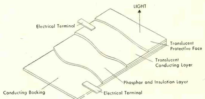
an electroluminescent lamp are very thin. For example, the two conductive layers may be separated by only a few thousandths of an inch. Varying amounts of additional thickness are, of course, required for external insulation material and for a backing panel to supply structural strength. At present, an unlighted border one-eighth to one-half inch wide is necessary on all types of panels to allow positive sealing and to prevent electrical breakdown at the edges.
