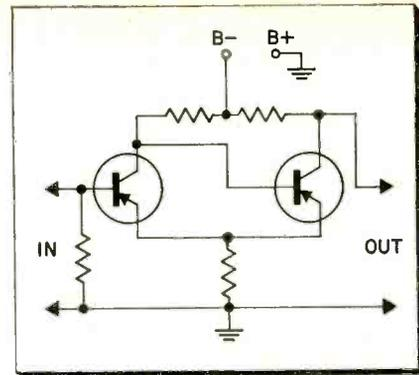
Fig. 8—The transistorized Schmitt Trigger in an electronic relay. An output is obtained when the input is of a predetermined amplitude.
