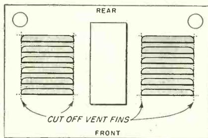
Bottom view of TV set shows fins which may be cut out so hand can pass tube through.
