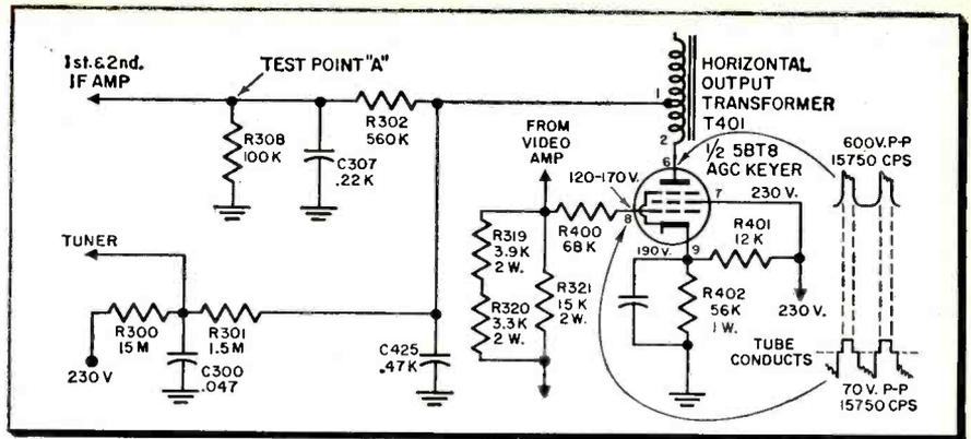
Fig. 3—Horizontal sync pulse triggers the AGC keyer tube so that the control voltage developed is proportional to the signal strength, and not to video information. Also has good noise immunity.
