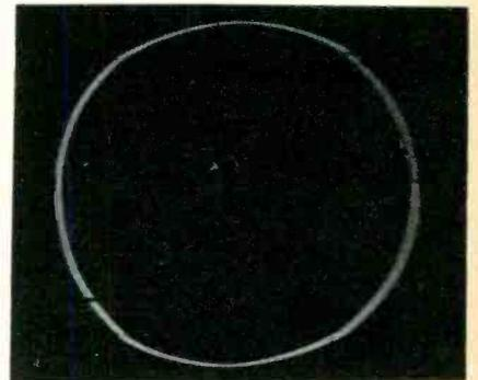
Fig. 3—Astigmatic distortion is evident by inability to focus in both the vertical and horizontal direction at the same time.
