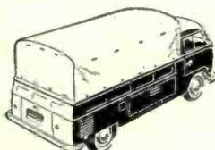
**PICK-UP**—1764-lb. payload... 45 sq. ft. floor area plus 20 sq. ft. in a lockable weather-tight compartment underneath. Sides and back drop down for easy loading.
