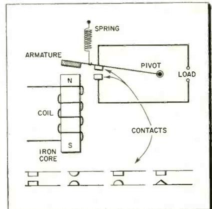
Fig. 2—Electromagnetic relay contains at least one set of contacts which may be flat, half-round, pointed or combination.
