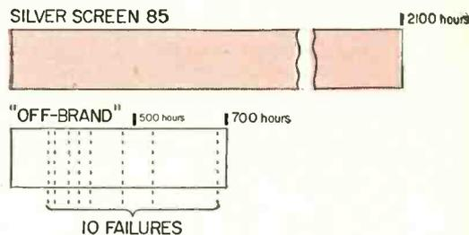
Nineteen off-brand tubes were placed on Sylvania's standard 2000-hour life test. Chart 3 tells you how fast these tubes developed slow-heating cathodes. Over half, or ten units, failed to go beyond the 700-hour mark. Small wonder then that Silver Screen 85 gives you less troublesome callbacks.
