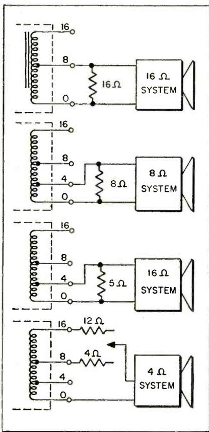
Fig. 6—Possible combinations of partial resistive loading to reduce effects of reactive load.
