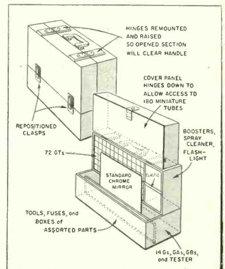
Caddy opens up instead of out when hinges and clasps are moved, saving floor space.
