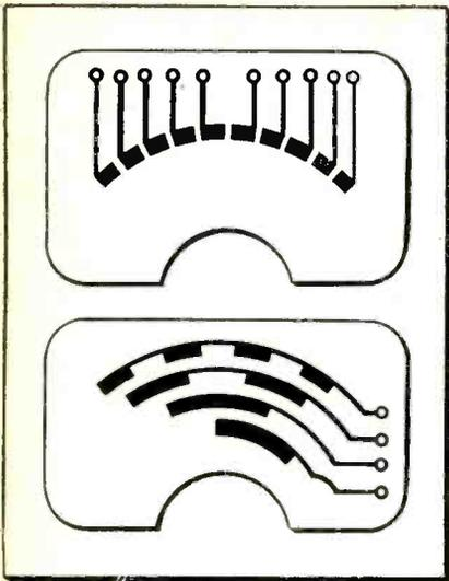
Fig. 6—A large number of switching steps is possible by using different combinations of contacts on a multicontact plate inserted in a meter relay.
