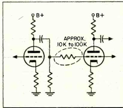
Fig. 3—Addition of a resistor in the grid circuit will help overcome grid blocking.
