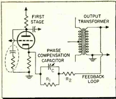
Fig. 2—High end instability can often be eliminated by slightly reducing the amount of feedback or inserting RC network.
