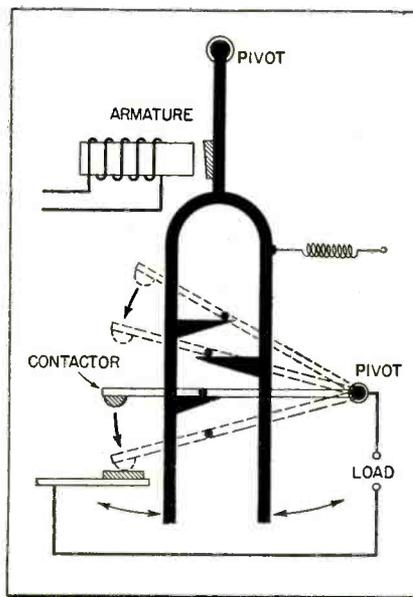
Fig. 4—Simplified version of a stepping relay. Not shown, is provision to return the contactor to its uppermost position.
