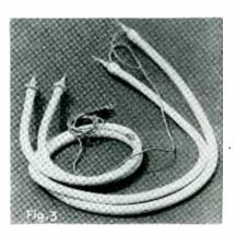
been proven by extensive usage, and for mechanical wearing qualities, the ordinary 7 mm. cable appears to be fully as satisfactory as most well made test leads. But in order to avoid eventual wire strand breakage due to excess handling of the test leads, an effort should be made to obtain 7 strand chromium steel 7 mm. ignition cable. It is virtually impossible to break any of these strands by ordinary flexing.
