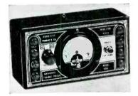
TROUBLE TRACER—Model 456 accurate inexpensive pocket size general utility instrument. Voltage ranges from 5 to 1000 volts; resistance from 5000 to 500,000 ohms; two current ranges of 0-1 and 0-10 ma.; decibels from minus 12 to plus 54. Radio City Products Co., 88 Park Place, New York, N. Y.
