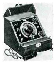
EXAM-ETER — New circuit and component analyzer. Serves as output indicator, dual range peak-voltmeter; r.f. alignment indicator; capacitance bridge; resistance bridge; power factor indicator; leakage indicator; and continuity checker. Solar Mfg. Co., Bayonne, N. J.
