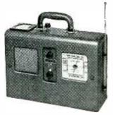
INTERFERENCE LOCATOR—Battery operated supersensitive receiver complete with loudspeaker, self-contained loop, fishpole antenna, output meter, and phone lack. Ideal for tracking down all types of man-made radio interference. Sprague Products Co., North Adams, Mass.
