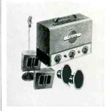
SOUND SYSTEM — Medium powered complete sound system, model C-418. Rated at 16 watts; 113 db. gain on mike input; 60 db. gain on two phono inputs; response 40 to 9500 cycles; output apped from 2 to 500 ohms. With two 10 inch p.m. speakers in wall baffles, mike, floor stand, all cables and plugs, \$99.98 list. Transformer Corp. of America, 69 Wooster St., New York, N. Y.
