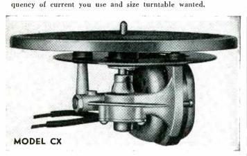
Model CX — Direct drive, self-starting induction-type motor. Fan-cooled. Fully enclosed, with silent helical-cut gears running in oil bath in sealed housing. Double-insulated drive sleeve. Delivered ready to install. Choice of 8", 9", 10", or 12" turntable.
