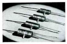
DUAL ELECTROLYTICS-Model BRL tubular units DUAL ELECTROLYTICS—Model BRL tubular units with common negative leads and polarity clearly marked. Supplied with sturdy mounting strap around its center which can be firmly attached to chassis by a single screw. Available in voltage ranges from 25 to 450 volts; capacity sizes from 5-5 mfd to 20-20 mfd. Cornell-Dubilier Electric Corp., South Plainfield, New Jersey.
