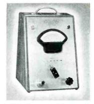
V. T. VOLTMETER—Model VG-6 full-wave square-law type infinite impedance vacuum tube voltmeter. Readings not affected by harmonics; frequency error is 3 per cent between 40 cycle and 56 mc.; furnished with coaxial test cable; voltage range from 2 to 600 volts in 6 steps; a.c. or d.c. scales selected by toggle switch. Televiso Co., 337-345 N. Crawford Ave., Chicago, III.
