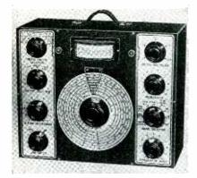
MICROVOLTER—Crystal controlled signal generator with self contained vacuum tube voltmeter and power level meter. Provides signals from 100 kc. to 15,000 kc. at 100 kc. points; also 1000 kc. to 100 mc. at 1000 kc. points. Accuracy better than 01 percent. R.f. output from ½ to 100,000 microvolts. Seven radio frequency ranges calibrated directly from 100 kc. to 60 mc. Hickok Electrical Instrument Co., 10514 Dupont Ave., Cleveland, Ohio.
