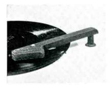
CRYSTAL PICKUP—Model X-79A phono pickup with convenient single mounting hole fastener; may be used on motorboards 1/16 to ½ inch thick. Frequency response stated to be 50 to 8500 cycles; 2.5 ounce needle pressure. Arm assembly is rubber cushioned eliminating microphonic feedback and motor noises. Available with or without built-in pilot light. Webster Electric Co., Racine, Wisconsin.
