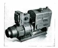
POWER PLANT—A 5 k.w. gas electric power plant designed for heavy duty. Engine completely enclosed in sheet metal housing to protect it from dirt, dust and rain. Uses 4 pole generator rotating at 1800 r.p.m. Complete with rheostat, voltmeter and switchbox. Filter and shielding available for radio operation. Pioneer Gen-E-Motor Corp., 466 W. Superior St., Chicago, III.
