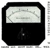
Bakelite case measures 31/2" square, mounts through 2 5/16" panel hole. Long arc scale with knife edge pointer. Rugged movement of 2% accuracy—sensitivity 50 MV in the 0/1 MA range.
