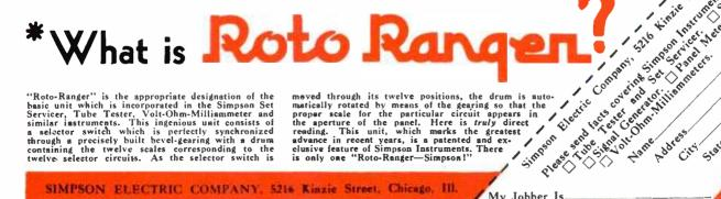
"Roto-Ranger" is the appropriate designation of the basic unit which is incorporated in the Simpson Set Servicer, Tube Tester, Volt-Ohm-Milliammeter and similar instruments. This ingenious unit consists of a selector switch which is perfectly synchronized through a precisely built bevel-gearing with a drum containing the twelve scales corresponding to the twelve selector circuits. As the selector switch is
