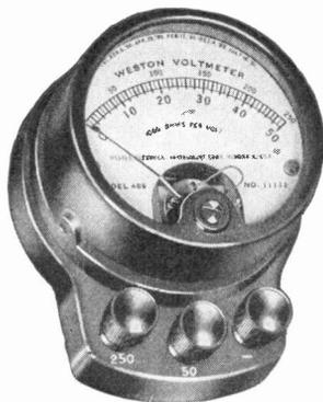
**D. C. Model 489 Battery Eliminator Voltmeter** — with self-contained resistance of 1000 ohms per volt—for testing the output of B-Eliminators. Also furnished with lower resistance for general D. C. testing requirements. Very popular models, and they are moderately priced.
