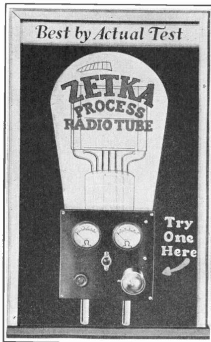
The above counter display stands 22 inches high and contains a tube tester made up of Weston instruments mounted on a small bakelite panel. A rheostat located in one corner controls the filament voltage, and the push button in the center operates a safety circuit, so that in case the tube elements are short-circuited no damage will be done to the meters.
