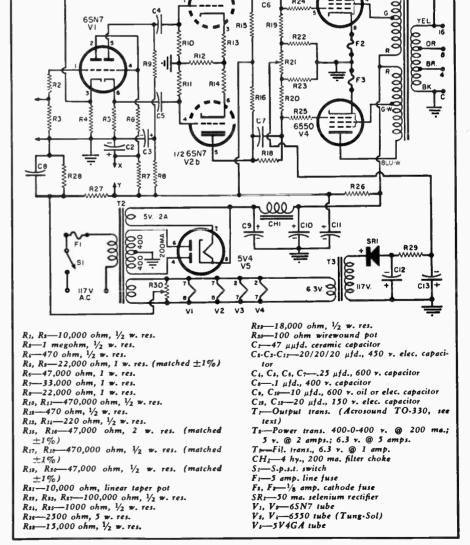
procedure local feedback may be added to stages within the amplifier in order to reduce their contribution to the phase shift. Thirdly, the bandwidth of the stages may be extended by the use of certain design techniques, and the phase shift correspondingly reduced.
