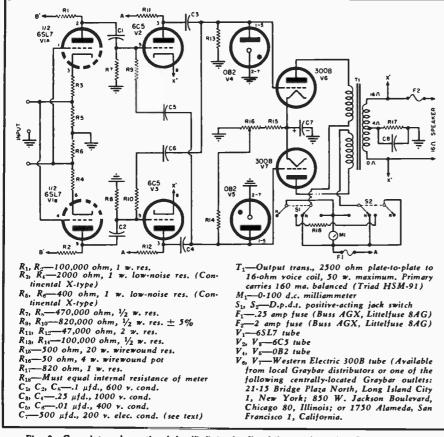
Fig. 3. Complete schematic of the "infinite feedback" amplifier. See Fig. 5 as well.
