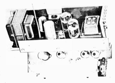
Rear and bottom views of the S-1000 amplifier chassis. Dimensions are 14" x  $10\frac{1}{2}$ " x 4".
