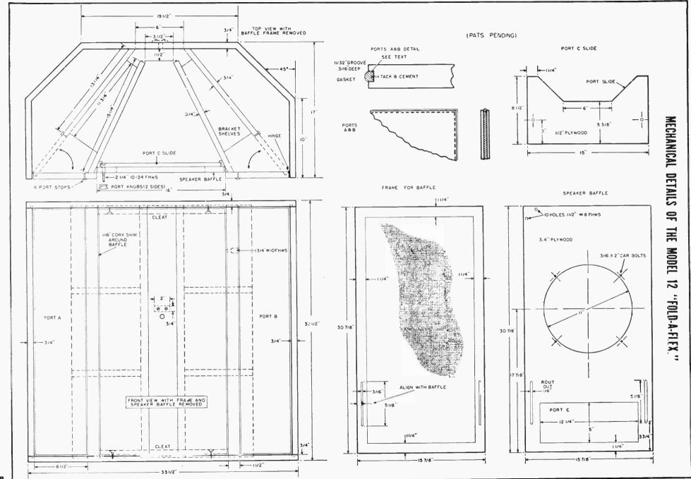
there a cabinet that has all three baffle characteristics built in? There is one all-purpose loudspeaker enclosure. It is called the "Fold-a-flex" because it can be used as a folded horn, an infinite baffle, or as a bass reflex.
