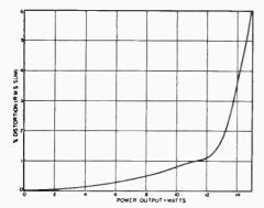
Fig. 3. Intermodulation distortion of the amplifier, 60 and 7000 cps. 4 to 1 ratio.
