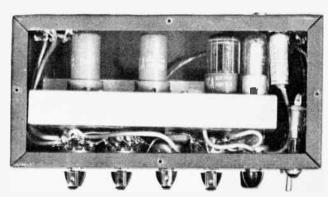
THE preamplifier in a modern high-fidelity installation is called upon to perform several very important tasks. It is required to supply the amplifying system with most of its voltage gain. It is required to supply the proper gain vs frequency characteristics of the program material, and it must act as the control center for the entire high-fidelity system.
