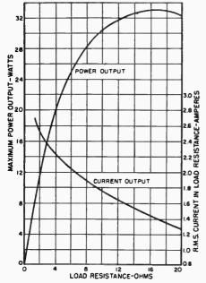
Fig. 9. The calculated maximum power and current delivered by the amplifier into various load resistances. Refer to text.
