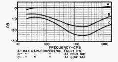
controls are set for flat response or some degree of boost-seldom for cut. The "Compentrol" offers a combined bass and treble boost in itself and, with the judicious use of the level set. a flexible tonal range is obtained. Despite the controversy, the reader is urged to try the unit himself and make up his own mind.
