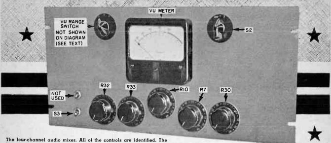
The four-channel audio mixer. All of the controls are identified. The "not-used" toggle switch was incorporated to provide an extra switch should it be required. It could serve as a power supply "on-off" control, if desired.
