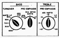
Fig. 5. Sample control panel for the constant-amplitude equalizer unit.
