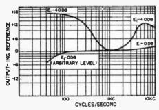
Fig. 3. Measured curves of the "Auto-Tone."
