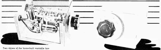
Two views of the home-built variable lowpass filter. It is housed in a 3"x4"x 5" aluminum utility box which is small enough to be tucked in almost anywhere.
