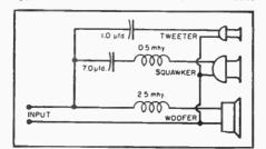
having a 6 db/octave slope instead of the type having a sharp cut-off. When using separate, 3-way drive systems in this enclosure it is possible to achieve the same response and freedom from distortion above 1000 cycles as are available in the "Klipschorn" in the same frequency range. This means that the reduction in size and cost has resulted in a sacrifice in tonal response only in the region below 1000 cps.
