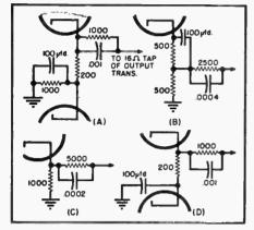
Fig. 3. Various feedback arrangements from voice coil of the output to the cathode of an early stage. See text for discussion.
