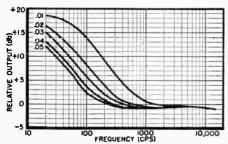
Fig. 1. Hesponse of booster with different condenser values from .01 to .05  $\mu$ fd. The zero level is .775 volt in this instance.
