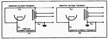
Fig. 1. The use of current feedback for damping factor control. Refer to article.
