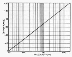
Fig. 3. Relation between constant-velocity and constant-amplitude characteristics. If a variable-frequency disc were recorded at constant amplitude and played back with a velocity-sensitive pickup, the response would follow the curve indicated above.
