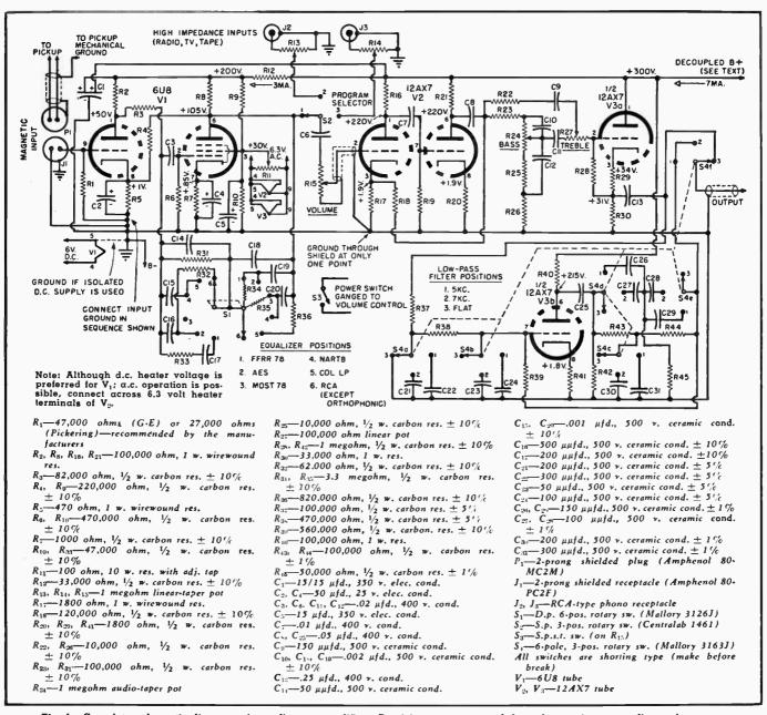
Fig. 1. Complete schematic diagram of equalizer-preamplifier. Precision parts are used throughout to insure quality performance.
