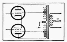
Fig. 2. Basic "Ultra-Linear" arrangement.
