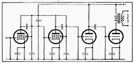
It acts as a negative resistance. This often occurs if the plate voltage falls considerably below the screen voltage. Changing the value of the screen dropping resistor is usually the cure for this kind of oscillation, so that the tube resumes stable operating conditions. Too high a plate load resistor, in relation to the screen dropping resistor, can cause oscillation.
