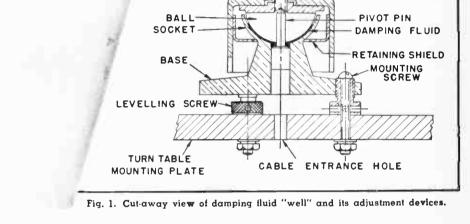
The use of a special silicone regulates both vertical and horizontal movement and prevents disc damage from dropping.
