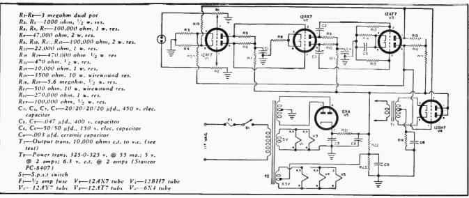
Fig. 2. Schematic of cathode-follower amplifier. An inexpensive output transformer and single dual-triode output tube are used.
