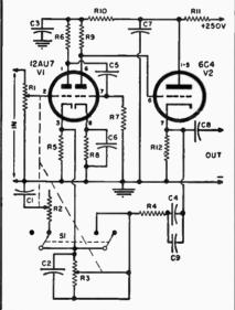
$R_1*=500,000$  ohm linear-taper pot  $R_2*=3000$  ohm linear-taper pot  $R_3*=250,000$  ohm audio-taper pot  $R_3*=250,000$  ohm, 1/2 w. res.  $R_1=3300$  ohm, 1/2 w. wirewound res.  $R_1=1000$  ohm, 1/2 w. wirewound res.  $R_1=470,000$  ohm, 1/2 w. res.  $R_1=470,000$  ohm, 1/2 w. res.  $R_1=1000$  ohm, 1/2 w. res. 1/2 w. res.  $R_1=10000$  ohm, 1/2 w. res.  $R_1=10000$  ohm, 1/2 w. res. res. 1/2 w. res. res. 1/2 w. res. 1/2 w. res. 1/2 w. res. 1/2 w. res. res. 1/2 w. res. 1/2
