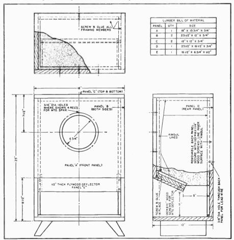
well glued and screwed. Internal damping is provided by "Kimsul" insulation.
