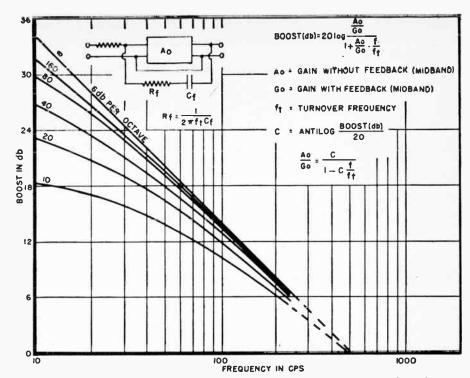
Fig. 2. Rate of bass boost of feedback equalizers depends largely upon the ratio of midband gain with and without feedback. Text points out shortcomings of many equalizers using degeneration and offers basis for development of unique circuit.
