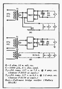
Fig. 4. Two easily-built d.c. heater supplies designed to be used with the first stages of the high-gain preamplifier unit.
