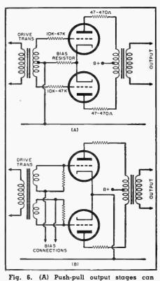
sometimes go into high-frequency oscillation. Grid and plate blocking resistors, connected close to the tube pins, will stop this. In pentode or tetrode stages, such blocking resistors may also be required. (B) Alternative connections necessary for output stages running into AB<sub>2</sub> or B<sub>2</sub>, to avoid stage loading by the grid current.
