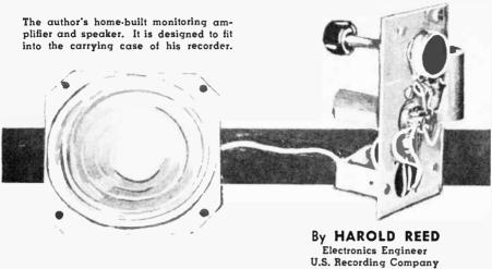
Details on a compact, 1-tube amplifier that is small enough to be tucked into the recorder's carrying case.
