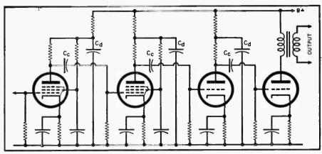
Fig. 2. This kind of high-gain audio circuit can cause motorboating troubles. Attention to the values of  $C_{\rm c}$  and  $C_{\rm d}$  can sometimes cure this particular circuit fault.
