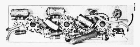
The amplifier section was constructed on an "L"-shaped aluminum bracket with shield.
