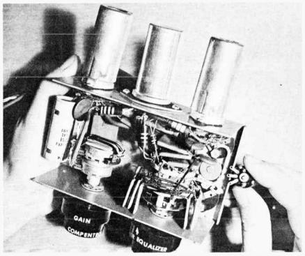
of the second stage  $V_{1B}$ . In the original the outputs are separated into positions for the standard (78 rpm) records and for the LP's (both 33 and 45 rpm). The output for the 78's is divided down for the lower output voltage while that for LP is not. Component-wise the circuit follows the Scott circuit but the feedback net-
