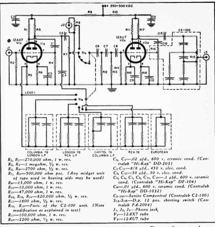
Fig. 4. Complete schematic of the printed circuit preamp. The equalizer networks, shown dotted at lower left, are not commercially available but suitable networks can be substituted by following the diagrams and parts values shown in Fig. 2.
