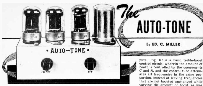
Front panel view of the "Auto-Tone." Three 7F7's are used although almost any twin-triode can be substituted if desired.
