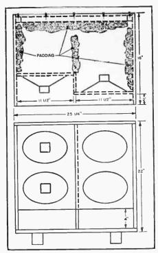
Dimensions of 3½ cubic foot enclosure for push-pull speaker system. All panels should be of ¾" plywood. All joints should be glued and nailed, except back which is screwed on. Sides are lined with acoustically absorbent material as shown above.
