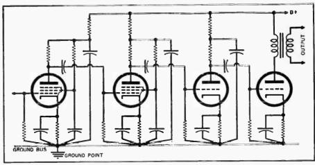
Fig. 5. Poor ground return wiring can cause either type of instability. This schematic shows the method of making returns, using the circuit of Fig. 2, to avoid the ground return as a possible cause of instability in the audio amplifier.
