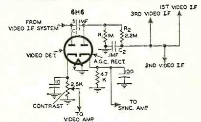
Fig. 3. The a.g.c. network in Farnsworth television receivers (the Model GV-260)
