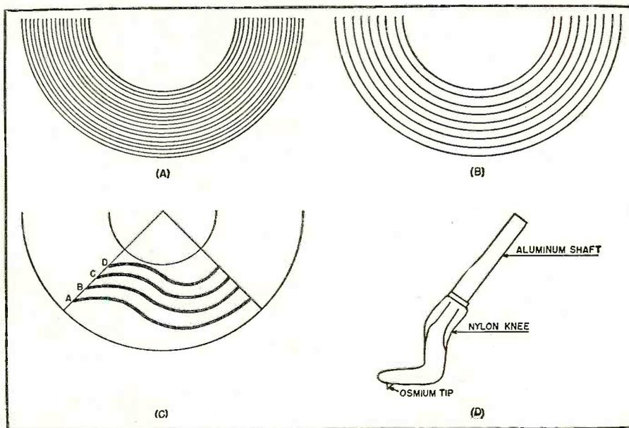
Fig. 2. (A and B) Comparison of the number of grooves cut on a (A) Microgroove and (B) standard recording. (C) An exaggerated example of the "pinch effect." (D) The Webster-Chicago nylon "knee-action" needle designed to be used with Microgroove records.
