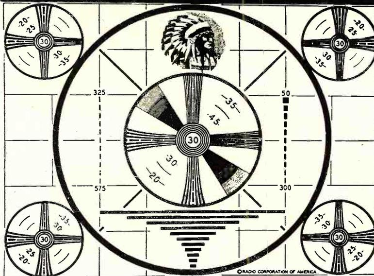
Fig. 1. "Indian Head" test pattern used by many television stations.
