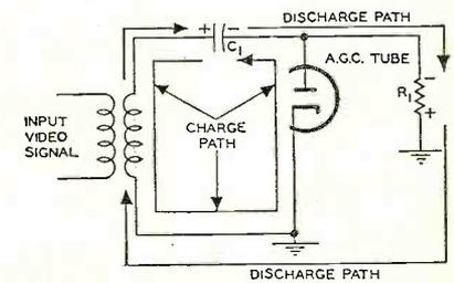
Fig. 4. The equivalent a.g.c. network of Fig. 3, and its mode of operation.
