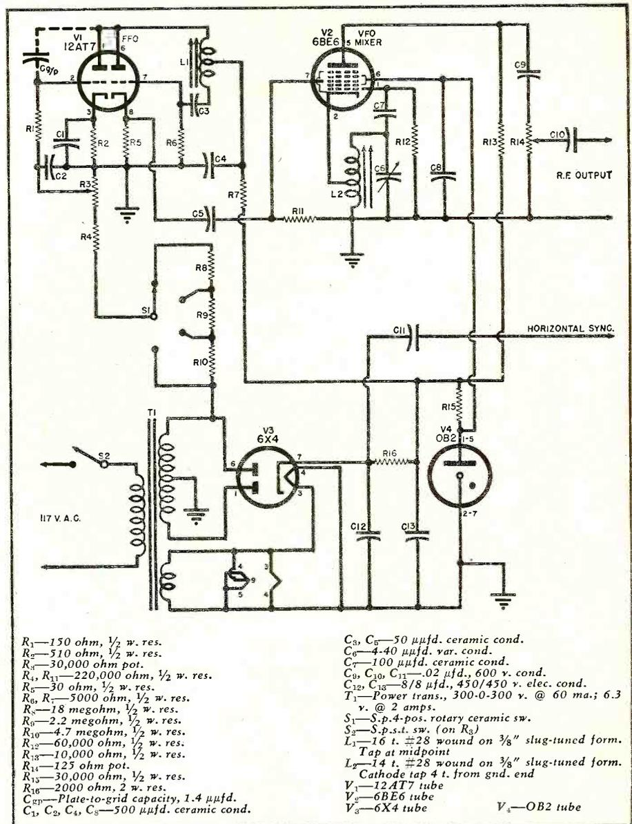
Fig. 1. Complete circuit diagram and parts list of the stable FM sweep generator.
