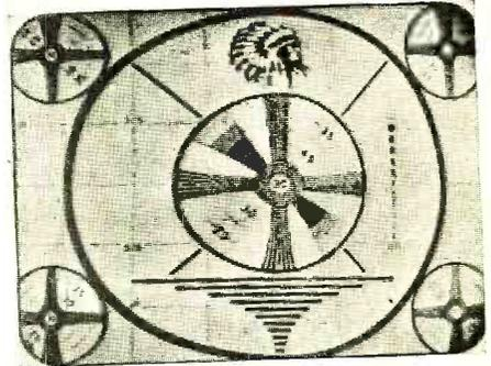
Fig. 3. Example of horizontal non-linearity.
