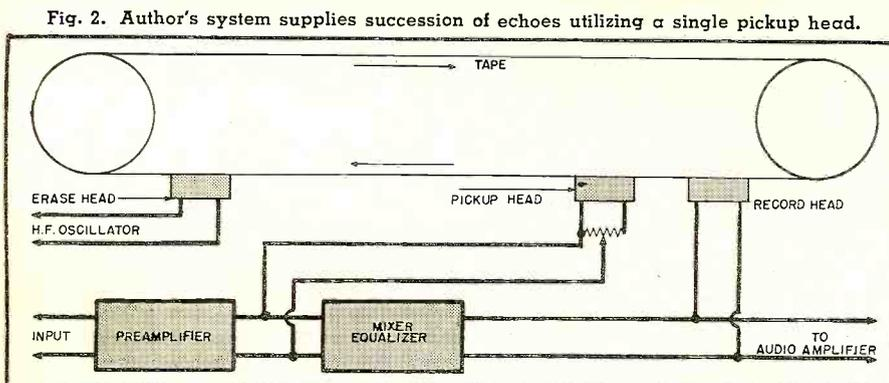
Fig. 2. Author's system supplies succession of echoes utilizing a single pickup head.
