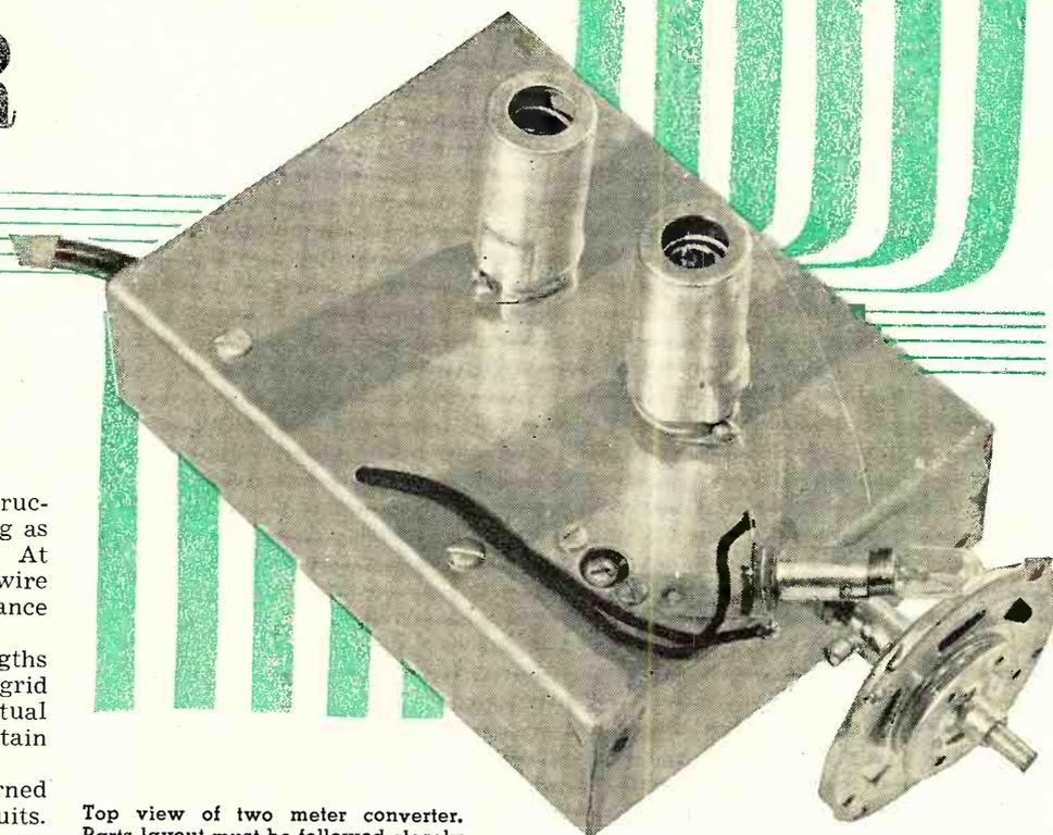
Top view of two meter converter. Parts layout must be followed closely in order to insure correct operation.
