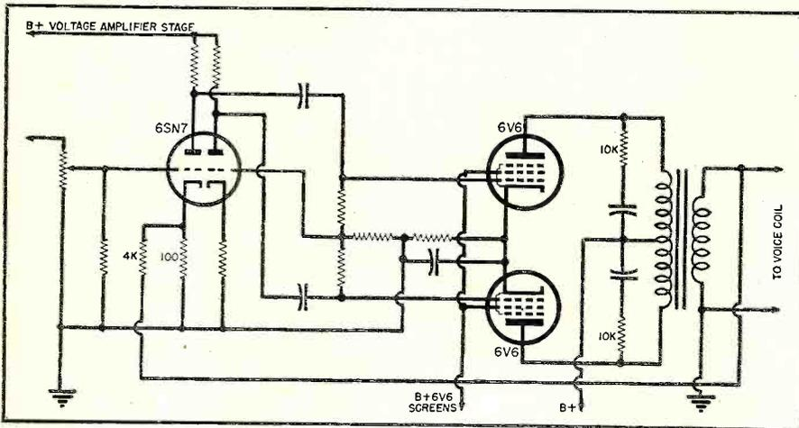
Fig. 4. Audio system of first set showing the four added resistors which were inserted in the circuit to improve the response and performance.
