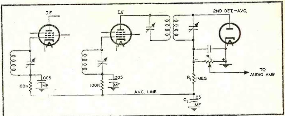
Fig. 1. A typical a.v.c. network found in standard broadcast AM receivers.
