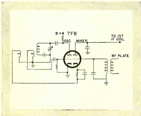
**TRIODE MIXING . . .** in the first detector. This quieter method of conversion greatly boosts the signal-to-noise ratio because there's almost no first detector "hiss." Inductive coupling (rather than electronic) of the oscillator signal avoids multi-grid noise in the sensitive 50-Mc range.
