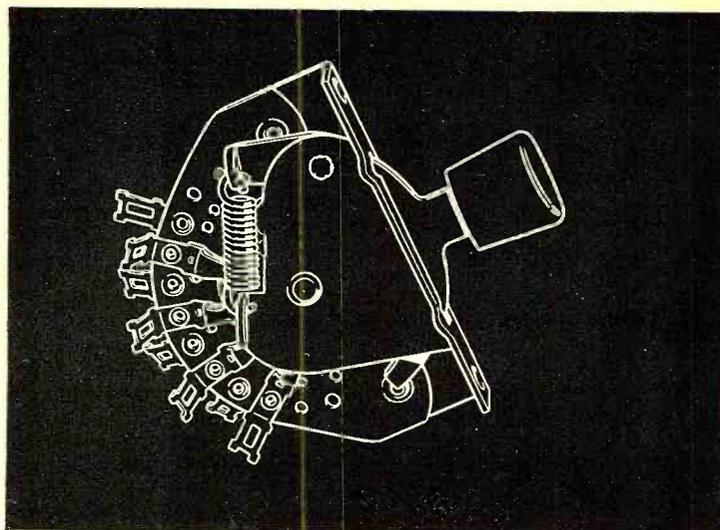
**Controls:** With CRL's improved *Adashaft* Radiohms you can carry a small stock of controls, yet be ready to handle almost any kind of control replacement problem. No wiggle, no wobble, no slip. Just insert shaft pilot in control stub shaft, and slip "C" washer into place. Available in all sizes for all model "M" volume control applications. Six types of shafts.
