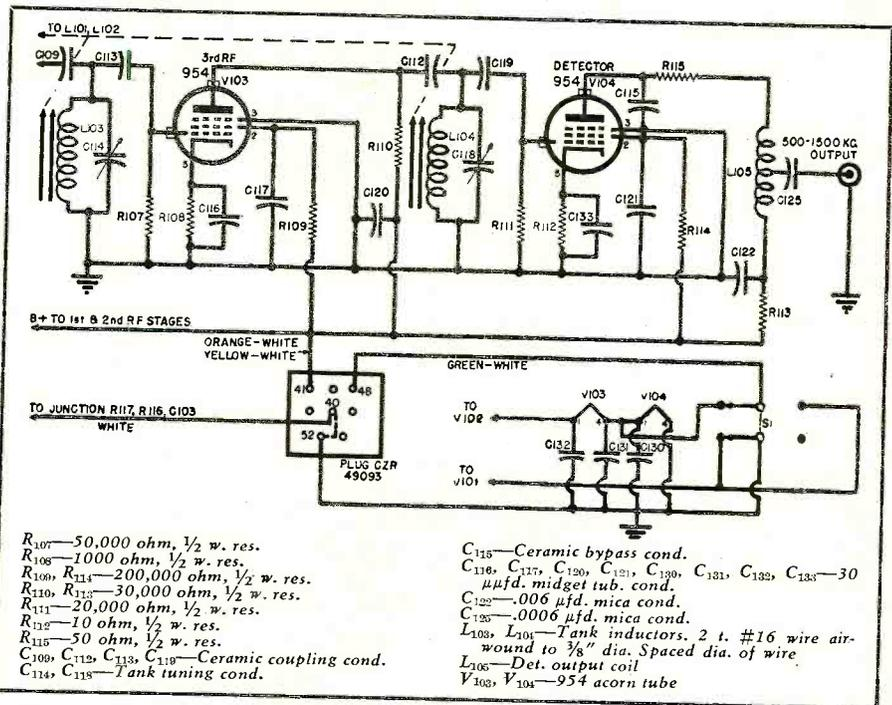
Fig. 1. Original diagram and parts list for the last 2 stages of the surplus ARR-1 unit.
