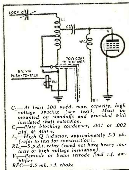
Fig. 2. Coupling network and tank circuit for use with single-turn loop of Fig. 3.
