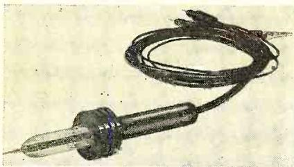
age Safety Test Probes, the new units afford direct measurement facilities up to 30,000 volts d.c. with complete safety to the operator.
