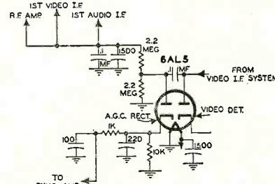
Fig. 5. The a.g.c. system used by Belmont. It is similar to the Farnsworth system.
