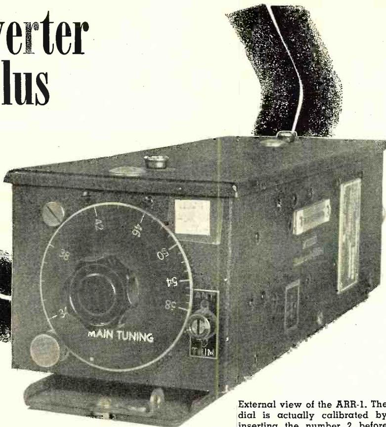
External view of the ARR-1. The dial is actually calibrated by inserting the number 2 before each of the dial markings. Thus, 38 becomes 238, the frequency to which the unit is tuned. Since the photo was taken the amateur assignment has been lowered to 220-225 mc. instead of 235-240 mc. A simple alteration of the tuning coils effects this lowering of frequency.
