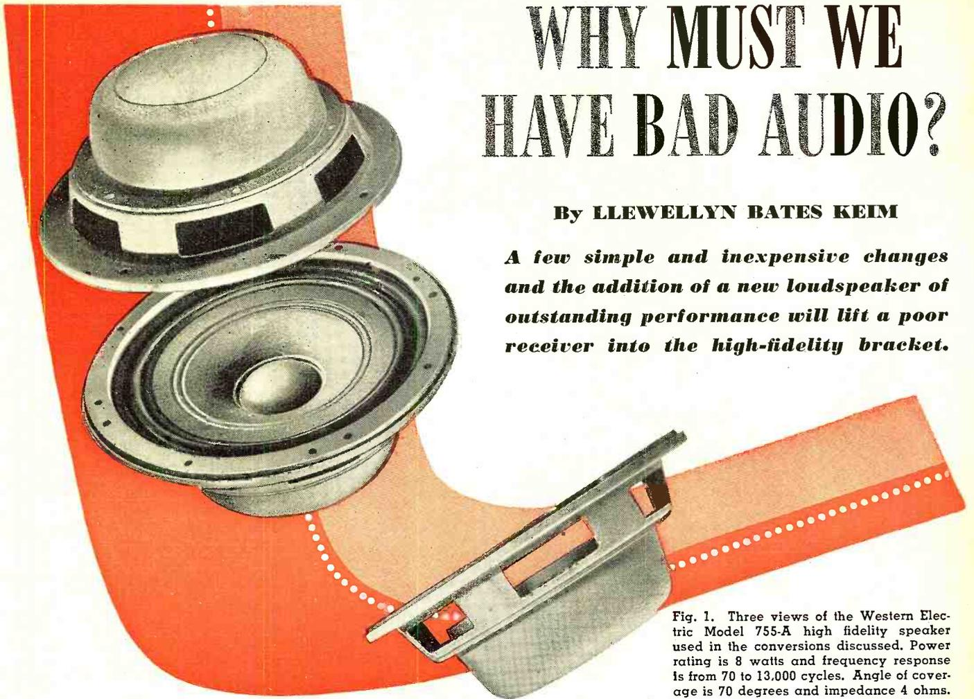
Fig. 1. Three views of the Western Electric Model 755-A high fidelity speaker used in the conversions discussed. Power rating is 8 watts and frequency response is from 70 to 13,000 cycles. Angle of coverage is 70 degrees and impedance 4 ohms. The unit should be housed in a 2 cu. ft. baffle totally enclosed except for 7" baffle hole. Inside dimensions of baffle should be 19" wide, 22" high, 8 7/8" top depth, and 11 13/16" bottom depth. Lining should be 1" sound absorbing glass wool.
