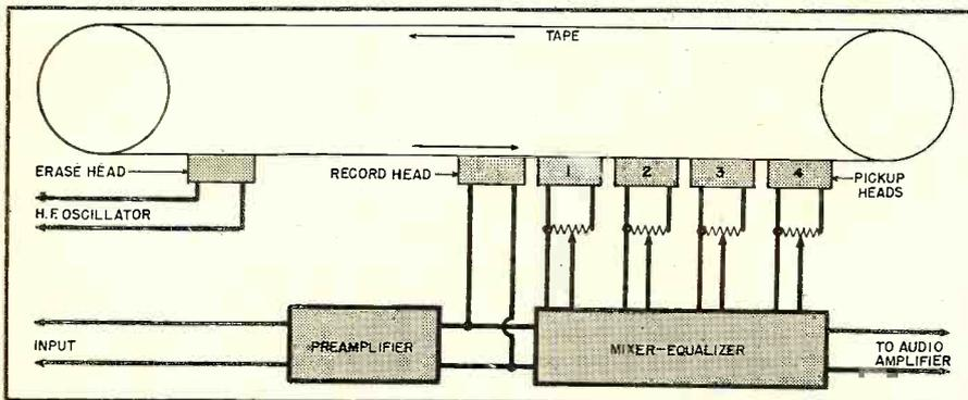
Fig. 1. Diagram shows conventional system (not described in text) whereby four individual pickup heads are used to supply reverberation effect.
