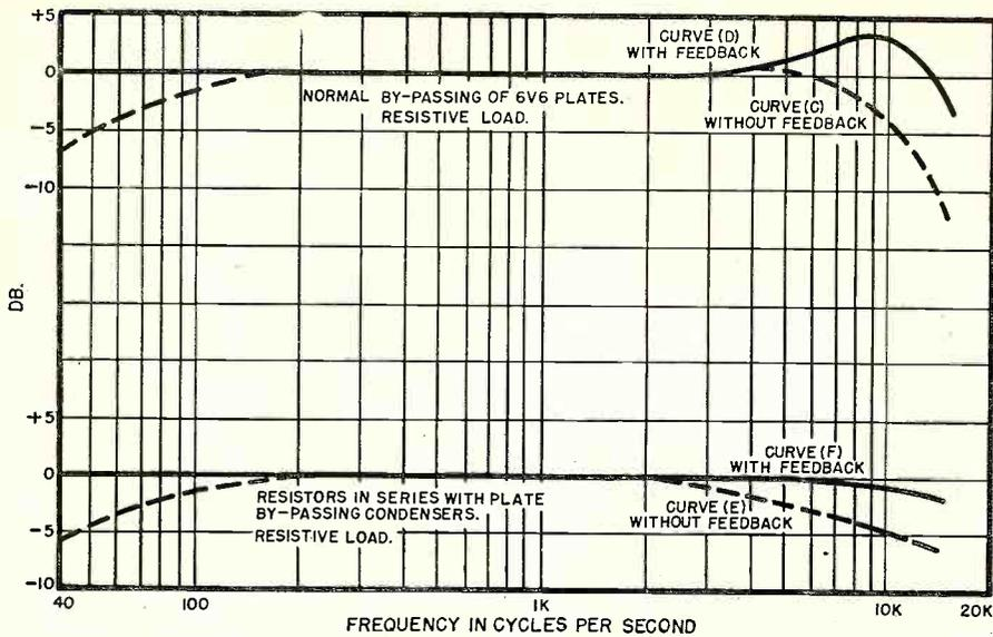
Fig. 3. Curve shows improvement in the set's response after circuit alterations were made. Curves were taken with the volume control full-on.
