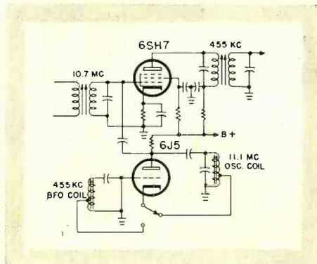
**DOUBLE SUPERHET . . .** After two stages of IF at 10.7 Mc, this 6SH7 makes a second conversion down to 455 kc for ample selectivity, plus complete absence of images. The 6J5, which is used as BFO on other bands and otherwise idle on this band, acts as local oscillator. No extra tubes, yet plenty of extra performance!
