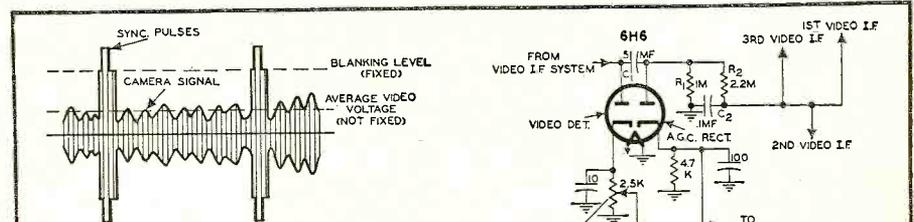
Fig. 2. Only the blanking and the sync pulse level of a television signal are indicative of the true carrier level.
