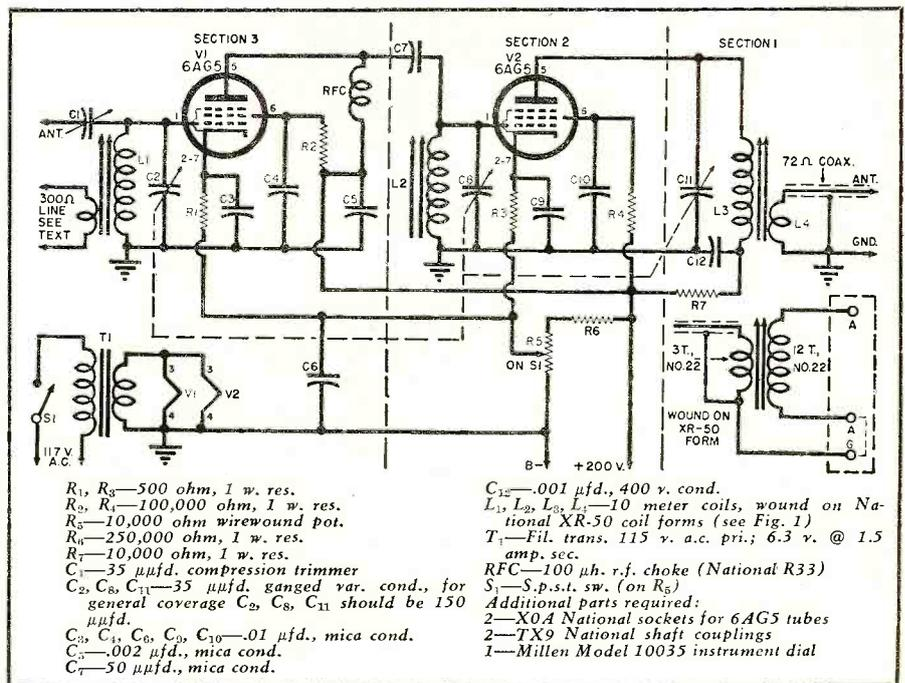
Fig. 2. Circuit diagram of the two-tube preamplifier. The circuit shown at the lower right may be used to match preamplifier to the normal 400 ohm receiver input.
