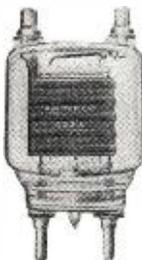
TYPE 833 A: An exceedingly compact glass triode widely adopted for many functions in both the communications and industrial services. As a generator of frequencies up to 30 mc it will give 1000 watts output without forced air cooling and as much as 1600 watts with a small blower.
