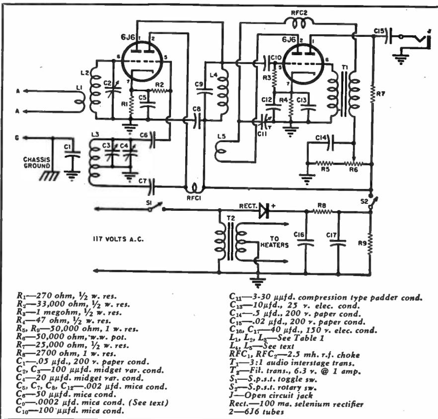
Fig. 3. Complete circuit diagram and parts list for simple two tube "ham-super."
