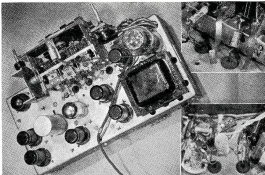
Fig. 6. Top view of the converted General Electric JFM-90 FM tuner. Insets show position of series condensers that are placed in the variable condenser leads and the under chassis position of the new oscillator coil.
