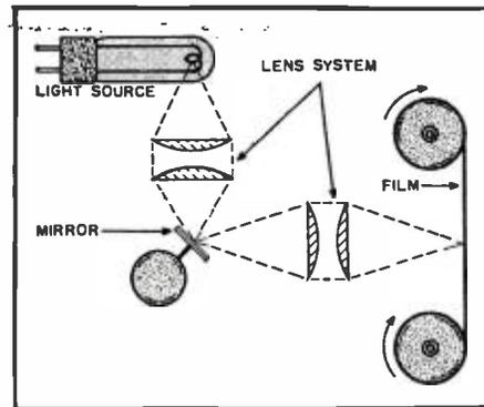
Fig. 7. The essential elements used for variable area optical recording.
