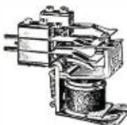
**A-100 Antenna Relay** A low loss AISiMag insulated relay. For single wire fed installations specify the A-100-C, SPDT unit. Two A-100-C in place of one A-100 in open wire line systems will avoid possible impedance mismatch. A very popular relay with radio amateurs.
