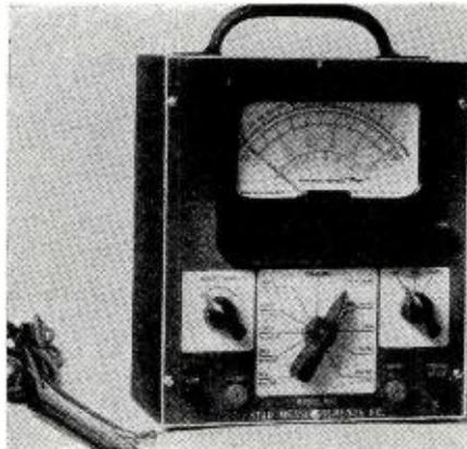
voltage ranges up to 1000 volts, both a.c. and d.c. Current ranges up to one ampere and resistance ranges up to five megohms are also included. Calibrated db. scales provide for measurements as high as 54 db.; the zero power level is based on a 6 mw. level in a 500 ohm line. In all, 27 separate ranges of measurement are provided.
