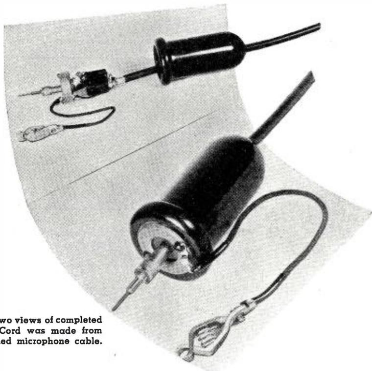
Fig. 1. Two views of completed probe. Cord was made from a shielded microphone cable.
