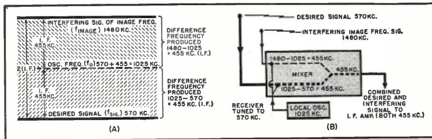
Fig. 2. (A) Should a superheterodyne receiver with an i.f. frequency of 455 kc. be tuned to 570 kc., a 1480 kc. image frequency interference will result. (B) How a desired and an image response signal can combine with the local oscillator output to produce two signals, both having a frequency equal to the i.f.
