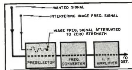
Fig. 3. Illustrating how an image frequency signal may be sufficiently attenuated by a preselector so that it does not reach the frequency converter.
