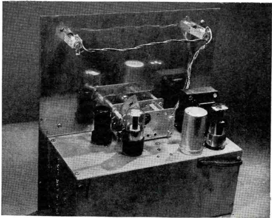
Fig. 3. Rear view of signal generator. Under chassis components of this r.f. section are completely shielded to prevent radiation to external circuits.
