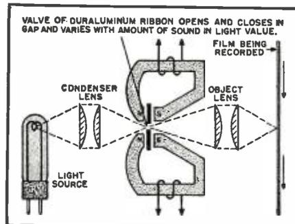
Fig. 5. The essential elements employed in variable density recording.
