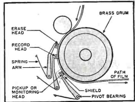
Fig. 9. Triple head assembly for recording and reproducing (magnetically) on film.
