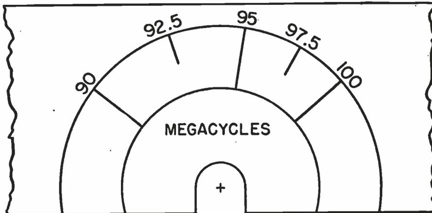
Full scale drawing of recalibrated dial scale for GE tuner.
