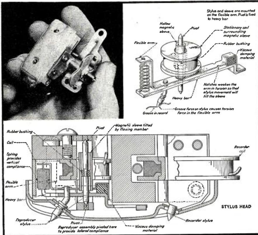
Fig. 3. Audograph record-playback head for embossing sound on Vinylite records.
