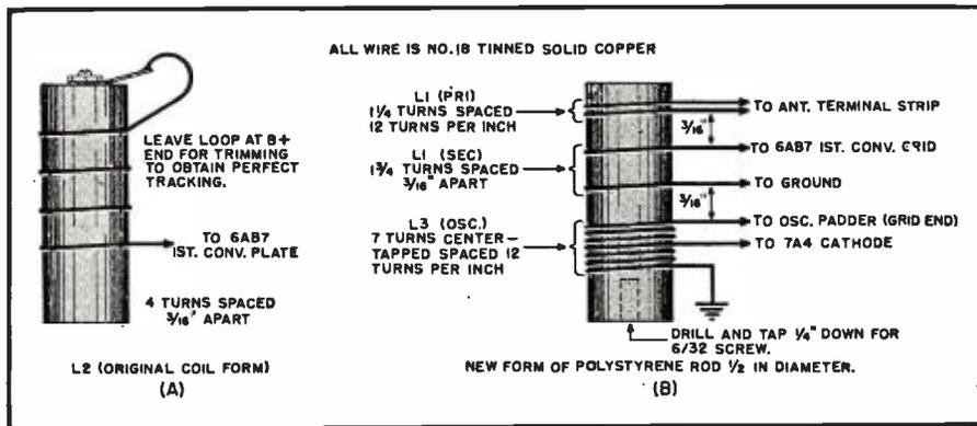
Fig. 9. Mechanical details of coil assembly for the General Electric JFM-90 tuner.
