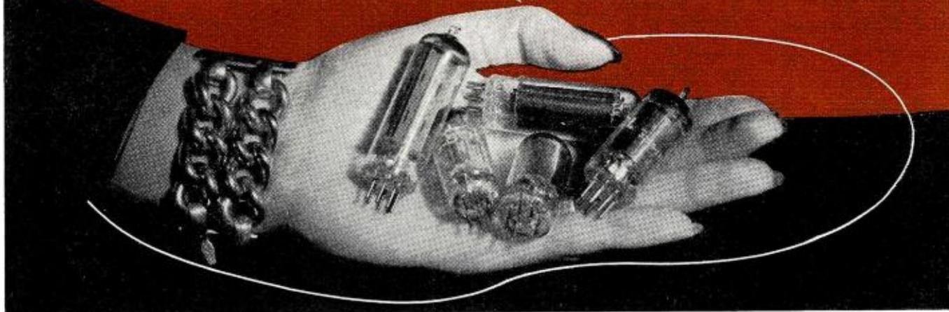
As soon as production permits, these new miniature tubes will be used in 5-tube, table model, a.c.-d.c. receivers. This new tube kit will consist of 35W4, 50B5, 12BA6, 12BE6 and 12AT6. They will replace the 35Z5, 50L6, 12SK7, 12SA7 and 12SQ7 respectively.
