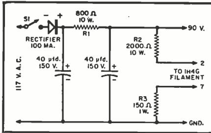
Fig. 2. Schematic diagram of power supply to be used with photocell unit. The power supply covered in last month's issue, page 67, can be easily adapted for this purpose.
