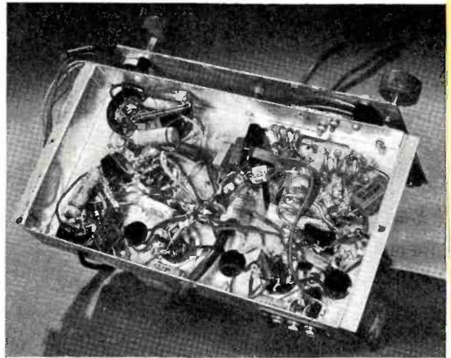
Fig. 4. Converted Meissner tuner showing coil placement.
