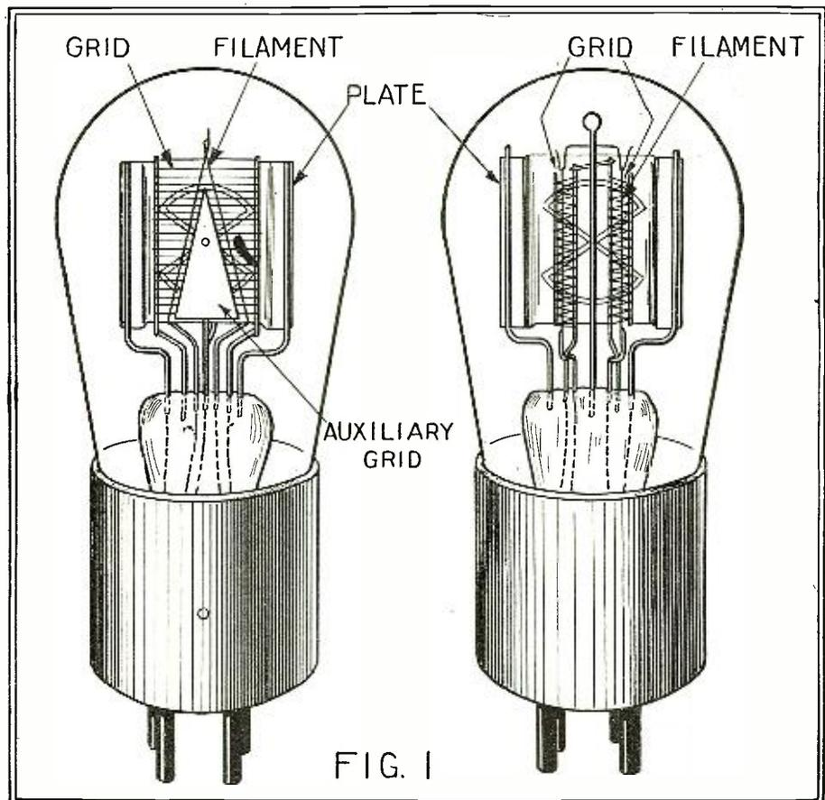
Constructional details of the two vacuum tubes described in this article. The auxiliary grid shown in the left-hand tube functions as a control element. A number of circuits particularly adaptable to this tube are shown above.
