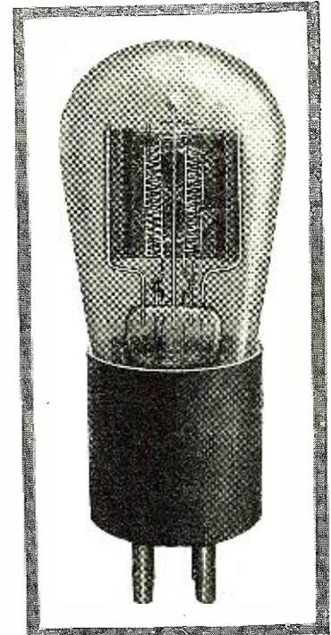
A tube so designed that it has a very low inter-element capacity. Note the slender low-section grid.
