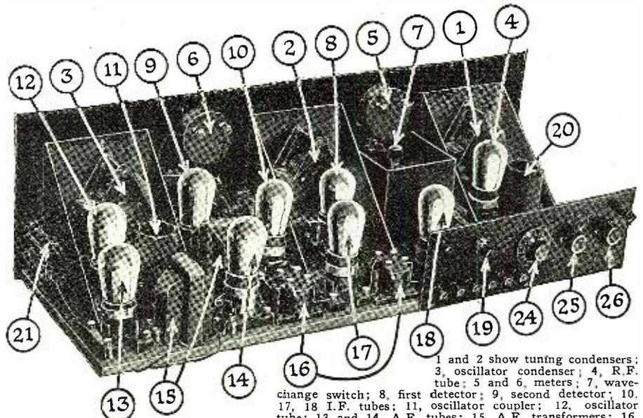
1 and 2 show tuning condensers; 3, oscillator condenser; 4, R.F. tube; 5 and 6, meters; 7, wave-change switch; 8, first detector; 9, second detector; 10, 17, 18, I.F. tubes; 11, oscillator coupler; 12, oscillator tube; 13 and 14, A.F. tubes; 15, A.F. transformers; 16, long-wave transformers; 19, jack switch; 20, antenna inductance; 21, phone jack; 24, potentiometer; 25 and 26, rheostats. Parts shielded by copper cans when in use are seen here.
