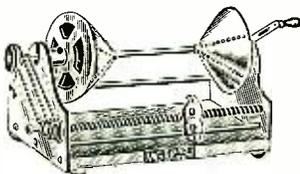
ORATORIES for test. This machine is a very handy addition to the radio workshop. Tubing of any size may be wound with any size wire.
