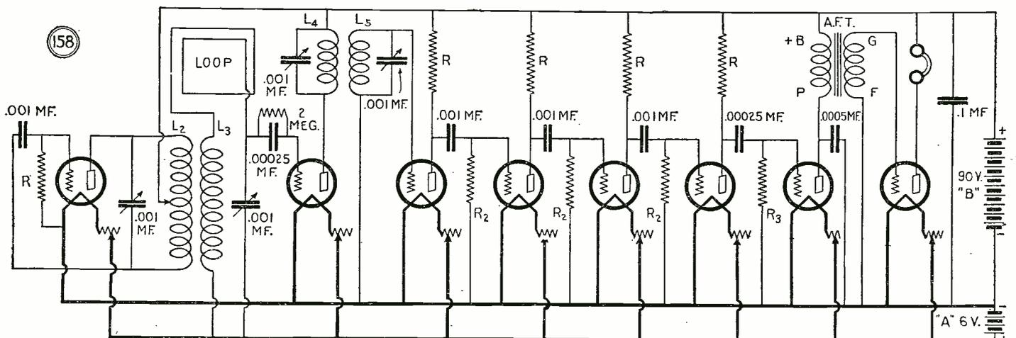
(158) An exceptionally efficient and "quiet" Super-Heterodyne receiver, capable of producing unusual results with pure tonal quality due to the most efficient type of amplification known (as regards its capabilities of distortionless reproduction) that of the resistance-coupled type. The circuit is a very flexible one and may be made to operate at various intermediate frequencies, by simply changing the oscillator and filter-coil design.
