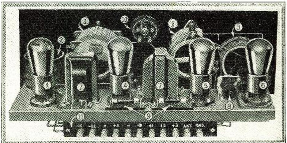
The rear view of the receiver: 1, the variable condensers; 2, the R.F. transformer; 3, the antenna coupler; 4, A.F. amplifier tubes; 5, detector tube; 6, R.F. tube; 7, A.F. transformers; 8, compensating condenser; 9, automatic filament controls; 10, high-resistance rheostat; 11, terminal board.
