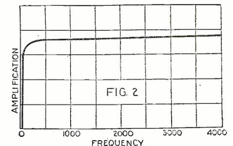
With a resistance-coupled amplifier the amplification curve is flat over a wider range of frequencies than that of a transformer-coupled amplifier.
