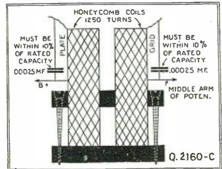
The design of the filter or in-pu transformer. Although these coils may be wound similarly to ordinary transformers, ordinary honeycomb coils may be used with the same efficiency.
