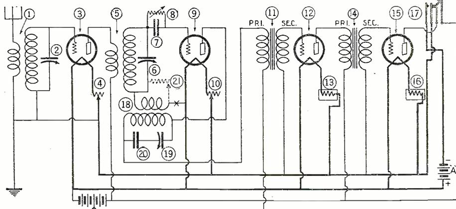
Fig. 1. The schematic circuit diagram of this novel, experimental tuned radio frequency receiver is shown above. Using standard units for tuning, this circuit gives exceptional results when it is properly balanced. The same numbers assigned to the various instruments in the diagram above are also placed on the illustrations on this and the next two pages.
