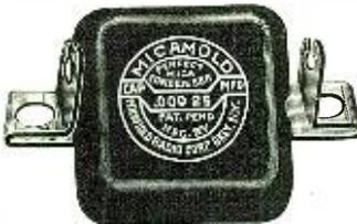
It is designed for use in the detector circuit in any receiver. The condenser plates are entirely enclosed by some moulded material, which makes the condenser moisture-proof and therefore constant in capacity.
