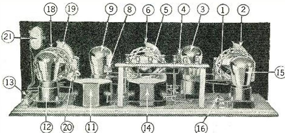
Fig. 4. 20 indicates the .00025- $\mu$ f. fixed condenser, which is connected in series with the tuning condenser of one of the tuned radio frequency units, in order to reduce the effective capacity of the circuit; 21 is the 100- to 1,000-ohm variable resistance, used for controlling oscillation in the circuit of the detector tube.
