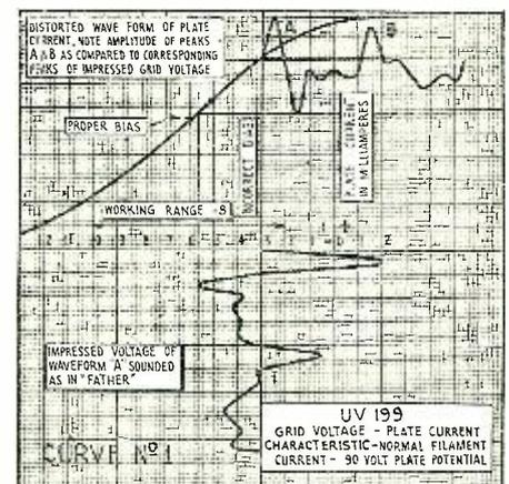
An ordinary static curve of the UV-199 tube, showing how an incorrect grid bias can cause severe distortion on strong signals. Note that the proper bias of  $-6$  is higher than is commonly used with the UV-199. Since the working range is only 8 volts, larger grid fluctuations than this will overload the tube. Compare this curve to curve No. 2.
