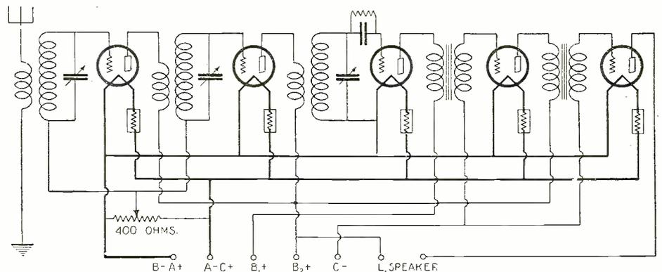
The circuit diagram of the Doughnut Five is shown above. The only adjustment, beside that of the three tuning condensers, is the potentiometer, for regulating the grid bias on the R. F. tubes.
