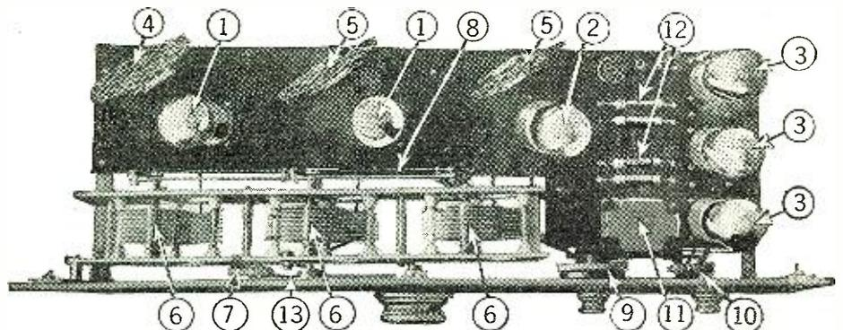
Top and rear views of the set described on this page: 1, R. F. Amplifiers; 2, Detector; 3, A. F. Amplifiers; 4, Antenna Coupler; 5, Interstage R. F. Transformers; 6, Tuning Condensers; 7, Dial Light; 8, Single-Control Mechanism; 9, Filament Rheostat; 10, Filament Switch and Volume Control; 11, Audio Frequency Transformer; 12, Resistance-Coupling Units for A. F. Amplifier; 13, Celluloid Dial. Photos by courtesy Pfanstiehl Radio Co.
