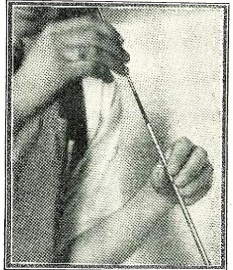
By using a piece of copper tubing, shown in the operator's left hand, spaghetti may be easily pushed over bus bar wire.
