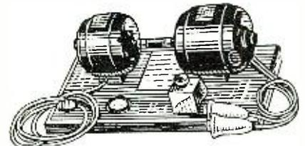
Fig. 9. Motor generator chargers are efficient and are often desirable. Here is a small, compact type.
