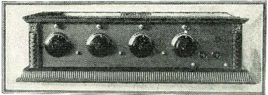
This cabinet is distinctive in design, but the circuit and instruments within are even more unusual. Notice the separate panel light above each dial. The four controls run in absolute synchronism, and do away with the necessity of single control.
