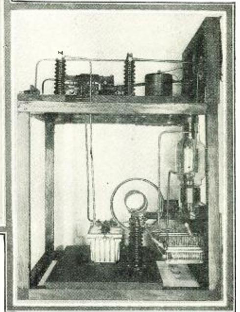
At the left are shown the panel and interior views of the receiver, which is of the Snell type, used at station FX1. The various inductance coils, which are shown on each side of the set, fit in the sockets provided for them in the upper left side of the receiver's baseboard.
