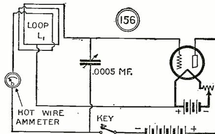
(156) An extremely efficient and simple portable transmitter capable of signaling within the distance of 15 miles, using a loop in place of the conventional antenna.
