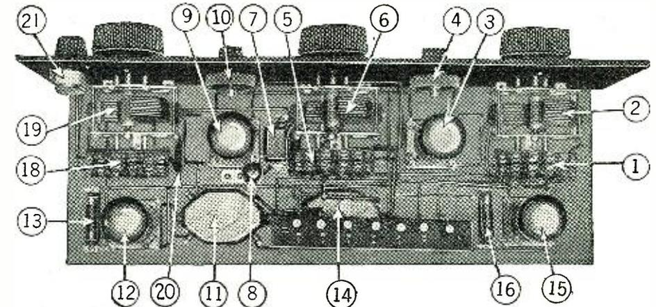
Fig. 3. 7 indicates the grid condenser, of .00025- $\mu$ f. capacity; 8 is a standard type of variable grid leak; 12 is the first audio frequency amplifier tube; 13 is the amperite controlling the filament of tube 12; 14 is the second audio frequency amplifying transformer; 15 is the second audio frequency amplifier tube; and 16 is its filament control resistance.
