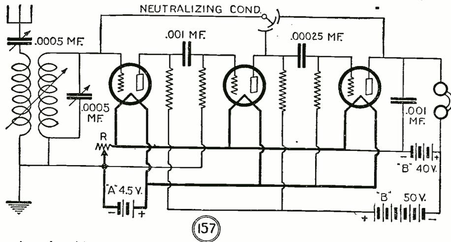
(157) A novel receiving system in which resistance-coupled amplification and a neutralized stage of tuned radio frequency amplification are used, resulting in clear, undistorted signals that are very pleasing to the ear.
