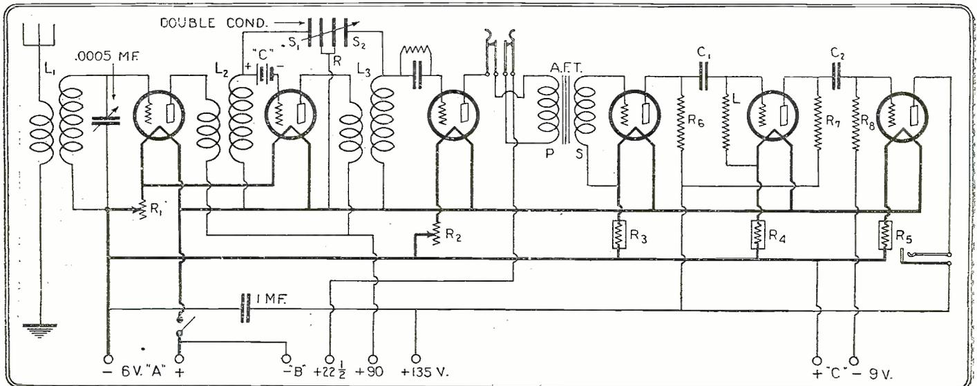
Above is shown the circuit diagram of this six-tube radio frequency receiver. The different values for the parts are given in the accompanying text.
