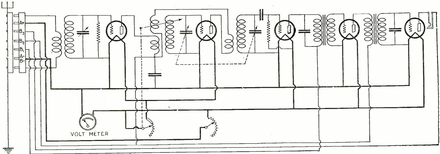
At the left of this diagram may be seen a conventionalized drawing of the round connection plug shown in the foreground of the half-tone at the bottom of the page. Observe that the filament voltage of the radio frequency amplifying tubes is varied simultaneously with the tickler coupling. This controls the tendency to oscillate. Two of the condensers are mounted on a common shaft.
