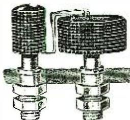
A new idea in crystal detectors is shown in the accompanying illustration. In the first place, the crystal element has a flat surface, composed of a number of very small crystals mounted together. It is stated that the great number of these makes the finding of sensitive points extremely easy. In place of the usual cat-whisker a small plate of resilient material is used. This detector may be mounted on the front of a panel; high efficiency is claimed for it.
