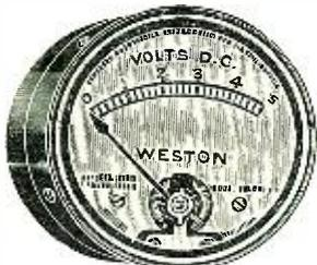
is of the highest grade construction possible, and can be used in connection with radio receivers to indicate storage battery voltage or amount of voltage used to light the filaments
