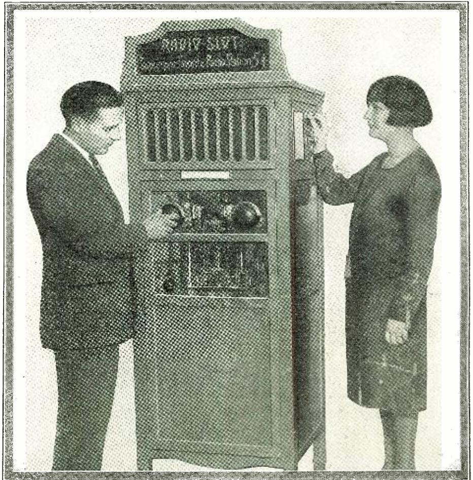
When a nickel is dropped in the slot, your favorite radio station can be tuned-in by the two dials on the front of the cabinet.
