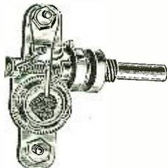
F. H. Noble Co., 29 East Madison Street, Chicago, Ill. This multi-point panel crystal detector was tested in conjunction with an ordinary crystal set and reflex receiver, and found to be satisfactory. It is of solid and efficient construction as the illustration shows and has a multi-point catwhisker.
