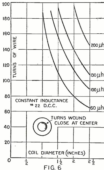
FIG. 6 At the left it is shown how the inductance varies with the number of turns (wound touching at center); above, the relation between the coil diameter and the number of turns; and on the right the effect of varying the coil diameter. Note how slowly the inductance increases compared with the number of turns, for the small diameters.
