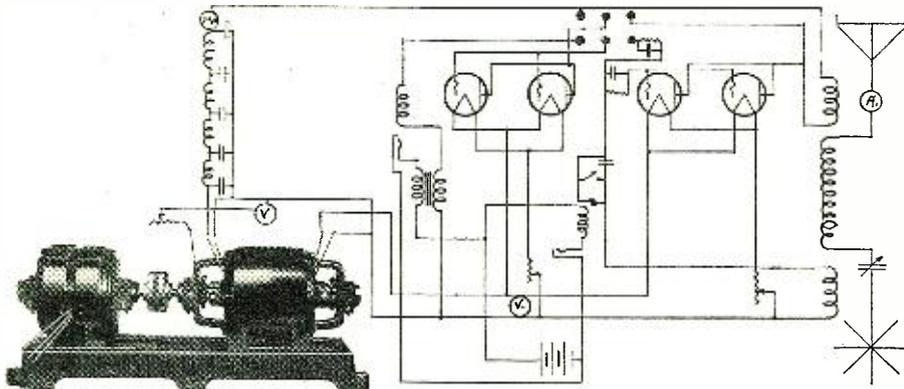
There is no question about the Miles per Watt with ESCO—it is the maximum. Item 35. Two unit four bearing set. Furnished with ring oiled or ball bearing Motor to suit local supply. This "ESCO" set delivers 1000 volts, 300 watts for plate supply and 12 volts, 150 watts for filament supply. This set driving two 50 watters will make a good consistent station.
