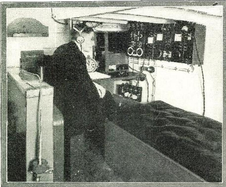
Interior of wireless cabin, showing Radio Operator Gilbert Moss, seated before his instruments. Behind him, on the deck, is the loop antenna, unshipped. In the corner of the bench is the 1/4 K.W. quenched spark transmitter, and on the bulkhead in front of Mr. Moss is the 6-tube radio compass receiver and the 2-tube all-wave receiver, both fitted for alternative crystal operation. Photos © Marconi Wireless Telegraph Co., Ltd.
