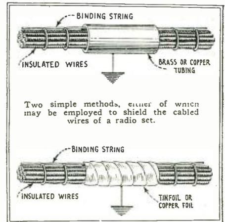
Two simple methods, either of which may be employed to shield the cabled wires of a radio set.
