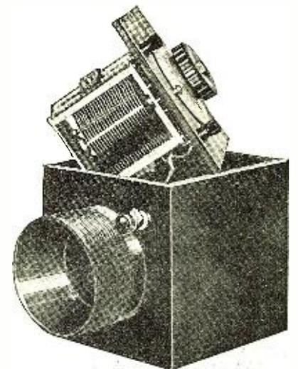
A standard type of wave-trap that will increase the selectivity of circuits is shown in the photograph above.
