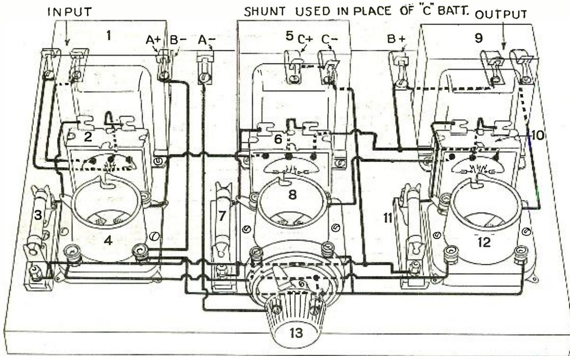
The bread-board layouts on these pages have been made because they show exactly how the amplifier will look when built into a complete set. The only difference will be found in the position of the rheostat controlling the filament current, which is generally mounted on the panel. To tell the truth, it may as well be mounted in back of the panel, for it is seldom necessary to adjust it, provided, of course, that a filament switch is included in the circuit.
