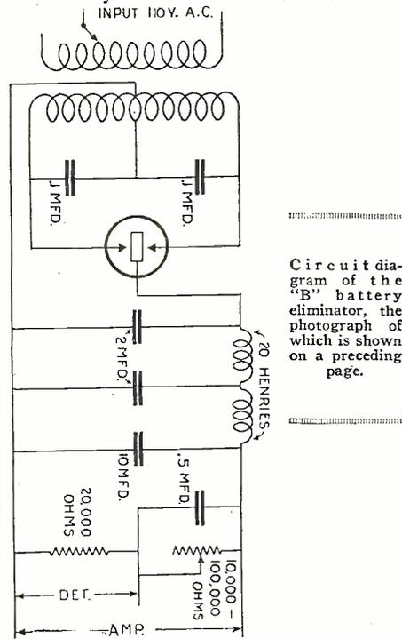
Circuit diagram of the "B" battery eliminator, the photograph of which is shown on a preceding page.
