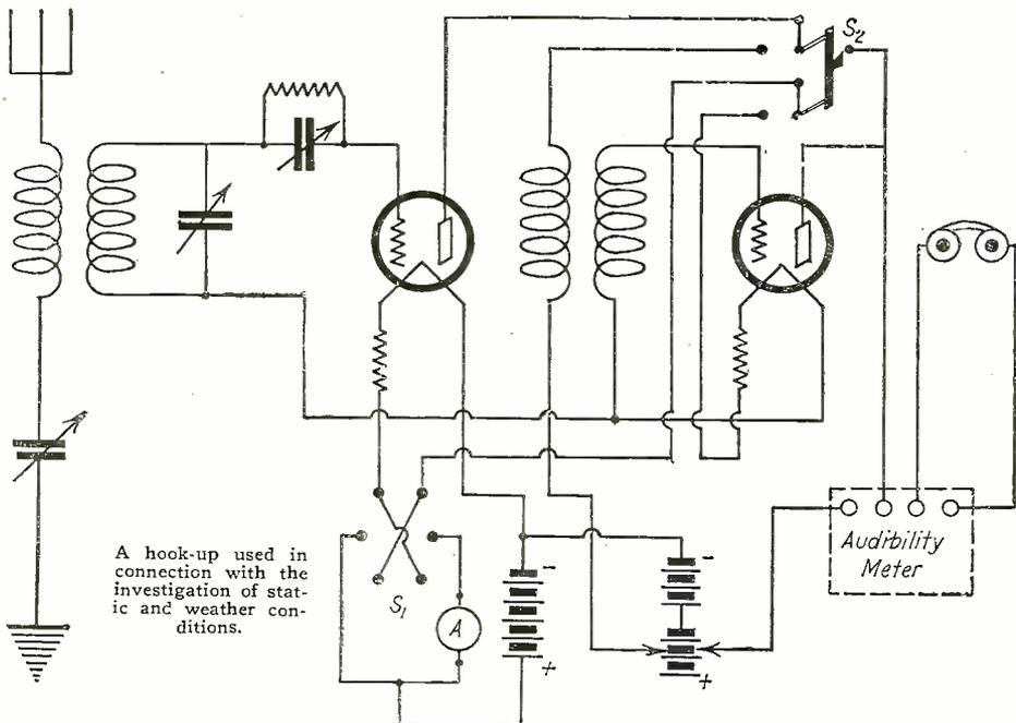
A hook-up used in connection with the investigation of static and weather conditions.
