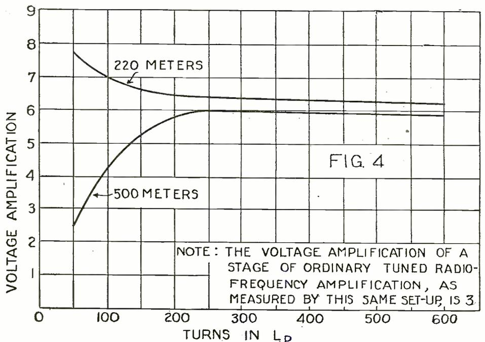
NOTE: THE VOLTAGE AMPLIFICATION OF A STAGE OF ORDINARY TUNED RADIO-FREQUENCY AMPLIFICATION, AS MEASURED BY THIS SAME SET-UP, IS 3.
