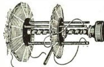
The carriage of the English basket-weave coil holder shown herewith is driven by the central screw. These carriages are so constructed that coils of different sizes may be substituted.
