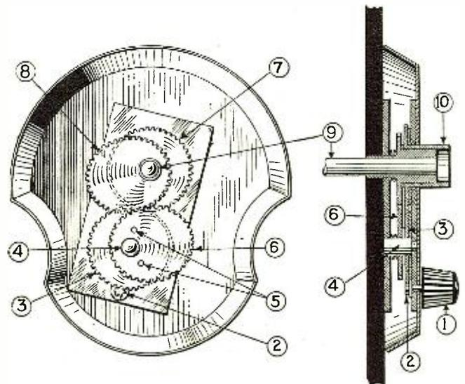
Pinion 2 turns circular gear 3, also turning circular gear 7, to which the dial pointer is fastened, at the same time. Elliptical gear 6 is carried (rigidly) by 3, and rotates elliptical gear, which moves the condenser shaft, at 9, at a variable rate.
