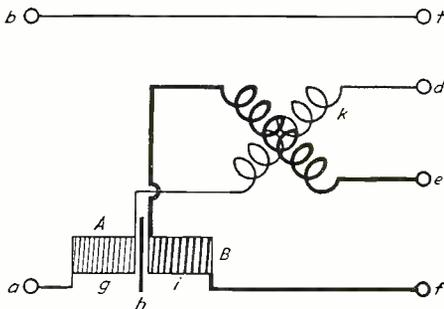
Fig. 4. Circuit diagram of the stereophone as developed by Dr. Kluth is shown above.
