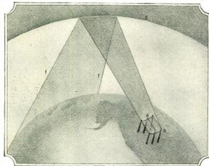
Fig. 2. According to Fessenden, if waves were radiated from a horizontal antenna and reflected so that the beam reaching the Kennelly-Heaviside layer would be wide and be reflected again from a large area, fading would be considerably reduced. In the illustration, (a) is the antenna, (b) the reflector, (c) the Kennelly-Heaviside layer, and (d, e, f) edges of the reflected beam.
