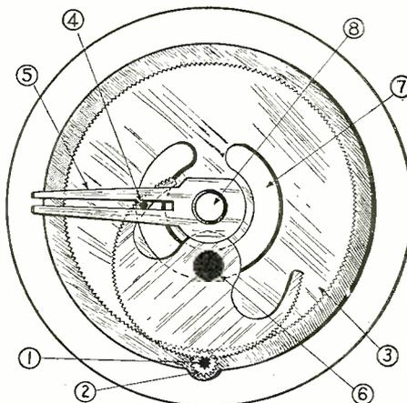
Pinion 2 rotates plate 3, which carries the calibration scale. Pinion 1 moves the sector about the center 6. Pin 4, fastened on sector, thus changes its radius (distance from 8) in arm 5. The smaller the radius the faster the arm (5) revolves about 8, which carries the condenser shaft.
