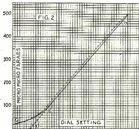
The characteristic curve of a condenser may be obtained within a few micro-microfarads by the experimenter.
