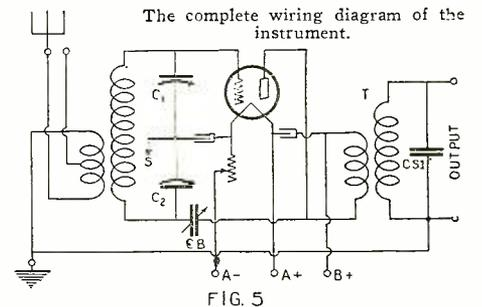
circuit diagram for the type used with sets designed for antenna reception. It will be noticed that the shield marked S is not connected directly to the ground, but through a by-pass condenser. While this grounds the shield and the rotor of the twin variable condensers to alternating currents, it removes the possibility of burning out a tube by having the posi-
