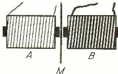
Fig. 3. The membrane, M, vibrating between two electro-magnets produces a phase displacement of 180 degrees in a telephone circuit.
