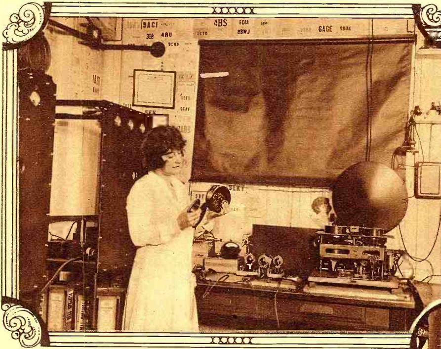
RECORDING VOICES ON ELECTRICALLY CHARGED WIRES. The method of recording on wires was discovered a quarter of a century ago by Valdemar Poulsen, a Danish inventor, but the system was impractical until the vacuum tubes could be used for amplifying signals. © International Newsreel.
