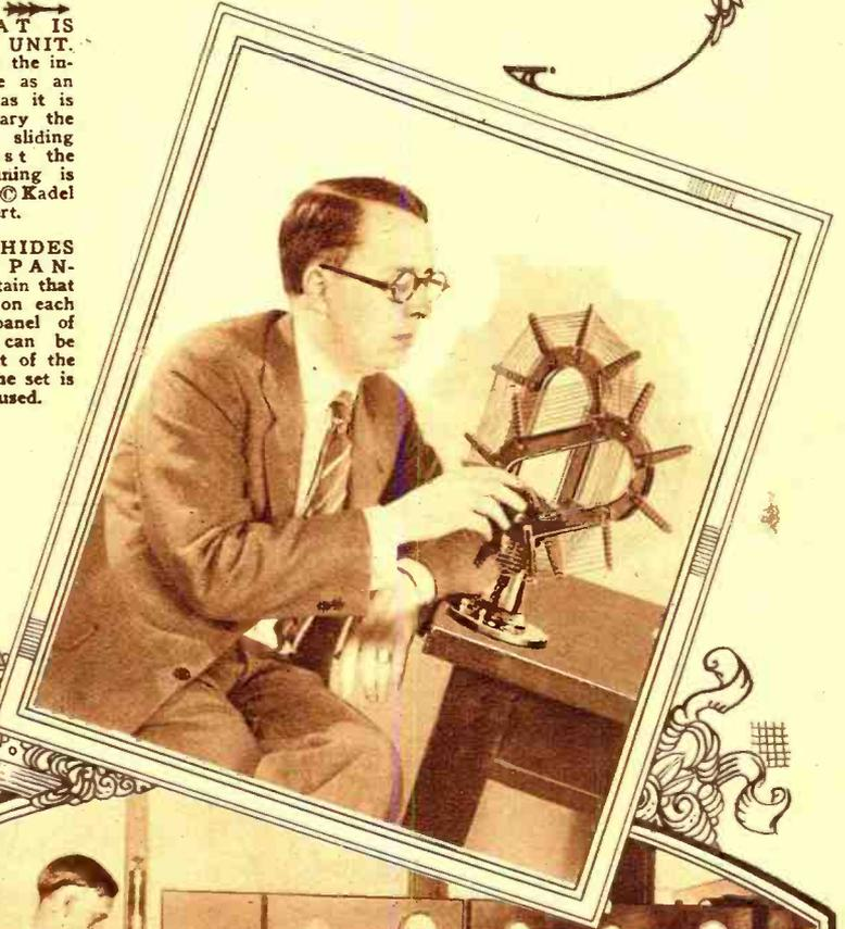
**CRYSTAL SOLVES INTERFERENCE PROBLEM.** The installation of a piezo-electric crystal in the transmitting circuit keeps the transmitter exactly on the desired wave-length, eliminating any possible interference with other stations. The crystal is shown over the man's right hand.
