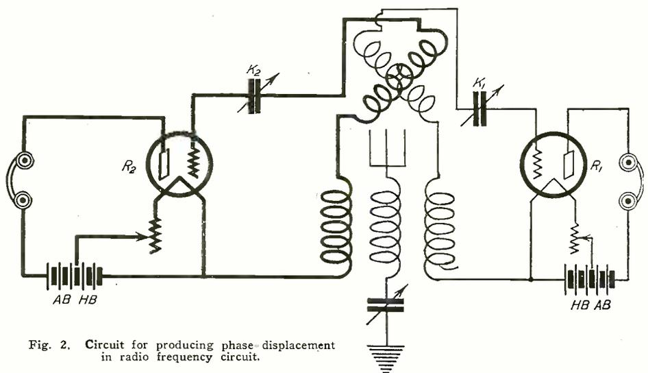
Fig. 2. Circuit for producing phase-displacement in radio frequency circuit.
