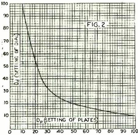
This chart shows the relation between the plate setting and dial setting, as determined from Fig. 1.
