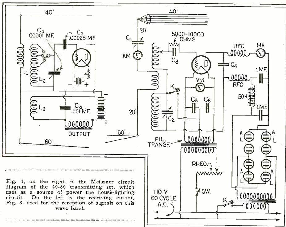
Fig. 1, on the right, is the Meissner circuit diagram of the 40-80 transmitting set, which uses as a source of power the house-lighting circuit. On the left is the receiving circuit, Fig. 3, used for the reception of signals on this wave band.
