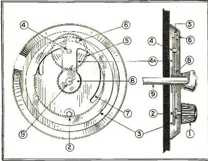
Knob 1 turns pinion 2, which rotates ring-gear 3. This carries pin 6 in groove 7. Gear 5 thus rotates slightly, changing the angular acceleration of arm 4 (a), which turns the condenser shaft at 9.
