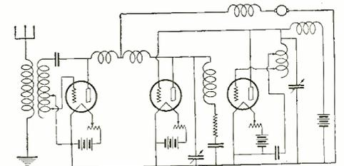
taneous transmitting and receiving. A grounded aerial circuit is provided with a tuning inductance connected thereto and a divided secondary circuit across one portion of which the input circuit of the tube is connected and across the other portion of which the output circuit is connected.
