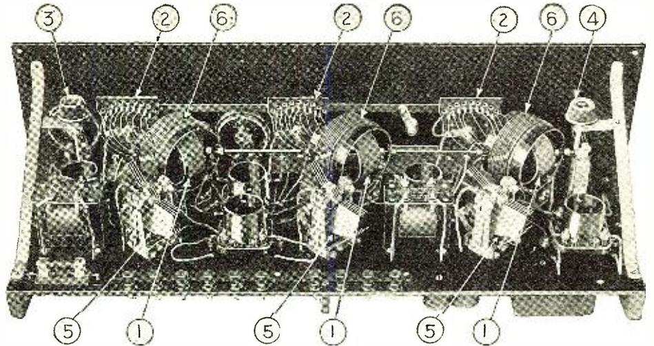
The interior of the five-tube receiver. The coils marked 1 are the rotors on which are wound part of the secondaries; the parts, 2, are the inductance tandem switches; 3 and 4 are filament rheostats; the condensers, 5, are the semi-fixed capacities across the secondaries, and the coils marked 6 are the primary and part of the secondaries.
