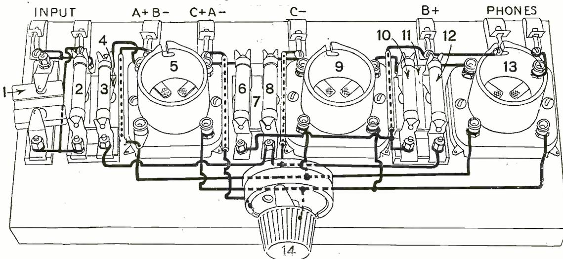
Resistance-coupled amplifier. 3, 8, 12—first, second and third stage grid resistances. 2, 6, 10—coupling resistances of each stage. 4, 7, 11—stopping condensers. 1—by-pass condenser.
