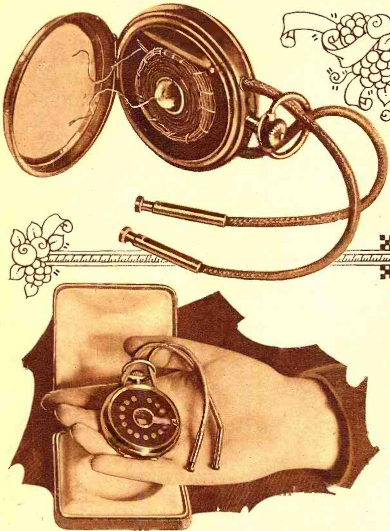
**WATCH-CASE CRYSTAL RECEIVER.** One of the unique sets that was entered in the Radio News Home-Built Set Contest is shown above. The wires shown are the antenna and ground leads, a condenser is in the cover of the case and the taps of the coil are brought out on the face of the watch. The phone tips fit into small jacks at the bottom of the case.
