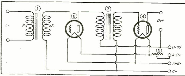
Wiring diagram of the transformer coupled amplifier which is shown in the photo above.
