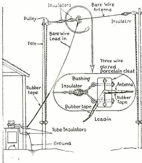
An antenna insulator of this type is both cheap and efficient.
