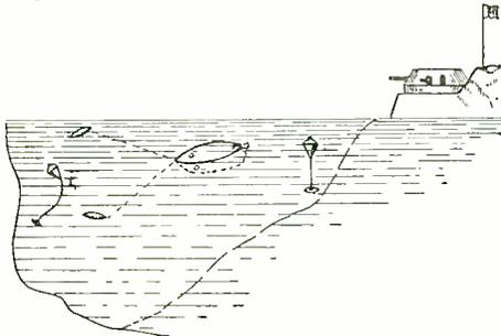
transmission system is illustrated whereby received radio signals are caused to actuate a submarine compression wave sound transmission system for transmitting energy under water for control of sound-receiving devices on board the submarine vessel.
