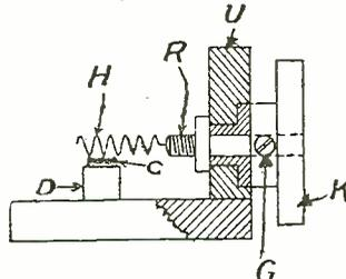
obtained between the surface of the crystal and a wire helix. Thus the crystal is held in a cup D fixed to a base B, supporting an upright bracket U, which carries an adjusting device. In the modification shown this consists of a rod R
