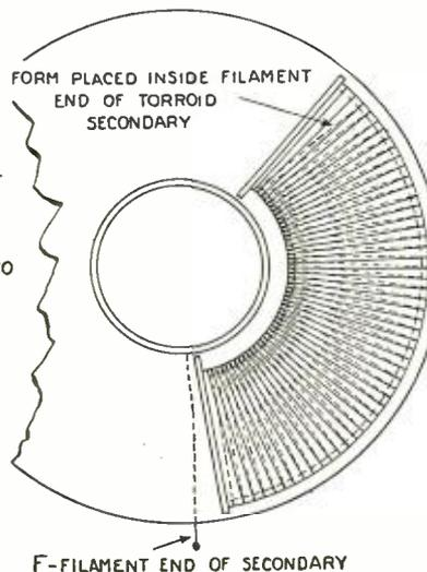
Specifications for the toroidal coils which are used for coupling the R.F. stages.
