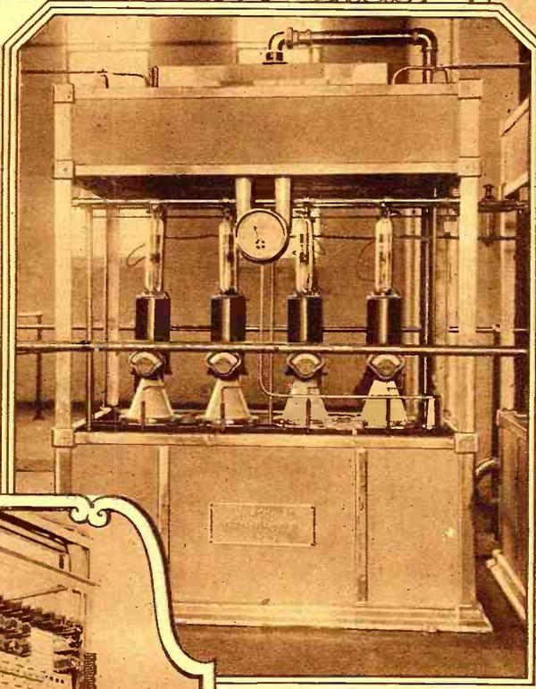
← **THE DISTRIBUTING POWER BOARD.** One of the most important units of the broadcast station is the power distribution panel, where different combinations of oscillator and modulator tubes can be made.
