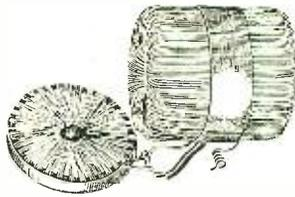
Company, 20 Grand Avenue, Brooklyn, N. Y. This toroidal coil is well built and can be used satisfactorily in tuned radio frequency amplifiers. Provision is made for primary and secondary coupling.
