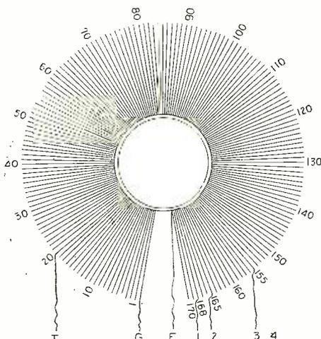
NOTE: COIL TO HAVE 170 TURNS OF NO. 24 D.S.C. WIRE TO BE TAPPED AT 168-165-155-140 AND 10 TURNS FROM GRID END. NO INSIDE COIL TAPS 1, 2, 3, 4, G, F, & T. FOR ANTENNA COIL T A ON COUPLING COILS BETWEEN TUBES T C - NOT TAPPED AT 1, 2, 3, 4, TAPPED ONLY AT T 20 TURNS FROM G.
