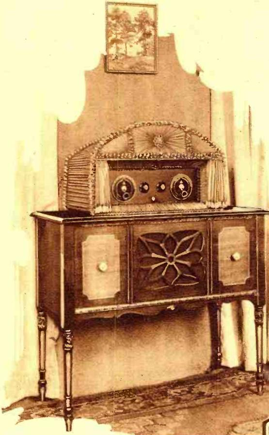
**LOOP THAT IS TUNING UNIT.** Not only does the inductance serve as an antenna, but as it is possible to vary the inductance by sliding one loop past the other, the tuning is accomplished. © Kadel & Herbert.
