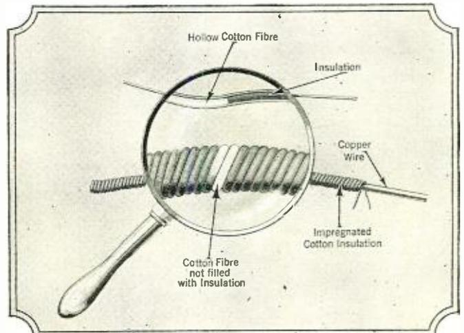
was sawed across with a hack saw and brought me, with the cut surface showing like the section of a submarine cable.
