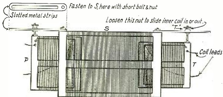
just the coupling simply loosen the thumb nut, T, and slide the coil in or out to the proper position and then tighten the nut.
