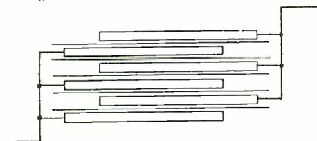
coated with rubber in solution which, when dry, forms an insulating filament directly upon the conducting plate, permitting condensers to be built up by stacking the conducting plates one upon another.
