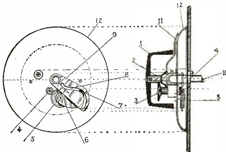
Through a vernier attachment controlled by knob 1, pinion 4 rotates gear 5 and the arm 6. The pin 7 slides in slot 8 in arm 9, which rotates the condenser at charging rates.
