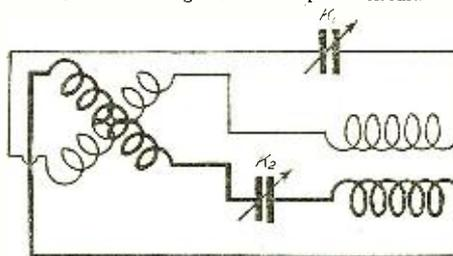
Fig. 1. Simple circuit illustrating an arrangement for setting up a phase displacement from 0 to 360 degrees using a variocoupler.
