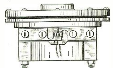
armature is arranged within the electro-magnetic field and is actuated by the variations in the magnetic flux in such manner that all of the vibrations are effectively employed for the reproduction of signals.
