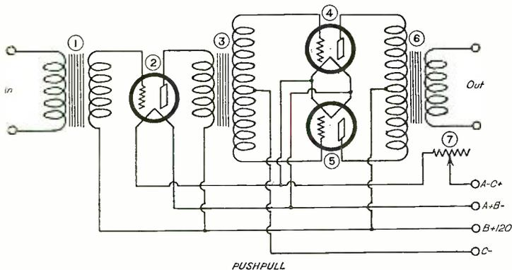
Wiring diagram of the push-pull amplifier.
