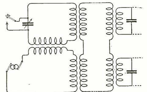
separate circuits in which two series of impulses of radiant energy having a predetermined phase difference may be utilized to control the operation of selenium cells at a receiver which, in turn, control circuits at the receiving station to selectively actuate the receiving mechanism.
