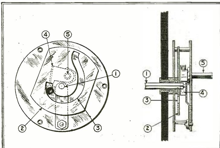
Shaft 5 turns plate 2, which carries a pin travelling in slot 3. This rotates arm 4 and condenser shaft 5. The distance (or radius) between the center 1 and the pin thus continually changes.
