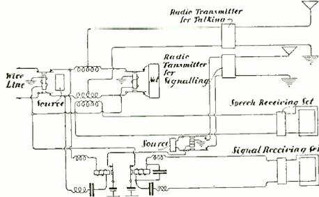
currents or telegraph signaling currents. The switching means is actuated by signaling currents transmitted over the line for connecting the modulating circuit in desired relation to the antenna system and control circuits.
