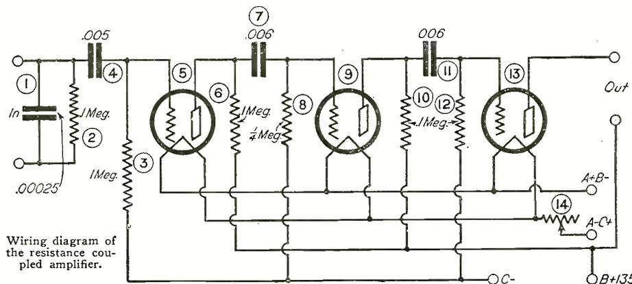
Wiring diagram of the resistance coupled amplifier.
