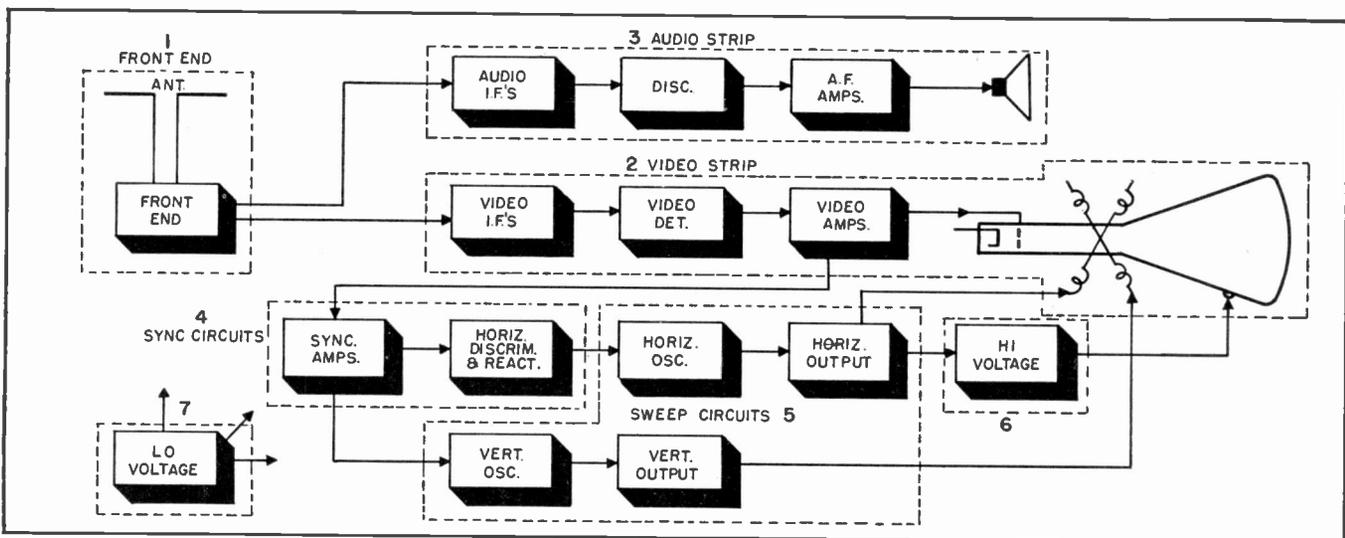
Fig. 1 Block diagram of the RCA-630-TS type receiver. Knowing the function of each of the sections of this type of receiver
