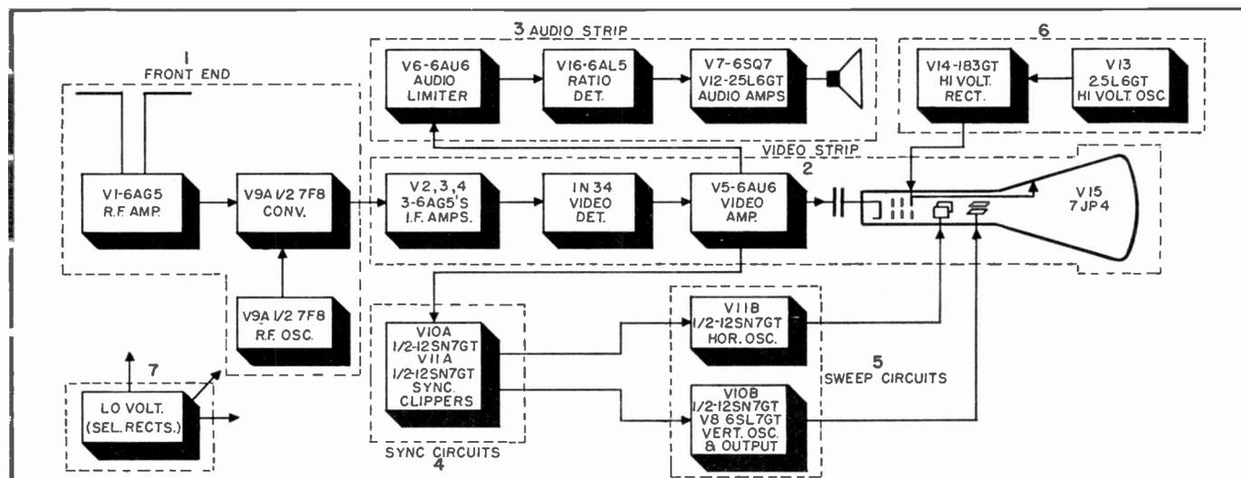
Fig. 2 The basic block diagram of the 7-inch receiver, using static deflection and focusing, inter-carrier sound system, and
