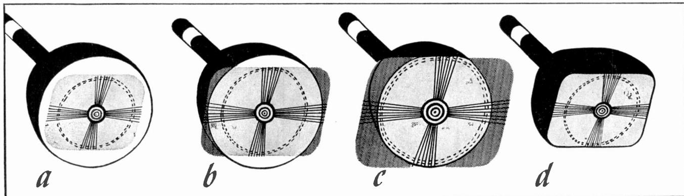
Fig. 1 Reproducing rectangular transmission on circular screen. A) 25% of tube face area lost. B) 14% of face area,
