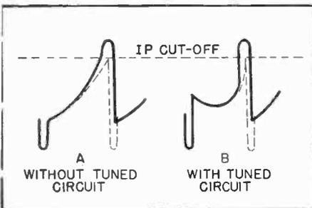
Fig. 5 Comparison of a-f-c waveshapes, with and without additional tuned circuit in plate of blocking oscillator.
