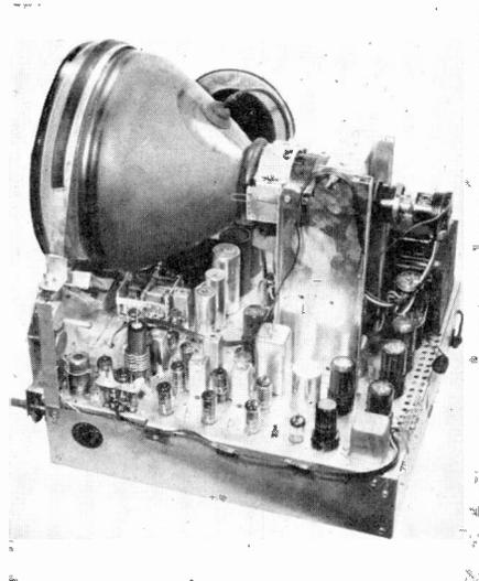
The high-voltage system (Section 6) is of the fly-back type, and must receive the horizontal sawtooth in order to operate. It provides the large amount of voltage necessary to bring the beam from the cathode of the picture tube to the screen at a high enough speed to give the required brightness.
