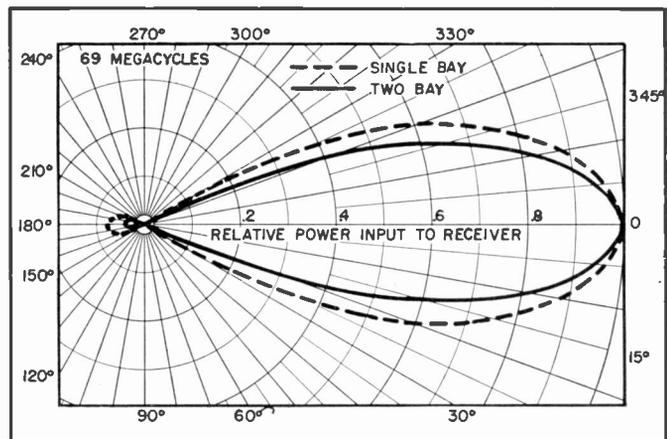
Fig. 2 Horizontal radiation pattern of Twin Driven Yagi, for both single and two-bay arrays, measured at 69 megacycles
