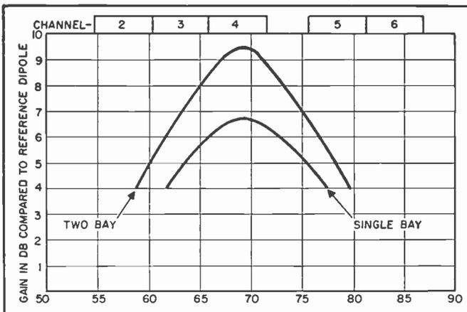
Fig. 1 Measured gain of new antenna in db, compared to standard dipole. Curves are for both signal and two-bay arrays
