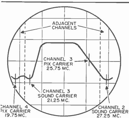
Fig. 2 Typical video i-f response curve
