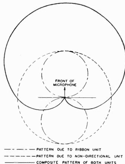
Fig. 5 Addition and subtraction of the sound energy received by the two sections of the uni-directional microphone produce the overall pattern known as a "cardioid."
