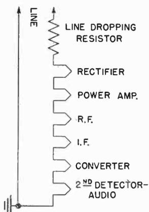
Fig. 1. Typical tube sequence for series-operated filaments.
