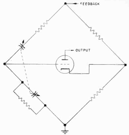
Fig. 1 Simplified schematic of bridge circuit for resistance-capacity oscillator.
