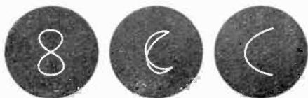
Fig. 3. Three possible forms of patterns obtainable with 2:1 frequency ratio applied to the plates of oscillograph.
