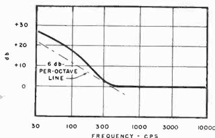
Fig. 2 Frequency response curve for network.
