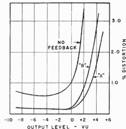
Fig. 6 Distortion curves for complete amplifier.
