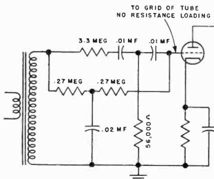
Fig. 1 R-C network in grid circuit of input stage to compensate for droop in low-frequency response of magnetic pickups.
