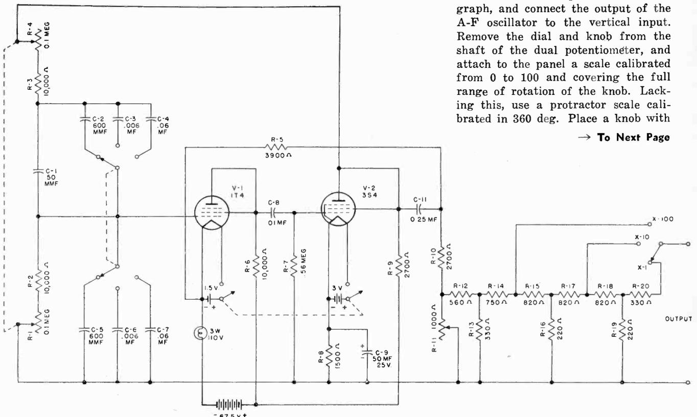
Fig. 2 Complete schematic of the midget audio-frequency oscillator.
