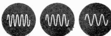
Fig. 5. Patterns on oscillograph screen corresponding to 3:1, 4:1, and 5:1 frequency ratios.
