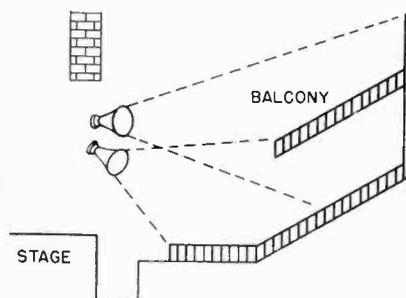
**Fig. 7** Arrangement of loudspeakers for the most efficient coverage of orchestra and balcony seats in a theatre with using speakers with wide angles of distribution.
