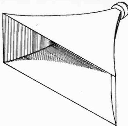
**Fig. 8** One form of speaker suitable for sound distribution over a long, low area, such as a grandstand.
