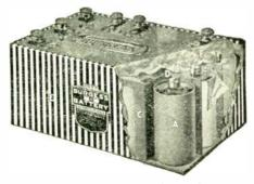
"A" is the Burgess one-piece seamless zinc can which requires heavier, more pure and more uniform metal than a soldered can, all of which add to the life of the cell. Also, it prevents any leakage through a weak joint and eliminates voltage differences on the inside of the can, a condition which might cause stray currents and potential differences and results in noisy voltage fluctuations and short-lived battery.
