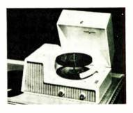
An automatic table model phonograph developed for playing Columbia and RCA 7-inch records automatically. Model 745 is a two-speed changer with velocity trip, 3-second cycle change "music to music," controlled tone arm performance, and non-record slippage. Housed in plastic, unit has self-contained amplifier and speaker.
