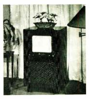
One of ITI's "Century" line of television receivers, this model has a 12½-inch cathode-ray tubes which gives an 85-square-inch picture. Eighteen tubes and three rectifiers: "Visual Tuning" and simplified controls. Available in cabinets of dark or bleached mahogany.
