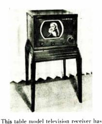
a 10-inch cathode-ray tube and yields a 61-square-inch picture. Provides coverage on all television channels. Priced at \$199.95, less table.
