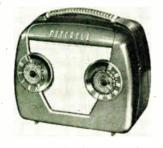
This radio weighs four pounds and operates from batteries only. Has specially designed Hi-Q 1F transformers. cosmalite forms and silver mica capacitors for maximum performance and stability. Loop antenna is built into back of set.
