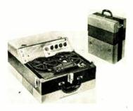
Portable tape recorder for recording and reproduction of sound. Recordings are made through microphone or directly from radio or record player and are played back through compact amplifier and speaker. Automatic rewind at end of forward movement of each reel. Recording speed constant. Ribbon can be edited and spliced. Microphone is non-directional, crystal. Output and input jacks allow playing through external speakers, recording other than through microphone.
