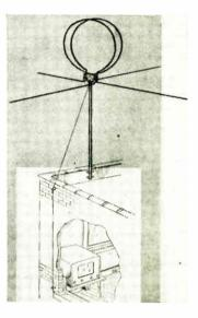
Consisting of two loops and two dipole sections 90 degrees out of phase, the Quad-Loop is a quadrature phasing antenna. It is a stationary antenna which achieves the effect of a rotated one by using a phasing device located at the receiver. Loops provide high frequency TV reception, dipoles the low. Needs no orientation when installed.
