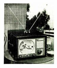
This 7-inch, portable television set operates on AC or DC current. Indoor aerial which goes with installation has separate plug-in base and lead-in wire for attaching antenna at best reception points. Housed in simulated leather case, with protective carrying case for traveling.
