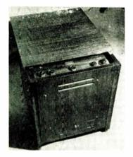
With 36 tubes, including picture tube. and six rectifiers, this chairside projection model in crotch mahogany throws a 3- by 4-foot picture on a home movie type screen. Cabinet measures 23 inches high, 21 wide and 26 long. Small doors in cabinet open to reveal the Proj-Tel unit, which houses projection system. Top slides forward to expose controls on back of cabinet. Set plugs into standard outlets, requires no special antennas, Say you saw it in Radio & Television Journal, June, 1949
