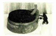
Primarily styled for children, this toy phonograph is constructed like the larger, more expensive units, employing two tubes, one as an amplifier and another as a rectifier. Built with all standard radio parts and is approved by underwriters lab. Also equipped with a high output pickup and four-inch permanent magnet speaker. Case is finished in blue, with lithographed figures in white.
