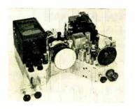
This is a modified version of the 630 circuit designed to accommodate STPR projection tube. Intense source of light on face of projection tube enables projection of image onto screens of sufficient size for large audiences. Contains 30 tubes, full 13 channel coverage, FM sound system, exclusive cut-out relay to protect projection kinescope in the event of sweep failure.
