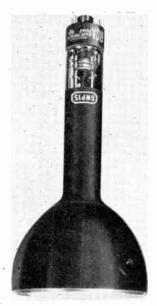
This new Flying-Spot tube furnishes a small, rapidly moving spot of radiant energy for scanning a slide transparency or opaque object. It thus makes possible a relatively simple and inexpensive videosignal generator capable of producing not only a repetitive picture signal like the monoscope, but also of permitting change of picture at will and of reproducing the picture with the halftone fidelity of photographic film.
