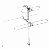
A newly designed antenna for 44 meg. to 216 meg. broadband signal reception in a stacked parallel feed system and employs a folded-dipole and reflector with a high front to back ratio, giving a maximum unwanted signal rejection factor.
