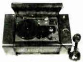
Called the Wiretone, this table model wire recorder includes both a radio and a phonograph and sells at about \$150. The cabinet is made out of a combination plastic and wood with walnut finish. The machine will record electronically from either the radio or the phonograph. People talking in a normal voice 25 feet away from the microphone will reproduce easily.
