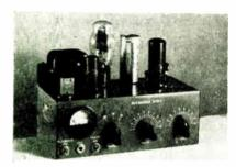
Micamold Radio Corporation, Brooklyn. N. Y., announces the first of a line of amateur radio equipment which it calls a CW Transmitter Kit. The kit includes all parts and complete instructions to assemble a well-engineered transmitter which is rated at 45 watts input to the final amplifier. Please mention RADIO & APPLIANCE JOURNAL, December, 1947 when writing to manufacturer.
