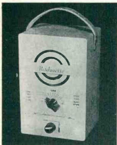
Model PR-1, a personal portable radio, has been introduced by Alamo Electronics Corp., 105 W. Romana, San Antonio, Texas. Set is 4 tube superheterodyne with 4 inch P.M. speaker and loop antenna. Case is plywood covered with Du Pont leatherette; plastic front has engraved dial. Total weight including batteries is 4½ pounds. Please mention RADIO & APPLIANCE, Oct., 1947, when writing to manufacturer.
