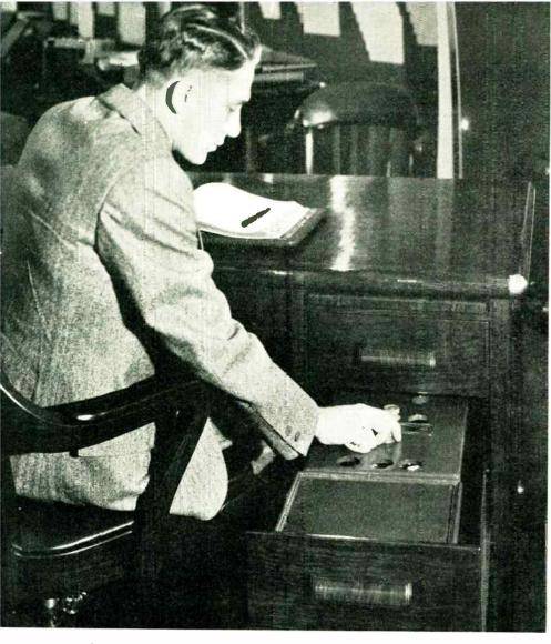
Shaw-Walker desk equipped with General Motors radio. In the front of the chassis is the speaker, which is silenced when the drawer is pushed in.
