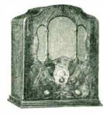
New detector-oscillator system has been designed for the Sentinel 116, five-tube super-heterodyne. Cabinet is 15¾ inches high, 13¼ inches wide and 8 inches deep. A 24 tube is used combined in first detector and oscillator, a 24 as second detector, a 35 in the intermediate-frequency, and a 47 in the output.
