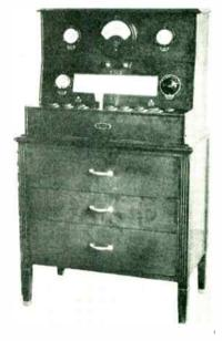
The Acremeter provides a visible tube test
