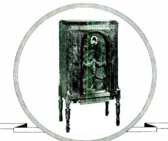
MODEL 17—Lowboy walnut console of distinctive design. Superheterodyne, 9 tubes. Color tone control, Brunswick Uni-Selector, automatic volume control, dynatron oscillator, turret type tuning condenser, 12" super-dynamic speaker, two pentode tubes in output stage and power detector. Dimensions 414" high, 214" wide, and 134" deep. List price, complete with Brunswick tubes . . . \$140.50
