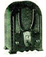
The General Electric Co.'s new midget receiver, incorporaing the pentode tube, which gives it high output, stands 151/4 ins. The cabinet, following the cathedral style, is of brown walnut finish. Chassis, including power supply system, is one complete unit, completely shielded, and employs the tuned radio frequency principle and two tuned circuits.
