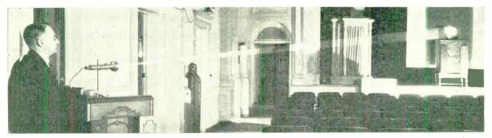
Speech and music are transmitted on a beam of light at an experiment conducted by Dr. V. K. Zworkin, research engineer of the RCA-Victor Co., Inc.
