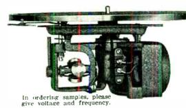
The Blue Flyer Motor unit. Like the smaller and lower-priced Green Flyer, self-starting induction type, with automatic stop equipment optional. Similar design . . . open construction with complete ventilation—no heat or hum. Silent spiral-cut fiber gears, long oversize bearings. Operates on all voltages and frequencies. Both the Blue Flyer and the Green Flyer are furnished as shown, complete with mounting plate, turn-table and speed regulator.
