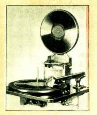
Model 10-12 in loading position. Note the lever on right side which throws the unit into position for 10-inch records when down or 12-inch records when up. With a special arrangement incorporating a double-throw master switch, one record cas be placed on the turn-table, the adjustment set according to the size of the record and the magazine can be loaded while the pick-up automatically comes into position and the first record is being played.
