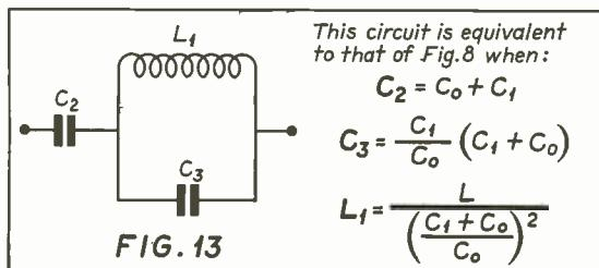
pass-band exists where the resonant frequency of the series branch coincides with the anti-resonant frequency of the shunt branch--these remarks applying to the so-called ladder type of structure; i. e., the T or  $\pi$  network. For the lattice structure, the condition for a pass-band is that the reactance of the line (series) branch shall be opposite in sign to that of the lattice (shunt) branches.
