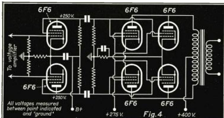
Fig. 4. The basic circuit of the resistance-coupled Class AB amplifier. The system is made possible through the use of metal-type output tubes having high power sensitivity.
