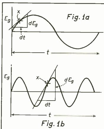
Showing effect of shock excitation: Fig. 1a, at low frequency; Fig. 1b, at high frequency.
