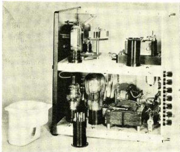
Interior view of the automatic potentiometer, showing the photo tubes on the upper deck and the rectifier and control tubes on the lower deck.
