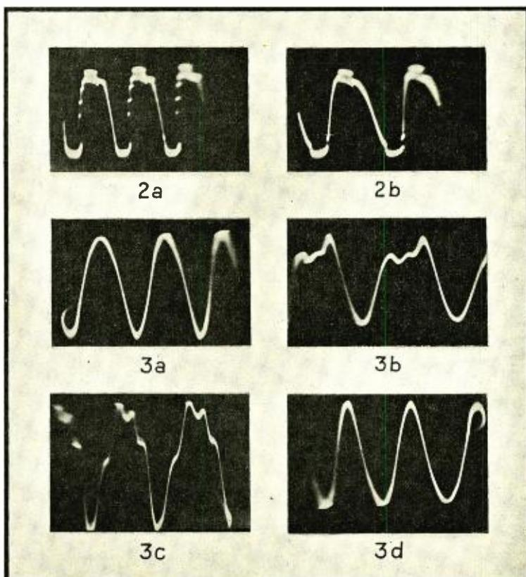
Fig. 3. A group of oscillographic photos showing waveforms obtained under various conditions of Class AB operation. Fig. 3d shows the 9000-cycle waveform obtained with the resistance-coupled method described in this article.
