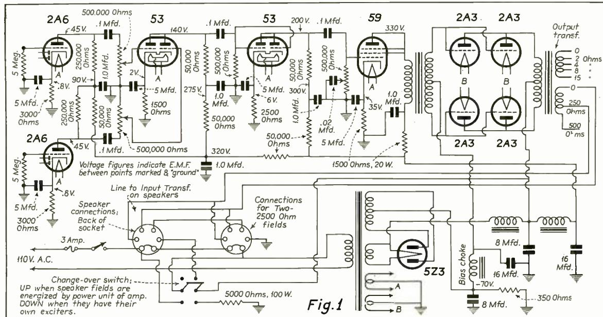
Design details of the amplifier. It has a peak output of 38 watts, gain of 124 db, hum level 42 db below sound output. Frequency-response variation between 40 and 10,000 cycles is 2 db.
