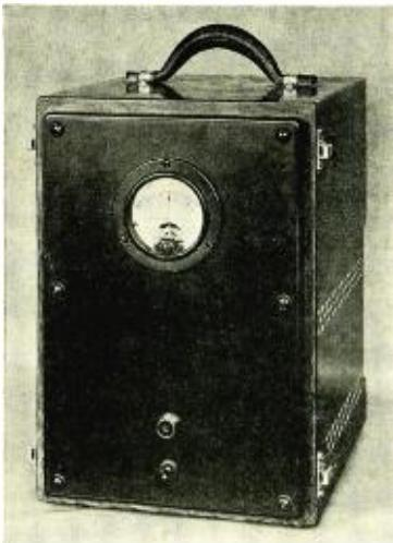
The automatic high-speed potentiometer in its carrying case.
