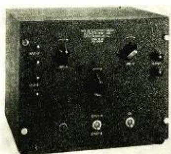
Front panel view of the electron switch for use with cathode-ray tubes.
