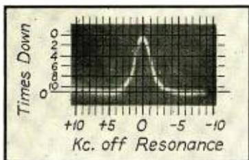
Fig. 1. Logarithmic curves obtained on screen of oscilloscope using the device described in the text.
