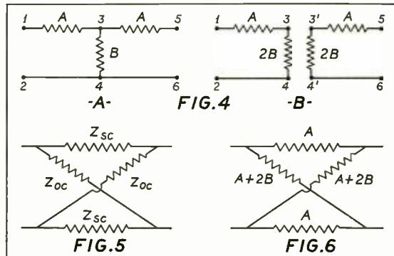
1:1 transformer. For the unity ratio case, the equivalent-T network can be physically realized, but for any other ratio the physical structure would have to have one series arm of *negative inductance*. The proof of this is easily seen if one substitutes numerical values for P, S, and M of the figure.
