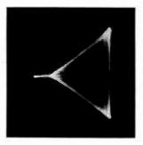
Fig. 37. Showing overmodulation.
