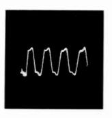
Fig. 55. Output of "squarewave" alternator with fifth and higher harmonics removed; fundamental and third present.
