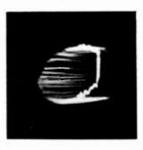
Fig. 57. Composite wave of 60-cycle pickup and commutator ripple.
