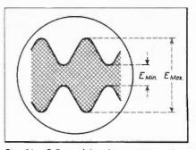
Fig. 28. R-F modulated at 1000 cycles. Timing axis supply: 500-cycle saw-tooth. Percent modulation =  $\frac{E \text{ Max.} - E \text{ Min.}}{E \text{ Max.} + E \text{ Min.}} \times 100.$
