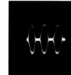
Fig. 47. Overmodulation with a-f distortion on positive peaks due to overloading.
