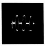
Fig. 45. Tone-modulated. Overmoculated due to overloading and insufficient r-f grid excitation.
