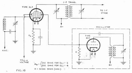
A 6L7 coupling circuit in which the total bias on  $G_3$  is augmented by the a-c component of the oscillator voltage.
