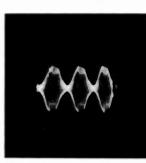
Fig. 49. Tone-modulated. Tank circuit of modulated stage defuned from resonance, showing phase distortion.
