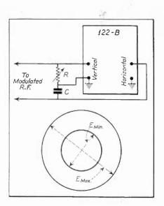
Fig. 38. When very near to 100% modulation, the inner circle, while extremely minute, will be open in the center. At exactly 100% modulation, the inner circle will simply be a spot which will increase in intensity with overmodulation.
