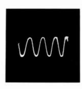
Fig. 56. Output of "squarewave" alternator; practically all harmonics filtered out, leaving fundamental only.
