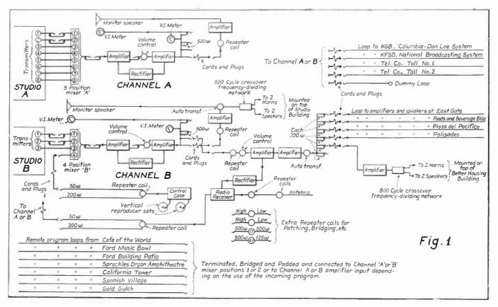
Block-diagram of the central distribution system, the heart of the audio-frequency broadcast chain.
