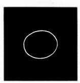
Fig. 39. Carrier only. Zero modulation.
