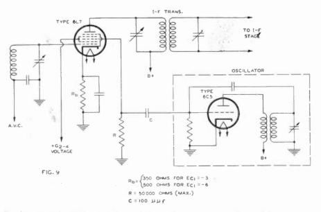
Coupling circuit for 6L7 in which the total bias on Gs is a function of the oscillator voltage.
