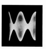
Fig. 30. A 60,000-cycle carrier modulated at 400 cycles, 75% modulation.
