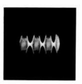
Fig. 46. Modulated trapezoid showing extreme phase distortion.
