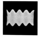
Fig. 29. A 60,000-cycle carrier modulated at 400 cycles, 25% modulation.
