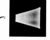
Fig. 35. Showing 50% modulation.
