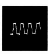
Fig. 53. Output of small "square-wave" alternator; third harmonic removed.
