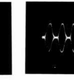
Fig. 48. Tone-modulated. Overmodulation but with reserve a-f to maintain good waveform on positive peaks.
