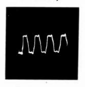
Fig. 54. Output of "squarewave" alternator with fundamental and fifth harmonic present.
