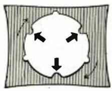
*Needs only a hole in chassis with three projections for gripping socket.*
