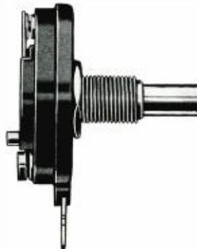
Both the switch type and the non-switch types are made very small to fit in with the new small a-c.-d-c. chassis.
