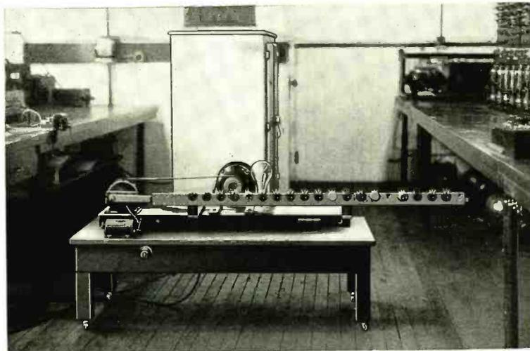
Fig. 2. Test board in the laboratory of the Stackpole Carbon Company, used to make life tests, wattage dissipation tests, voltage coefficient measurements and temperature coefficient checks on the experimental and production resistor elements.
