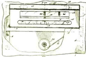
in a radio cabinet of standard construction and which is accessible from the exterior of the cabinet for permitting adjustment of the markers, and to provide improved actuation mechanism for moving an indicator and lamp in correspondence with the movements of the tuning apparatus of a radio.
