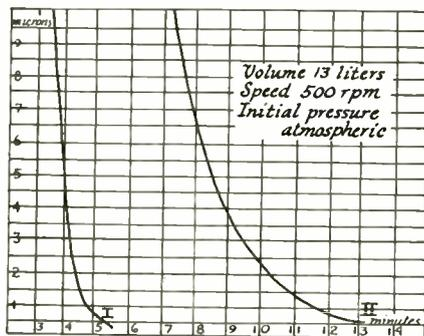
Fig. 3. Curves showing magnitude of pressure lag with two different diameters of connecting tubing.
