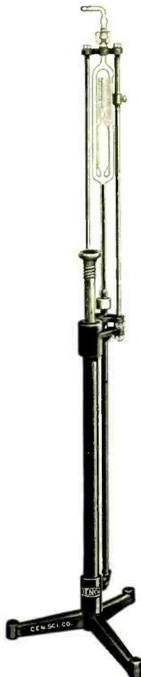
Fig. 1. Illustration of a typical McLeod gauge.
