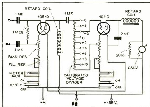
Fig. 11. Vacuum tube voltmeter suitable for measurement of audio voltages.
