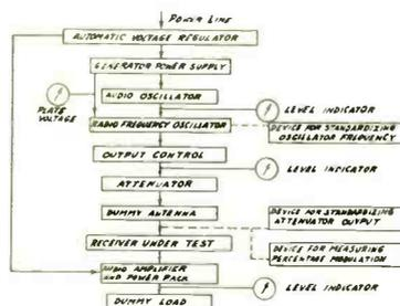
Fig. 1. Local generation system of receiver testing.
