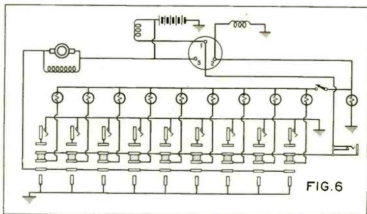
Fig. 6. Circuit diagram of the automatic transmitter unit shown in Figs. 4 and 5
