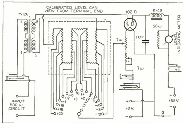
Fig. 14. Circuit diagram of the Jenkins & Adair level indicator, a panel view of which is shown in Fig. 13.
