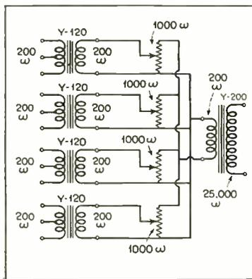
Fig. 16-A. Parallel potential divider type mixer.
