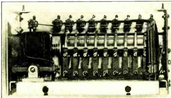
Fig. 5. Interior of the automatic radio transmitter unit. A ship's location, name and number can be sent to its base by merely pushing a button.
