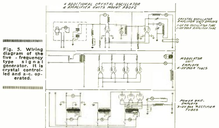
Fig. 5. Wiring diagram of the five-frequency type signal generator. It is crystal controlled and a-c. operated.
