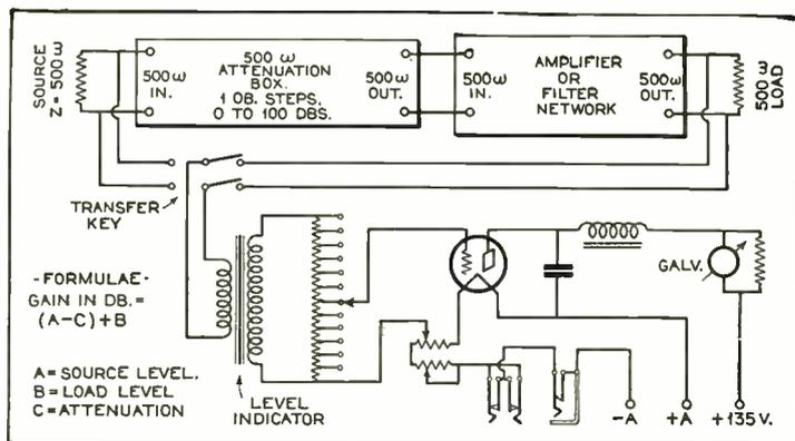
Fig. 10. Level indicator that can be used in measuring amplifier efficiency.
