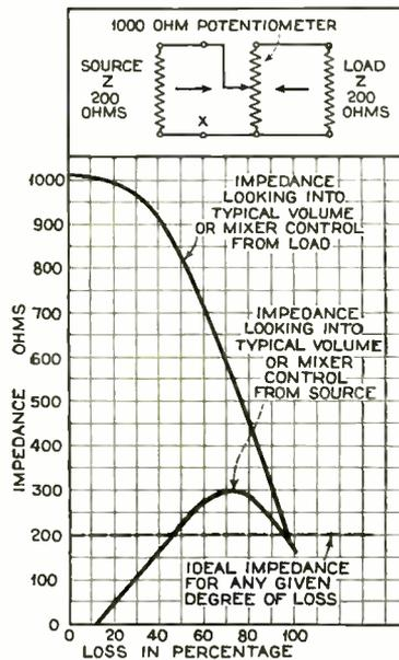
Fig. 15. Impedance curve of typical mixer.
