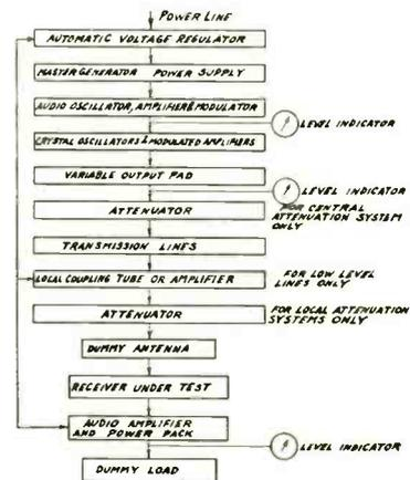
Fig. 2. Generalized central generation system of receiver testing.
