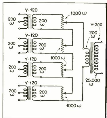
Fig. 16-B. Series potential divider type mixer.
