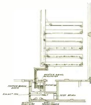
Fig. 6. General plan of the receiver testing department.
