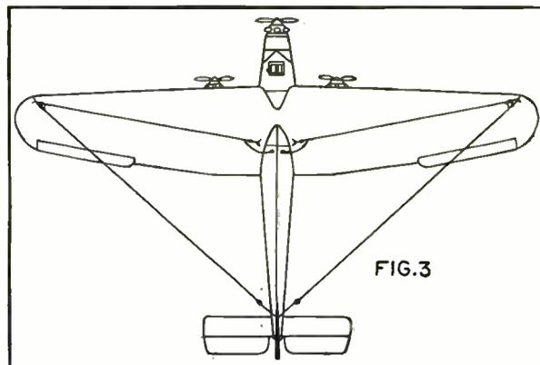
Fig. 3. A horizontal doublet antenna which, due to the size of the airplane, is easily tuned.
