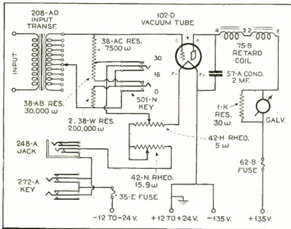
Fig. 12. Circuit diagram of the Western Electric Co. level indicator.
