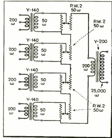
Fig. 17-B. Series constant output impedance mixer.
