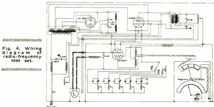
Fig. 4. Wiring diagram of radio-frequency test set.
