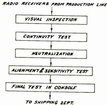
Fig. 3. Receiver inspection and test system.
