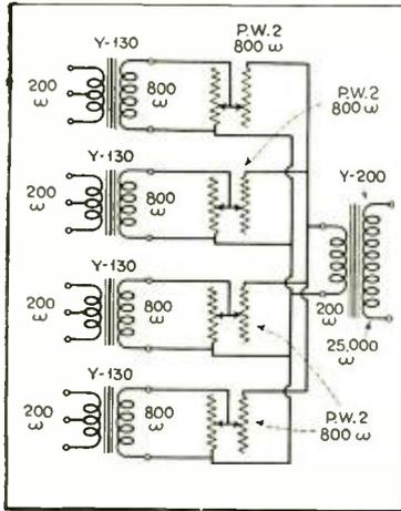
Fig. 17-A. Parallel constant output impedance mixer.
