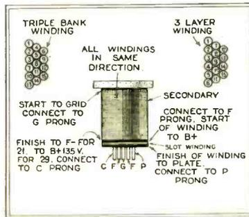
Winding details of the long wave coils.
