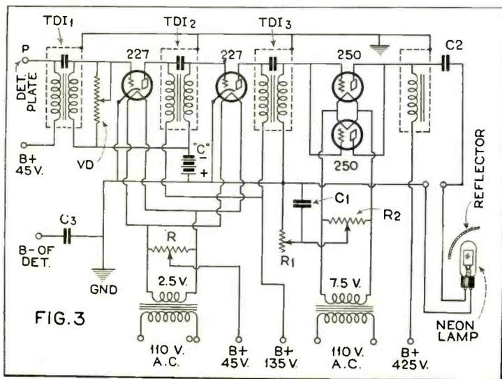
Schematic diagram of the double impedance audio amplifier which amplifies the low frequencies from the beat note oscillator before they are impressed on the neon tube.
