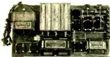
Here is the last word in a "B" Supply and Power Amplifier. Uses either a UX 250 or 210 in the last stage. Two voltage regulator tubes accurately control the 90 and 180 volt taps, thus making possible accurate determination of proper "C" voltages. There is also a 0 to 90 volt tap, variable; also 450 volts for the power tube.
