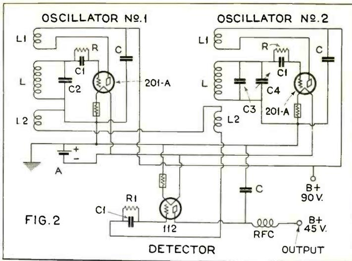
Schematic diagram of the beat note oscillator employed in connection with the neon tube to produce low light frequencies. Oscillator No. 1 is fixed.
