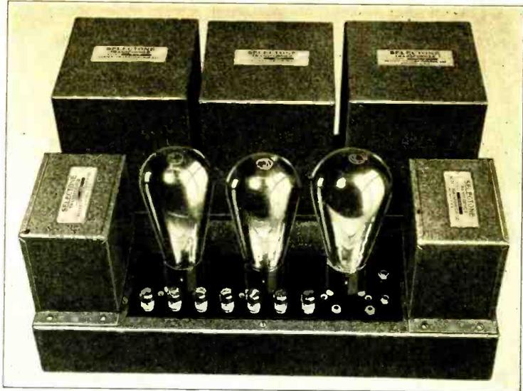
General view of the Scott Power Pack and Amplifier. The rear cases contain the power transformer, filter chokes and filter condenser block.
