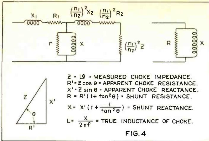
Equivalent electrical circuit of a transformer. The quantities  $X_1$  and  $R_1$  represent the primary leakage reactance.
