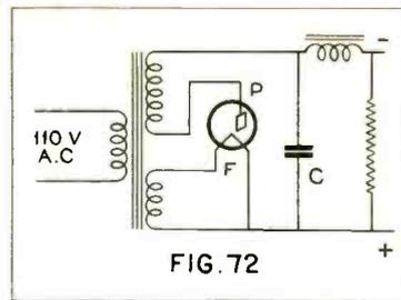
Conventional half-wave rectifier circuit, including resistance representing load.
