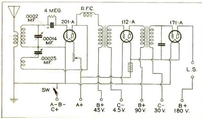
Schematic diagram of the Karas Short-Wave Receiver, employing the Weagant circuit. With plug-in coils the set covers the wavelength range from 15 to 133 meters.
