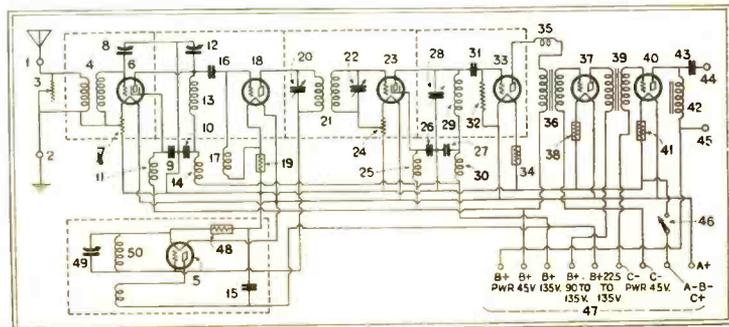
Schematic diagram of "Ultra Shield Grid Seven."
