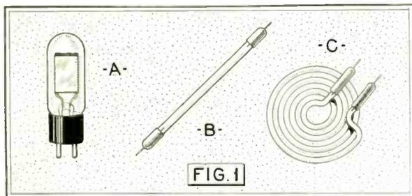
Three general types of neon tubes. A. is the square plate type, mainly associated with television work. B and C are the commercial tubular and spiral types.
