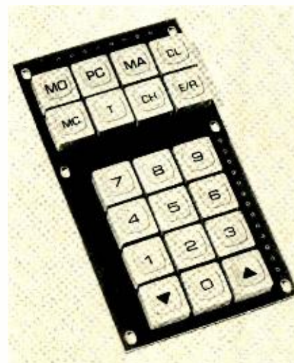
THIS KEYBOARD CONTROLS channel selection and programs a new TV set to automatically switch channels for you. It's an important part of Heath's programmer system. For full details turn to page 49.
