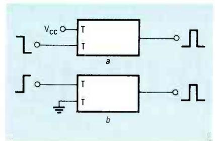
FIG. 4—THE MONOSTABLE can be configured to respond to either a rising or falling edge.
