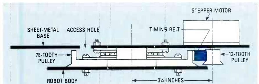
FIG. 1—THE HEAD UNIT mounts on a 78-tooth pulley. The pulley is secured to the base unit and does not rotate; instead the head rotates around it.
