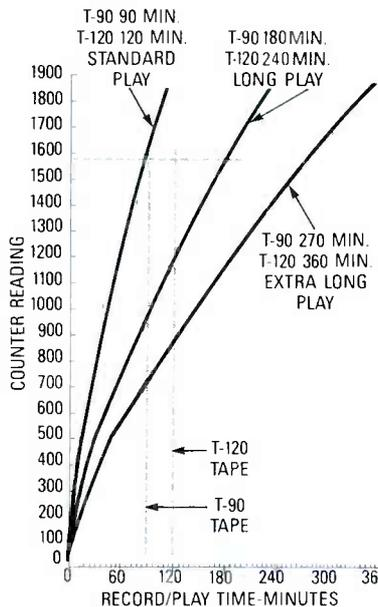
FIG. 4—USING "LONG" TAPES on the Magnavox VCR, we find that the calibrations for the 0-500 reading are exactly the same as those for the shorter tapes.
