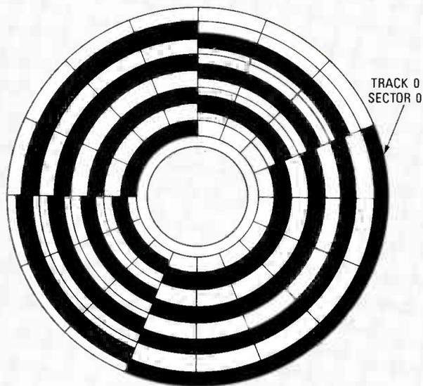
FIG. 7—A "SPIRAL" TRACK organization is achieved by offsetting alternate tracks or groups of tracks.
