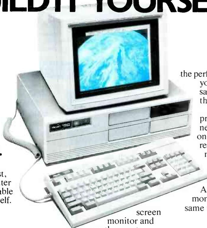
screen monitor and another port drives EGA, CGA and TTL monochrome monitors. Both ports automatically emulate common video formats for easy system configuration.
