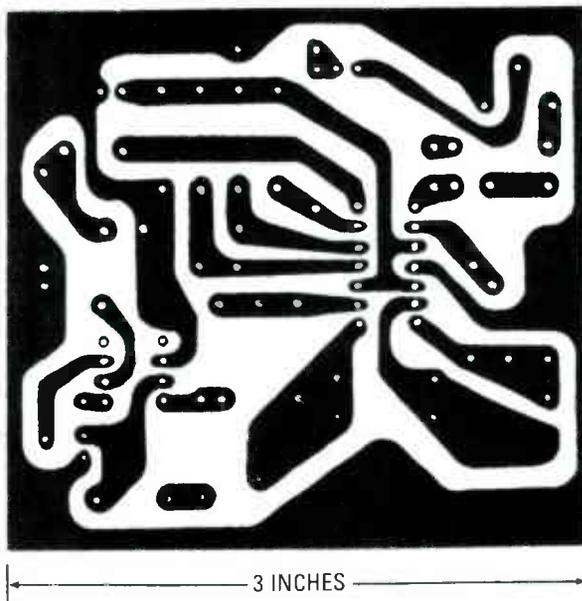
USE THIS BOARD to build the sine-wave generator circuit.
