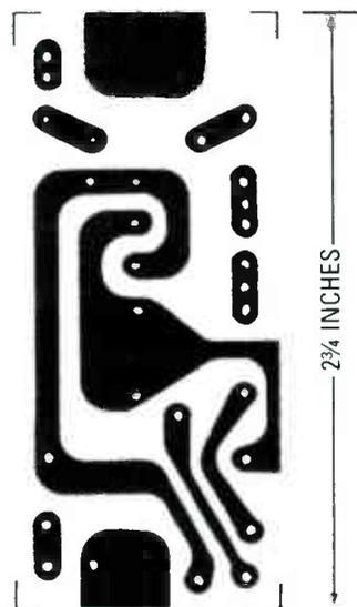
THE METER CIRCUIT can be built on this simple board.
