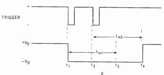
FIG. 6—A NONRETRIGGERABLE ONE-SHOT can not be retriggered until both  $t_{\sf m}$  and the refractory period have expired; the timing diagram for such a circuit is shown in a. In a retriggerable one-shot, each trigger pulse restarts the timing period,  $t_m$ ; the timing diagram for that circuit is shown in b.
