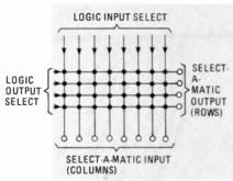
FIG. 3—IN THE SELECT-A-MATIC, switching is handled using a matrix arrangement.
