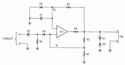
FIG. 4-AN OP-AMP BASED one-shot circuit.
