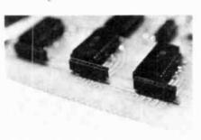
FIG. 8--HEADER STRIPS are used to make the connections between the I/O boards and the logic board.
