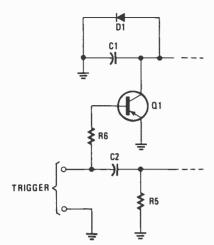
FIG. 7—THE NONRETRIGGERABLE ONE-SHOT of Fig. 4 can be turned into a retriggerable one-shot with the modification shown here.
