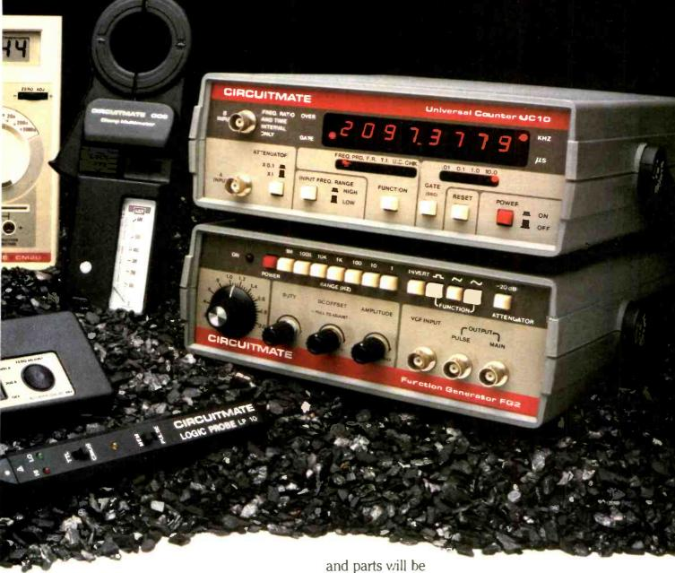
Our new circuit-powered LP10 Logic Probe is the ideal, low cost way to check TTL, DTL, HTL and CMOS signals.
