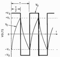
FIG. 9—TIMING DIAGRAM for the circuit shown in Fig. 8.
