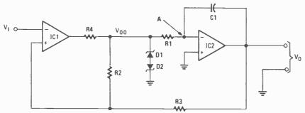
FIG. 14—THIS TRIANGULAR-waveform generator includes an integral squarewave generator.
