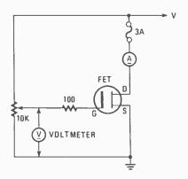
FIG. 12—TO CHECK THE MATCHING OF TRAN-SISTORS, you might want to use this simple circuit. Start by setting the potentiometer's wiper voltage to zero. Then turn it up to the desired drain current and measure the voltage as shown. For N-channel devices (IRF630), V should be 5 volts. For P-channel devices (IRF9630), V should be 5 volts.
