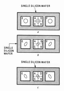
FIG. 7—PHOTODIODES are used to keep the videodisc perfectly in focus. The ones in a show a disc in focus, the ones in b show a disc that is too far away, and the ones in c show a disc that is too close.
