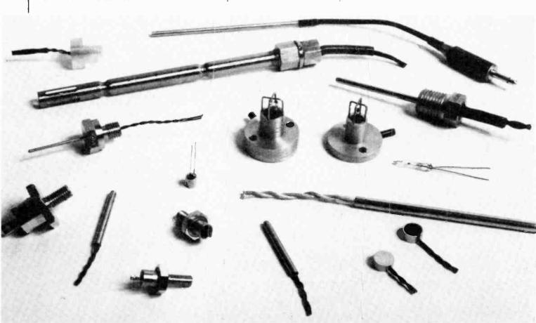
NTC thermistors are narrow-range, nighly sensitive, nonlinear devices whose resistances decrease with increasing temperature. Figure 1—a curve relating resistance change to temperature—shows typical resistance-temperature characteristics. The sensitivity is about 4–5%/°C (1°C = 2.5°F). A wide range of resistance is available, and resistance changes may be many ohms or even kilohms per degree.
