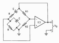
FIG. 16—THIS WIEN-BRIDGE OSCILLATOR can also be used to generate a sinewave output,
