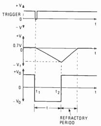
FIG. 5-TIMING WAVEFORMS for the circuit shown in Fig. 4. Note that the one-shot can not be retriggered until both the period t and the refractory period have expired.
