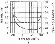
FIG. 3—TEMPERATURE AND RESISTANCE TOLERANCE for precision interchangeable thermistors. The dotted lines show temperature tolerance ( $\pm$ °C) and the solid lines show resistance tolerance ( $\pm$ %). In a, we see the curves for a  $\pm$ 0.2°C thermistor, while in b we see the curves for a  $\pm$ 0.1°C thermistor.
