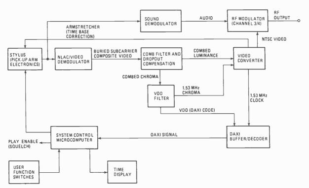
FIG. 12—SIGNAL PROCESSING CIRCUITS. This simplified block diagram shows the circuitry used to playback a CED videodisc.
