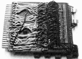
FIG. 3-UNDERSIDE VIEW REVEALS WIRING. The VIC-20 expander makes a good one-weekend project that will reward you with years of added convenience.
