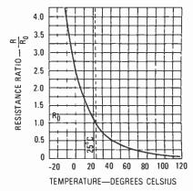
FIG. 1—NEGATIVE TEMPERATURE COEFFI-CIENT thermistors are very sensitive and highly nonlinear. Ro may be ohms, kilohms, or megohms.
