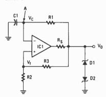
FIG. 8—A SIMPLE op-amp based squarewave generator.
