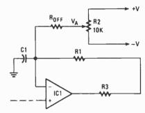
FIG. 11—ANOTHER WAY to generate a squarewave with an asymmetrical waveform is to use a potentiometer. The circuit shown here is another modification of the one shown in Fig. 8.
