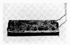
FIG. 10—TO ELIMINATE CROSSTALK, the inside of the case was lined with aluminum foil.
