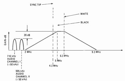
FIG. 10—CED SIGNALS. As shown here, the black level is at 5 MHz, which is the carrier frequency, the peak white is at 6.3 MHz, and the sync tips are at 4.3 MHz.
