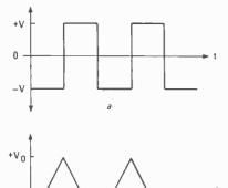
FIG. 13—TIMING DIAGRAM for Fig. 12. The squarewave, shown in a, is input to the Miller integrator; the resulting triangular waveform is shown in b.
