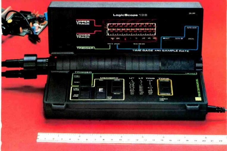
True Dual Trace • 10 MHz Real Time Bandwidth • 3 Input Channels • I/O Port Digital Waveform Storage • Boolean Waveform Operations • Audio Functions 8.25 (L) x 4.5 (D) x 1.75 (H) Inches • 1.25 Pounds • 9 Volt Battery/AC Operation
