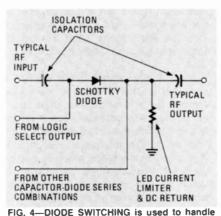
the RF switching in the Select-A-Matic. Because they can handle the frequencies involved, Schottky diodes are used.
