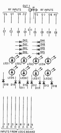
FIG. 9—PARTS PLACEMENT DIAGRAM for the I O boards. Note that only board 1 is shown; four I/ O boards in all are used by the project (see text).
