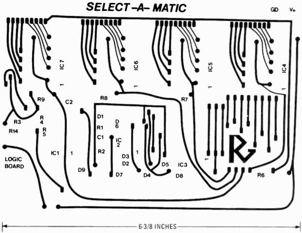
FIG. 5—COMPONENT SIDE of the double-sided logic board. The board is shown full sized.
