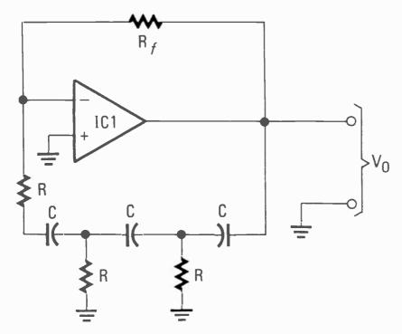
FIG. 15—AN RC phase-shift oscillator, such as the one shown here, can be used to generate a sinewave.
