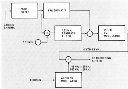
FIG. 11—THIS SIMPLIFIED BLOCK DIAGRAM shows the method used to record CED discs
