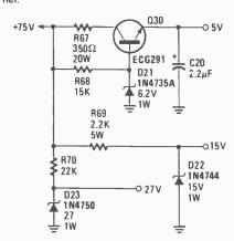
FIG. 15—THIS POWER SUPPLY is needed if the clipping indicators and bar-graph power meters are added. Note that Q30 requires a 10-watt heat sink.
