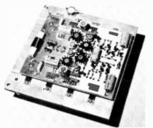
FIG. 9—AMPLIFIER BOARD is shown here mounted on heat sink. Note that Q12, Q13, Q15, and Q18 use TO-5 type heat sinks.
