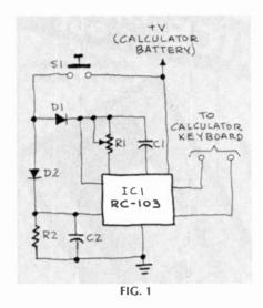
creased precision. Using the RC-103 along with a half-dozen common components and a simple calculator, you can build an instrument to measure resistance, capacitance, temperature, RPM, length, or angles. A stopwatch or a light meter may be constructed just as easily. So that you will know just how simple the whole thing can be, the basic circuit is shown in Fig. 1.
