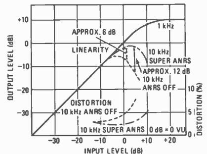
FIG. 9—RECORD/PLAYBACK linearity characteristics of cassette tape with and without Super-ANRS
