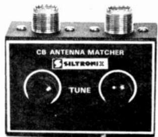
band. Most transceivers operate into 50-ohm loads, delivering maximum power with minimum distortion and harmonic radiation. A mismatch between antenna and transceiver occurs because the antenna impedance varies widely with frequency and physical location. The *Antenna Matcher* assures that the transceiver will be matched to the antenna at any time and on any channel with minimum harmonic radiation. Matches radio to antenna impedances of 35 to 150 ohms. Fitted with SO-239 connectors.
