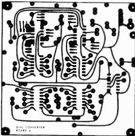
FIG. 3 (left)—PRINTED CIRCUIT pattern for Board-A shown half-size.
