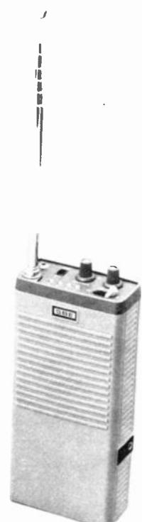
The model SB-11SM offers both low- and high-band VHF coverage from 30 MHz to 50 MHz and from 148 MHz to 174 MHz. It provides four-channel coverage and features LED channel indicator lights. Also featured are separate volume and squelch controls, switch for channel lockouts, a switch for manual scan of all four
