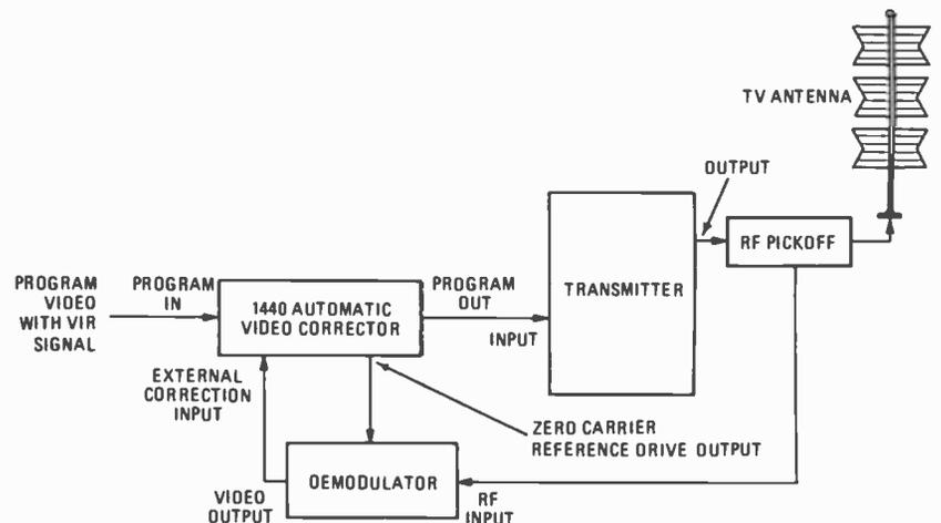
FIG. 3—COLOR SHIFTS due to transmitter distortion are corrected by negative feedback.
