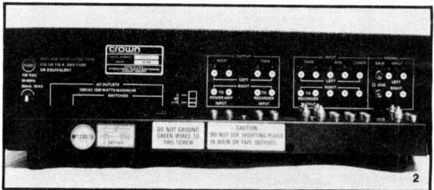
vertical surface for legibility. Near the pairs of PHONO inputs are screwdriver adjustment controls that permit you to vary the gain of the phono preamp section over a 20-dB range, with maximum sensitivity being 0.7 mV for rated output. In all of our subsequent tests, these controls were set to provide rated output (2.5 volts) from the main outputs with a phono input level of 2.5 mV. A slide-switch changes the gain by a fixed 10 dB.
