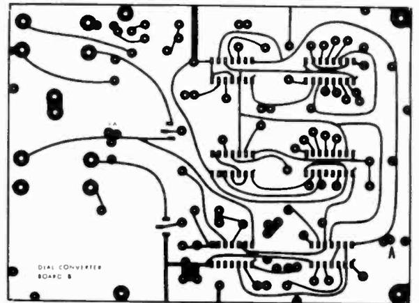
FIG. 4 (right)—PRINTED CIRCUIT pattern for Board-B shown half-size.
