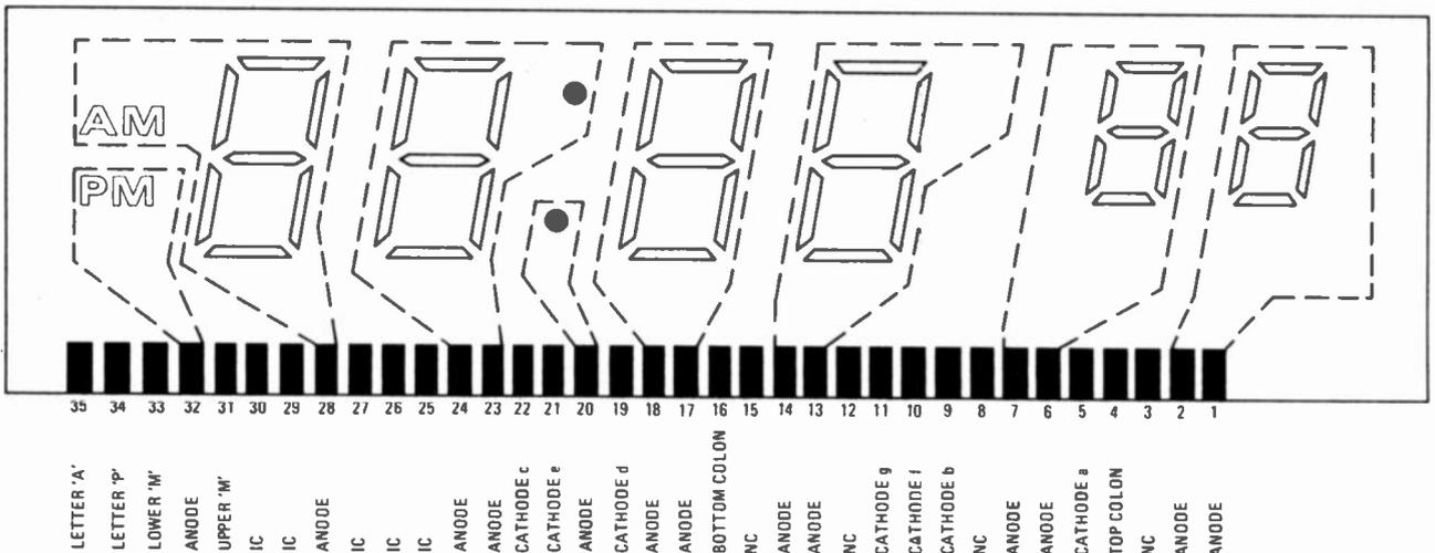
FIG. 2—PIN CONNECTIONS of the gas-discharge planar display.
