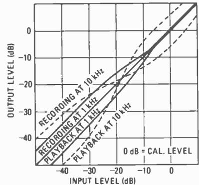
FIG. 8—INPUT/OUTPUT characteristics of the Super-ANRS circuit.
