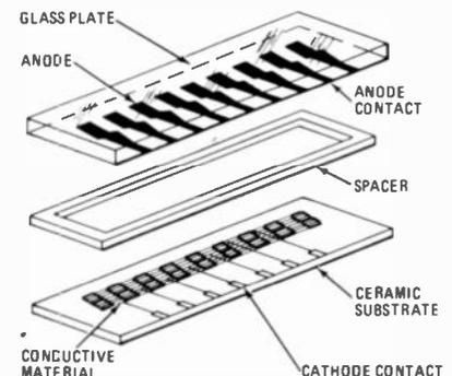
THIS GAS-DISCHARGE DISPLAY is a part of a digital clock you'll want to build. For details turn to page 67.
