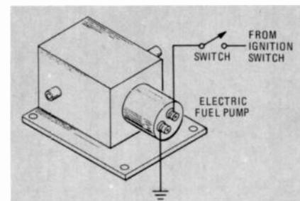
FIG. 4—FUEL-PUMP IMMOBILIZER operates by opening electric fuel-pump circuit.
