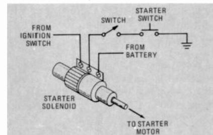
FIG. 3—STARTER IMMOBILIZER operates by opening starter-motor circuit.
