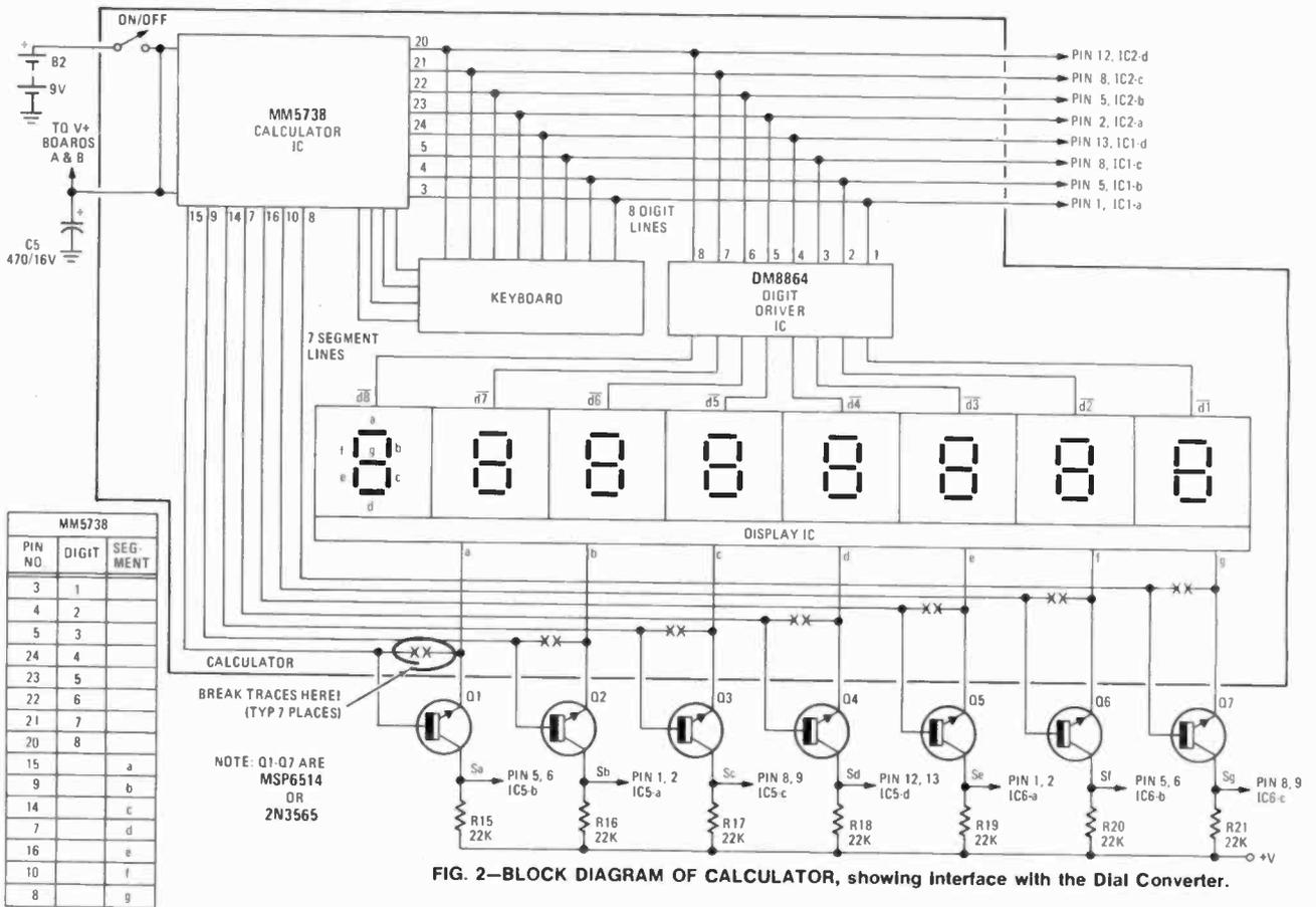
FIG. 2—BLOCK DIAGRAM OF CALCULATOR, showing interface with the Dial Converter.
