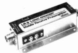
the receiver input, the LR-3 boosts received signals without in any way degrading the transmitted signal. A "sniffer" circuit senses the presence of transmitted RF signals and automatically causes the transmitted signal to bypass the receive preamplifier and be fed directly to the antenna.
