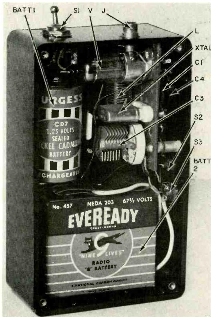
Interior view of transmitter. Notice unit is constructed on perforated panel.
