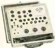
A deluxe tube tester that also tests diodes, rectifiers, fuses, pilot lamps, tube filaments.
