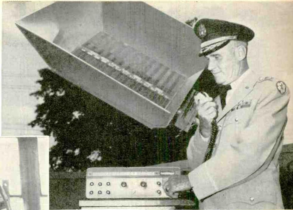
**SOLAR DISH** turns sunlight into 100 watts of electricity to power coast-to-coast radio network. Two stations were set up by Army Signal Research & Development Laboratory, one at Ft. Monmouth, N. J., and another at Los Angeles, Calif. The 20-square-foot solar dish came from Hoffman Electronics; transistorized transmitter-receiver from Hallcrafters.
