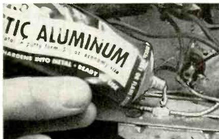
steel can be used as liquid metal for making wire anchors. Apply the liquid to the wire and to a spot on the chassis as shown. The liquid will dry metal-hard and hold the wire securely in place.—*James C. Conrad*
