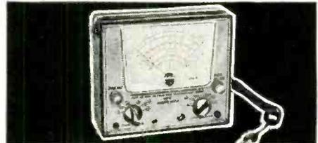
**EMC Model 107A - Peak to Peak Vacuum Tube Volt-Ohm Capacity Meter**—6" meter cannot burn out—entirely electronic. Measures peak to peak AC voltages to 2800 volts in 6 ranges. Measures capacity in 6 ranges from 50 mmfd to 5000 mfd. Measures resistance in 6 ranges from .2 ohm to 1000 megohms. Measures DC volts to 1000 volts in 6 ranges. Input resistance to 16.5 megohms. Wired ..... \$51.40 Kit ..... \$36.50
