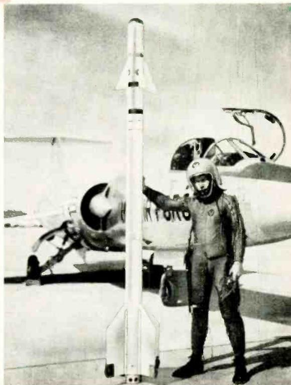
Fig. 6—The Sidewinder infrared-guided air-to-air missile. The detection equipment is all in the nose, above the black band.
