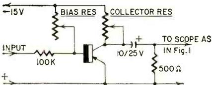
Fig. 4—Adding a resistance load to the transistor output changes the figures.
