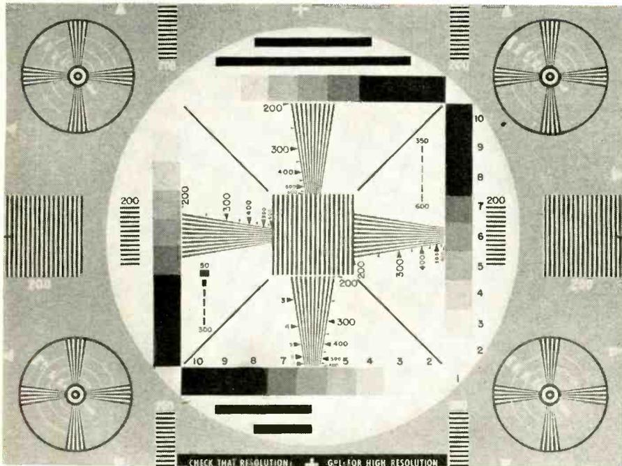
Fig. 3—Test chart used in adjusting the camera.
