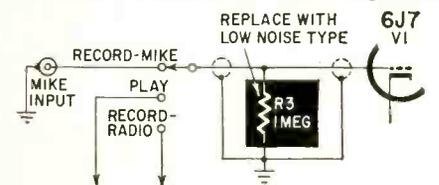
V1) with a deposited film or other relatively noiseless type of resistor. Do not overheat while soldering the replacement into position or it may become noisy also.—Lawrence Shaw
