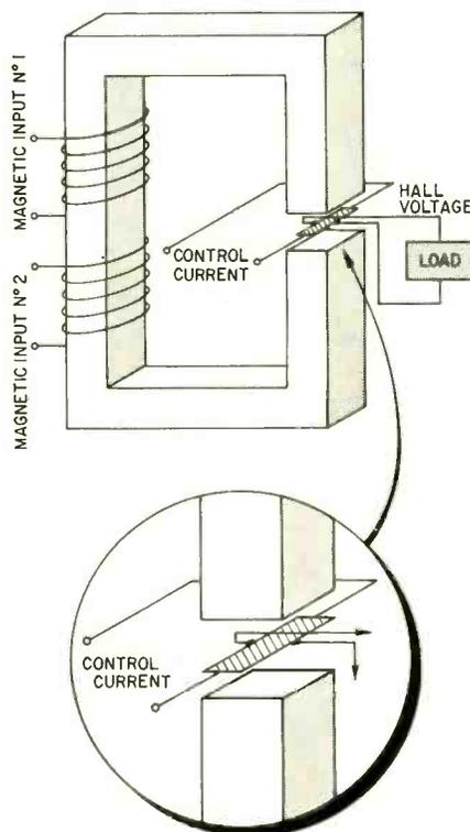
Fig. 2—Typical 2-coil magnetic circuit. The iron core concentrates the magnetic field on the Hall-effect device.
