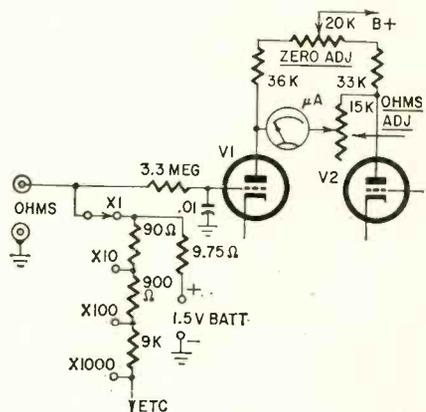
Fig. 3—In this vtvm ohmmeter circuit the 9.75-ohm resistor is normally the only one that burns out.
