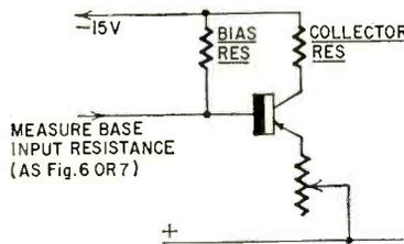
Fig. 10—Inserting emitter resistance linearizes base input resistance (and raises it) without affecting current gain. For voltage input it also linearizes gain distortion.
