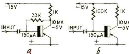
Fig. 9—Improved stability is obtained by using bias from collector (a) instead of the negative supply (b).
