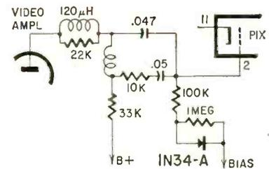
**Fig. 2—Simple dc restorer circuit uses a 1N34-A diode. Select diodes with back resistance of at least 750,000 ohms.**
