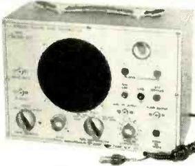
**EMC Model 107A Peak to Peak Vacuum Tube Volt-Ohm Capacity Meter**
