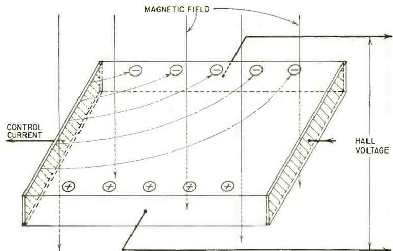
Fig. 1—Basic action of a Hall-effect device. The electrons supplied by the control circuit are deflected by the magnetic field to one side of the conducting slab. This leaves an excess of positive charges on the opposite side, thereby causing a voltage known as the Hall voltage, across the slab.
