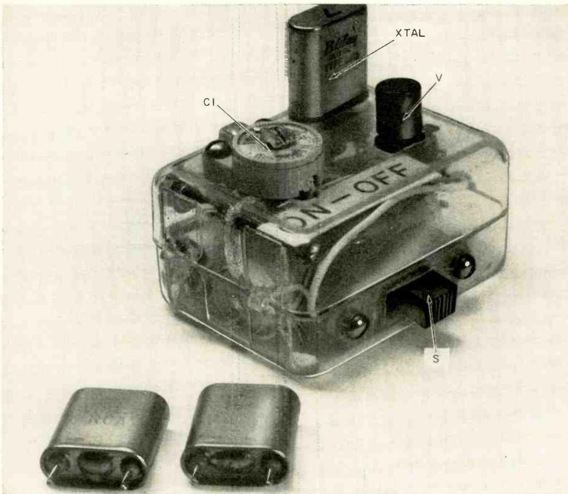
Slide switch turns the compact oscillator on and off.
