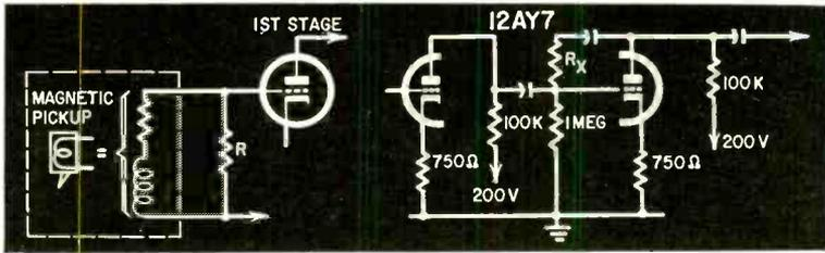
Fig. 7—For some magnetic pickups this arrangement will give the treble or high-end equalization.
