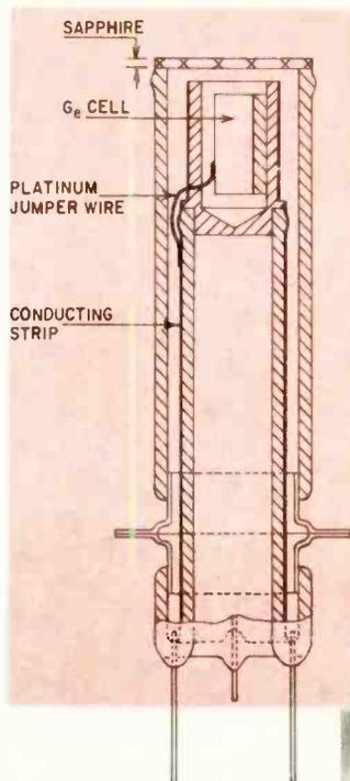
Fig. 4—Cross-section of the detector in Fig. 3.
