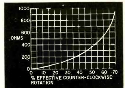
Fig. 3 — Taper of pot in meter leg of zero-adjust circuit.
