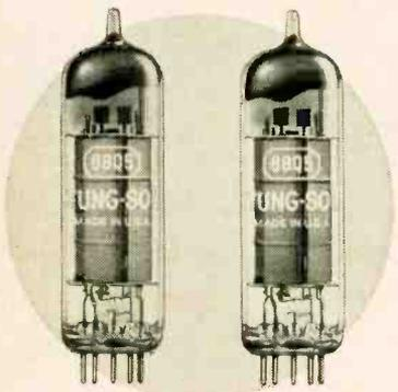
**6BQ5** Nine pin miniature power for low power requirements. Two in push-pull deliver up to 17 watts.
