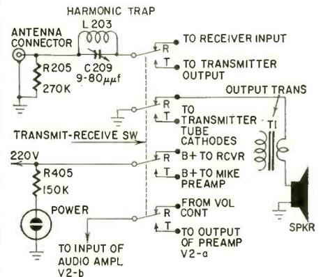
Fig. 2 — Transmit-receive switching circuits of the CB-1.
