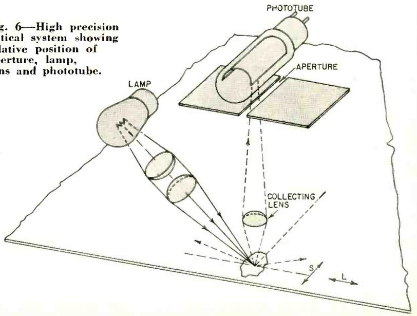
Fig. 6—High precision optical system showing relative position of aperture, lamp, lens and phototube.
