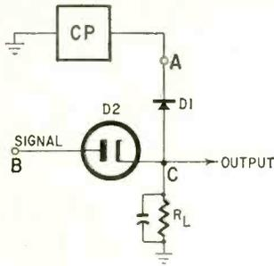
CP, so it does not conduct. At 3 μsec, a signal pulse (2 volts positive) is impressed. Since CP is zero at the time, it constitutes forward bias for D1. Thus the next CP causes a large reverse current through D1 and R<sub>L</sub>. With a
