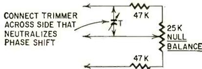
Fig. 3—Balance circuit modification eliminates phase shift between input and output.
