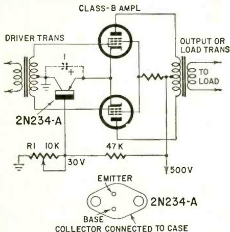
ply well-regulated bias to the class-B amplifier's cathode. The cathode voltage will be equal to the bias voltage, which should be adjusted with R1 for the particular tube being used. The transistor should be bypassed by a 1-μf capacitor (dashed lines) for hi-fi applications.—Bendix Semiconductors
