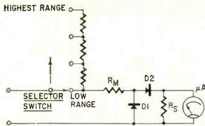
Fig. 6—Typical ac volts circuit.
