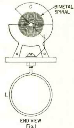
Fig. 1 shows a physical arrangement of the components. Fig. 2 is the corresponding diagram. When the tank is in tune, equal currents flow in L and C, so each bimetal spiral (BM) exerts the same force. Since the spirals are wound to
