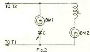
oppose each other, there is no net force. If the tank is off tune, more current will flow through L or C, as the case may be. Then C will tend to rotate until tuning is restored.
