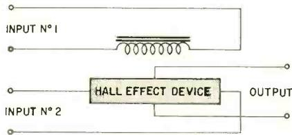
**Fig. 3—An electronic multiplier circuit. The output voltage is proportional to the product of the two inputs.**
