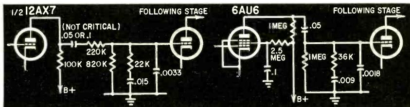
Fig. 5—A satisfactory design for a straight-forward equalizer circuit following a 12AX7 stage.
