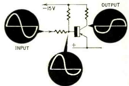
**Fig. 8—Relationship between distortions due to base input resistance and nonlinear amplification.**
