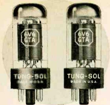
**6V6GT A** Bantam beam power amplifier with high power sensitivity and high power output with low supply voltages. Two in push-pull up to 14 watts.
