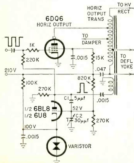
58). The diagram shows that only an additional triode is needed—here the triode section of a 6BL8 or 6U8.
