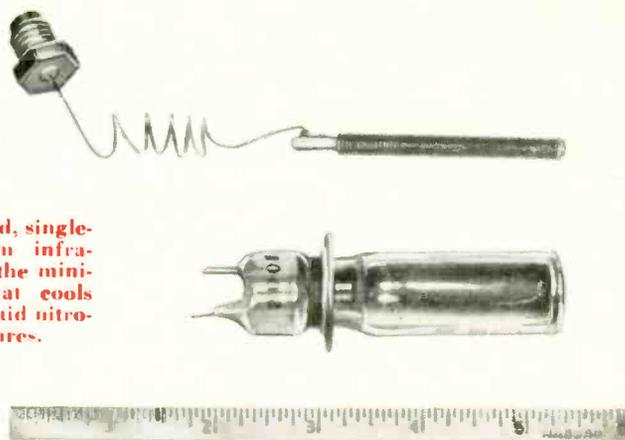
Fig. 3—Gold-doped, single-crystal germanium infrared detector with the miniature crystal that cools the detector to liquid nitrogen temperatures.
