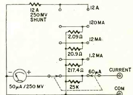
Fig. 5—Special circuit used to prevent contact resistance errors. The 2.09-, 20.9-, and 217.4-ohm resistors are frequently damaged.
