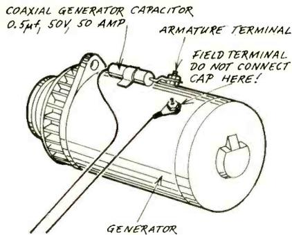
Fig. 2—Generator whine can be licked with a coaxial bypass capacitor.
