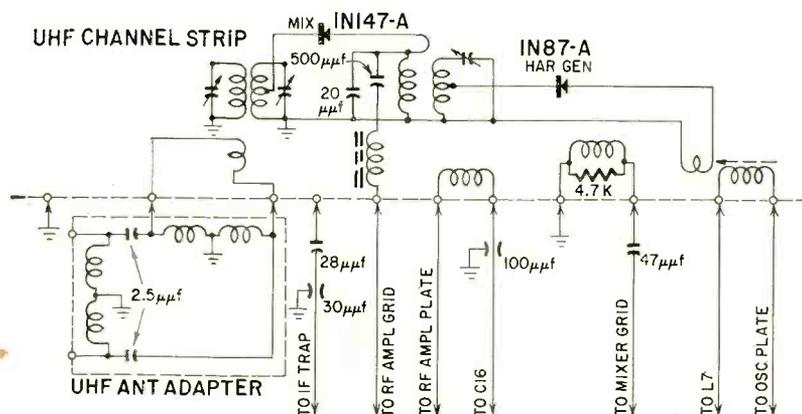
Fig. 3—A simplified circuit of a uhf tuner coil strip.
