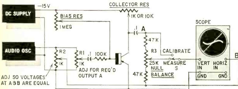
Fig. 1—Using scope balancing method to measure transfer distortion of unloaded transistor stage.
