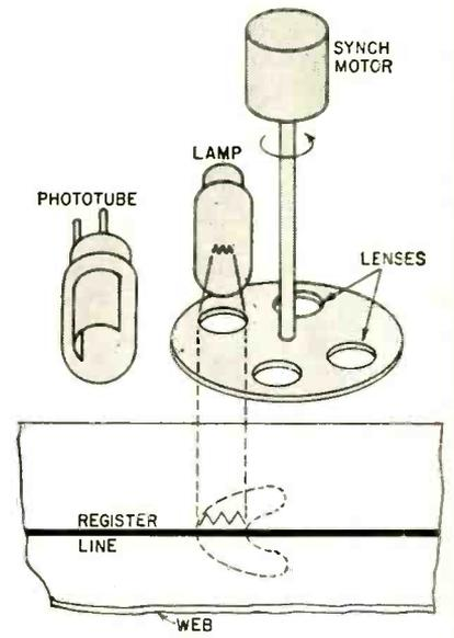
Fig. 5—Rotary lens web scanner.
