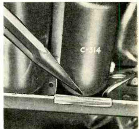
tubes removed, the chassis was wiggled out of the case—and the short vanished. Flexing the chassis would make the short come and go.
