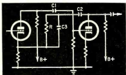
Fig. 12—Showing the method of using feedback over two stages.
