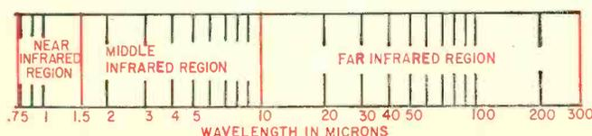
Fig. 1 — Infrared radiation spectrum showing the three infrared regions.
