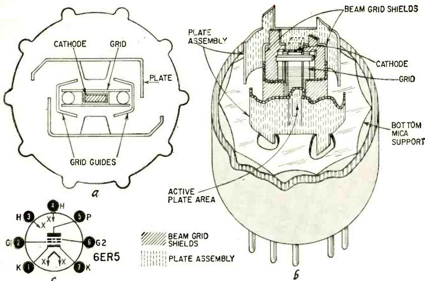
Fig. 2—Cutaway diagram shows construction of the Guided-Grid tube.
