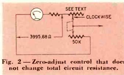
Fig. 2 — Zero-adjust control that does not change total circuit resistance.
