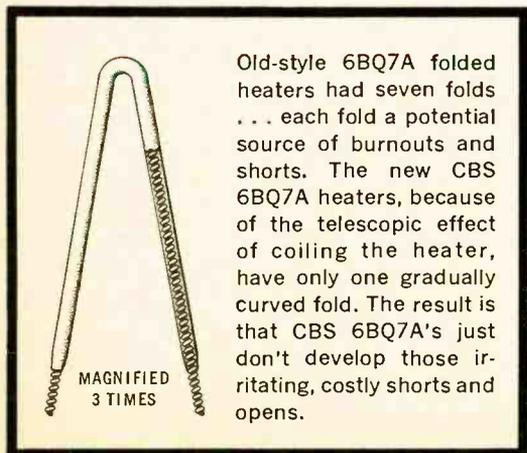
Old-style 6BQ7A folded heaters had seven folds . . . each fold a potential source of burnouts and shorts. The new CBS 6BQ7A heaters, because of the telescopic effect of coiling the heater, have only one gradually curved fold. The result is that CBS 6BQ7A's just don't develop those irritating, costly shorts and opens.
