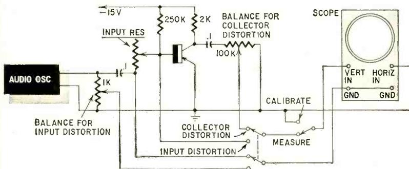
**Fig. 7—Measuring input current distortion and output distortion with sinusoidal input voltage.**
