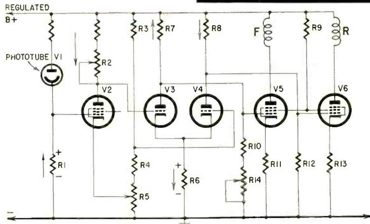
Fig. 10—Circuit of side register control CR7505-S119.
