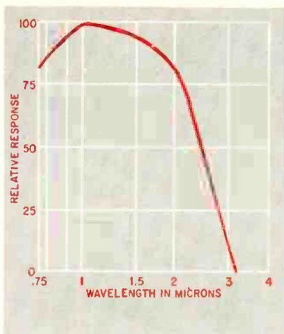
Fig. 2—Spectral response of a typical lead sulphide photocell.
