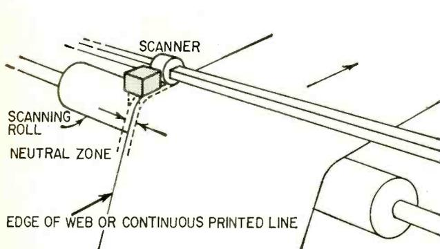
**Fig. 8—Two-point side register control system.**
