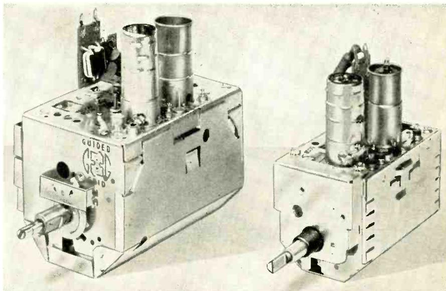
Miniature TV-tuner with Guided-Grid Neutrode circuit is on the right. It outperforms previous standard-sized version.
