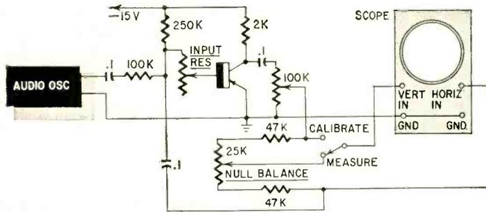
**Fig. 6—Measuring input-to-output distortion for voltage input with sinusoidal current.**
