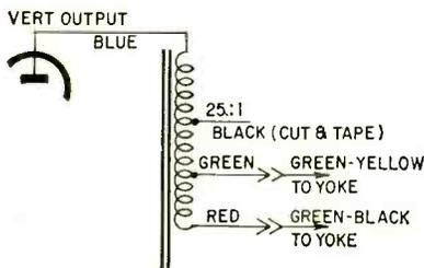
**Fig. 3—Correct connection for a Thordarson 26S55 replacement vertical output transformer in a Crosley G17TOMH TV receiver.**
