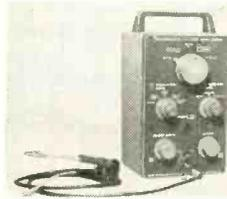
variable sweep width 200-kc to over 1 mc for if alignment. 100-kc markers each side of 10.7 marker. 10-mc crystal-controlled oscillator for calibration.—**Heath Co.**, Benton Harbor, Mich.
