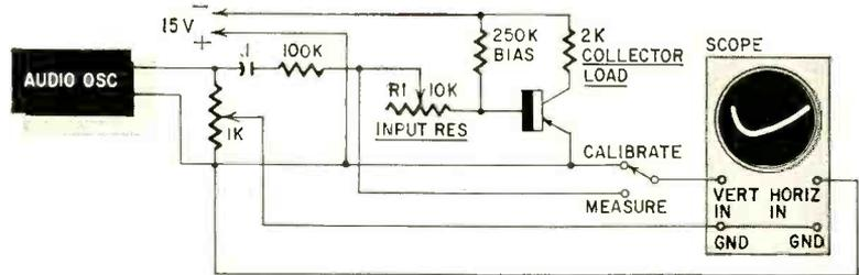
Fig. 5—Setup to measure the input base impedance with different series base resistors, on a sinusoidal current basis.
