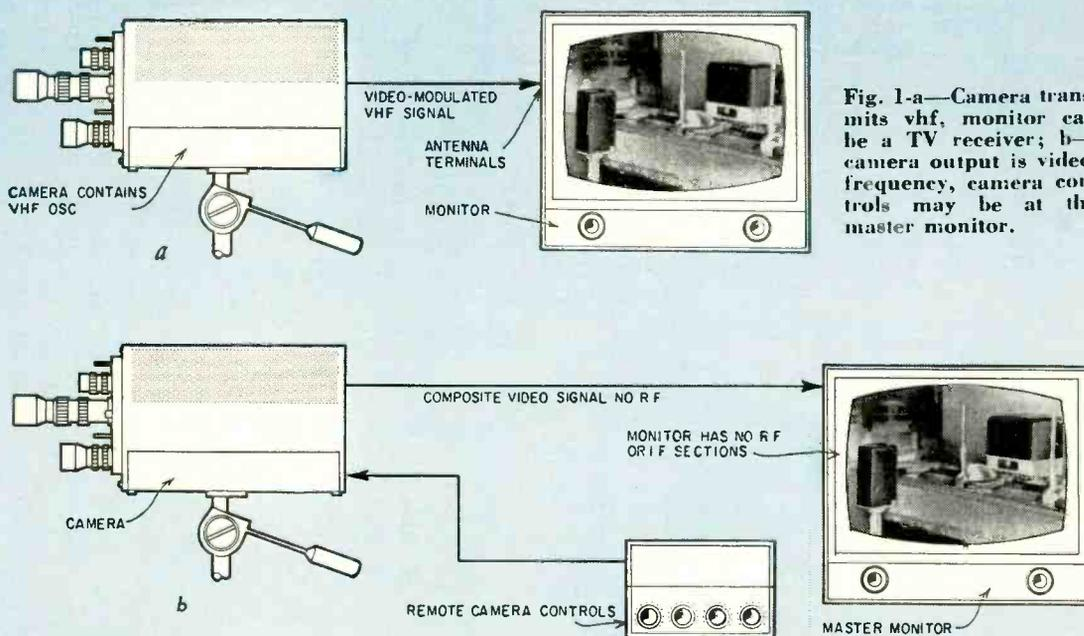
**Fig. 1-a**—Camera transmits vhf, monitor can be a TV receiver; **b**—camera output is video-frequency, camera controls may be at the master monitor.
