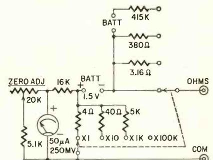
Fig. 2—Another common ohmmeter circuit. The 4- and 40-ohm resistors are usually the first ones to be damaged by overload.
