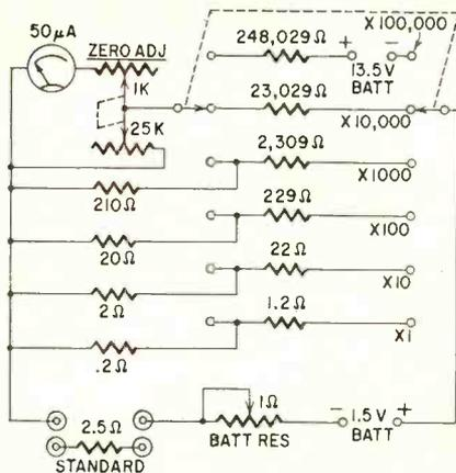
Fig. 6 — Semi-precision ohmmeter is somewhat easier to build than the unit shown in Fig. 4.
