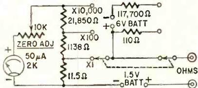
**Fig. 1**—In this type of ohmmeter circuit the 11.5- and 1,138-ohm resistor are most often damaged.
