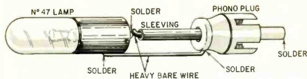
Fig. 3—A simple dummy-load antenna.
