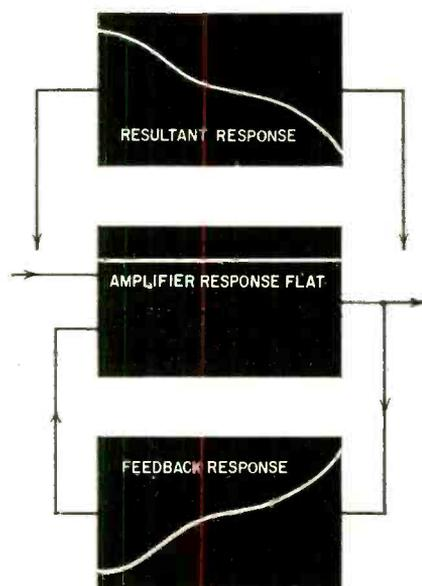
Fig. 3—Basic principle in design of feedback equalizers: Make the feedback response exactly the reverse of the equalization curve.
