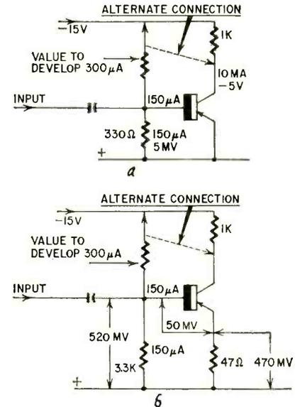
Fig. 11—How the use of an emitter resistance also aids the stabilizing problem by allowing the use of a practical value of base-to-ground resistance.
