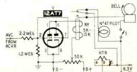
Fig. 1—Basic alarm circuit.
