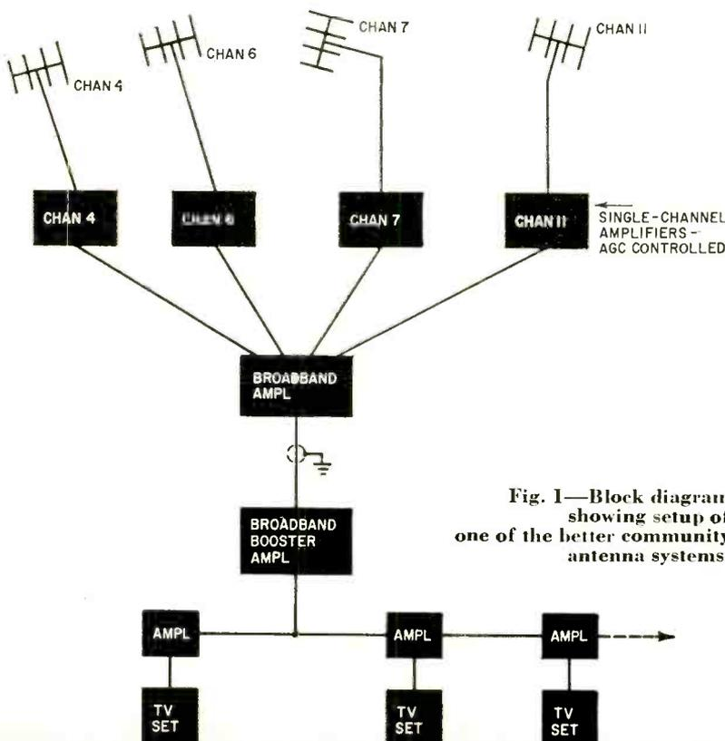
**Fig. 1—Block diagram showing setup of one of the better community antenna systems.**
