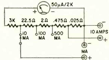
Fig. 4—If the milliampere ranges do not work and the circuit looks like this one, check the 0.475- and 2-ohm resistors first.
