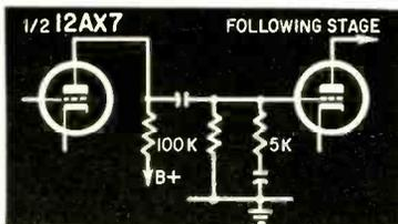
Fig. 4—The start of a design following a 12AX7 input stage. It is not completed because the 5,000-ohm load on the 12AX7 would cause an unacceptable amount of distortion.
