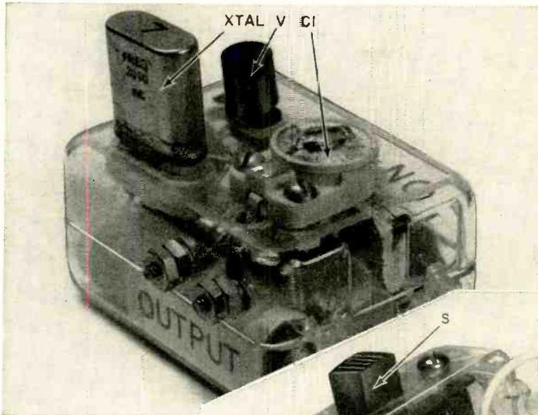
Output terminals are located on the rear of the case.
