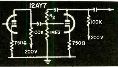
Fig. 8—A first try for a simple feedback equalizer using the two halves of a 12AY7.
