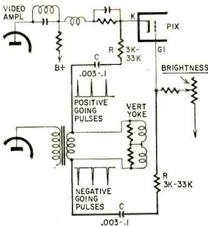
**Fig. 4—R-C network adds retrace elimination to a Transvision WRS-3.**
