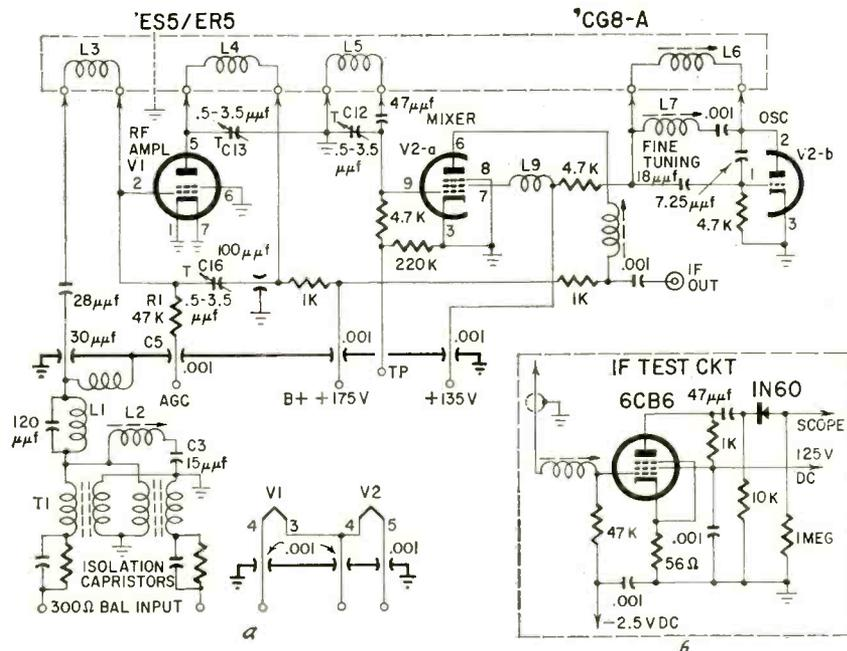
Fig. 1-a—Circuit of the Standard Coil vhf-uhf tuner; b—test circuit 7.25  $\mu\text{f}$  if strip.
