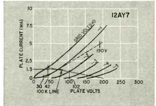
An alternative approach is to raise the effective grid circuit resistance. This will also, as mentioned earlier, help minimize any nonlinearity caused by the variation in plate resistance of the first stage. Assume that we use a 1-megohm resistor for the following grid and a 1-megohm resistor for the feedback as shown in Fig. 10. This will reduce the gain of the stage to about 28.
