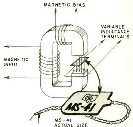
Ohio Semiconductors MS-41 uses a thin wafer of indium antimonide and has a high-field to zero-field ratio of 10 to 1 at 10 kilogauss. The MS-41 can be used in voltage-regulator, transducer, power amplifier and measuring circuits.
