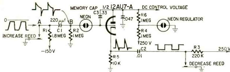
Fig. 5—Partial circuit of Magnavox remote control showing memory section
