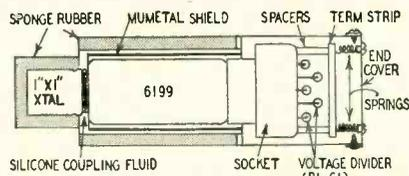
Fig. 2—Cross-sectional view of probe.
