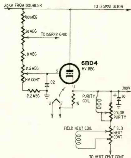
Fig. 2—Purity and field neutralizing controls in Westinghouse V-2284-15.
