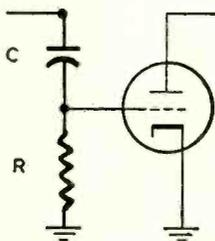
Fig. 9—Circuit for grid-leak biasing.
