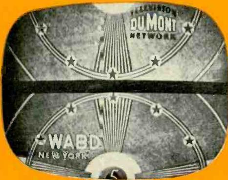
Fig. 1—Appearance of blanking signal.
