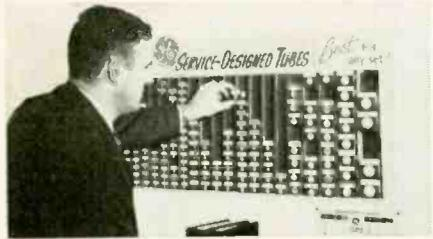
of visual tube inventory control by which the service technician can observe his tube requirements at a glance. The new *See-Lect-A-Tube* method features a dispenser unit which holds 250 tubes compactly.
