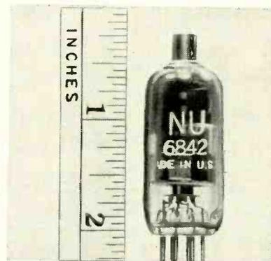
in a series regulator circuit in equipment that requires a stabilized voltage independent of line-voltage and load-current variations. The 6842 (see photo) can provide up to 10-ma average plate current and dissipate approximately 8 watts.
