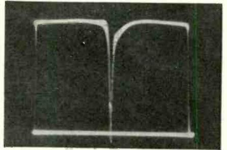
Fig. 8—Reducing sweep width shows details of zero-frequency point in Fig. 7.
