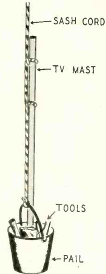
in the bucket and throw a couple of half-hitches of line around the other end. Carry the line to the roof and haul away. See drawing. It's easy to hoist antennas in cartons this way too.
