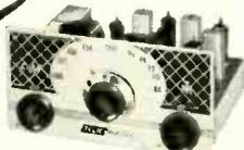
Self-contained power supply • Tuning range 87-109 Mc • 200kc IF bandwidth • Grounded-grid RF stage • AFC with front-control cutoff • Microvernier tuning • No-drift ratio detector • 4 uv sensitivity for 20 db quieting • Standard de-emphasis network • .8 volt RMS cathode-follower output • 3.2 volt RMS high-impedance output • 300 ohm input impedance • Switch-controlled AC receptacle for auxiliary equipment.
