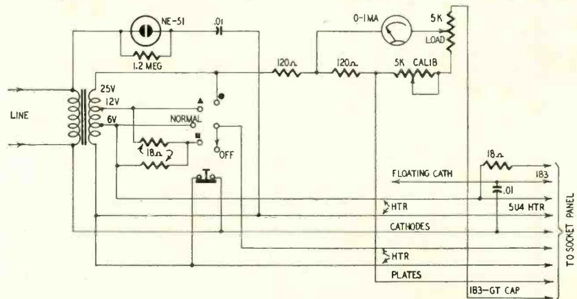
Fig. 1—Simplified schematic diagram of the model TV-20 tube tester.
