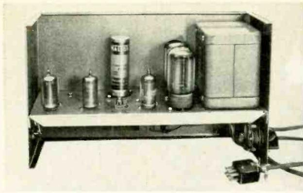
*Unit provides triode, pentode and Ultra-Linear operation*
