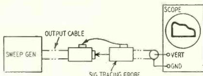
Fig. 5—Checking generator output for flatness—ground lead must be short.
