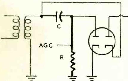
Fig. 8—Diode circuit for agc takeoff.
