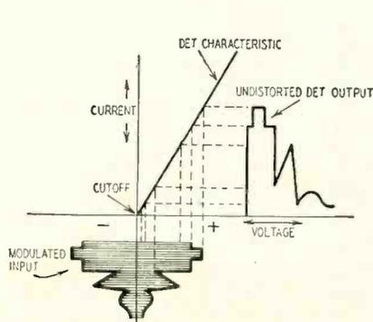
Fig. 2—Undistorted detector output.
