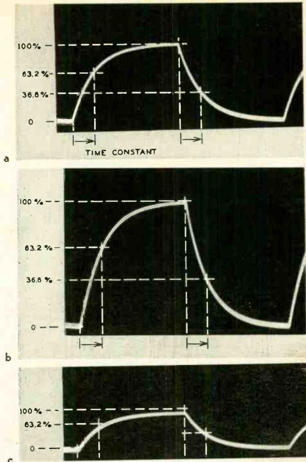
Fig. 4—Waveforms show that changes in voltage do not affect a time constant.
