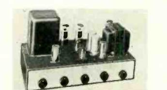
(1/4 watt) ±0.5 db 13 to 35,000 cycles, ±1.5 db 7 to 50,000. IM distortion (60 cycles and 6 kc, 4:1, 20 watts.) 1.3%; mid-band harmonic distortion 0.3%; maximum harmonic distortion (between 20 and 20,000 cycles at 1 db below 20 watts) 1%. Speaker taps 4, 8, and 16 ohms.—Electronic Instrument Co., Inc., 84 Withers St., Brooklyn 11, N.Y.
