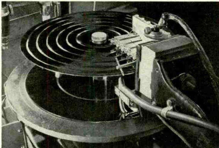
Fig. 3—The recording system. Six pickups on upper record pick up and mix signals to be combined into a single recording on the lower disc.
