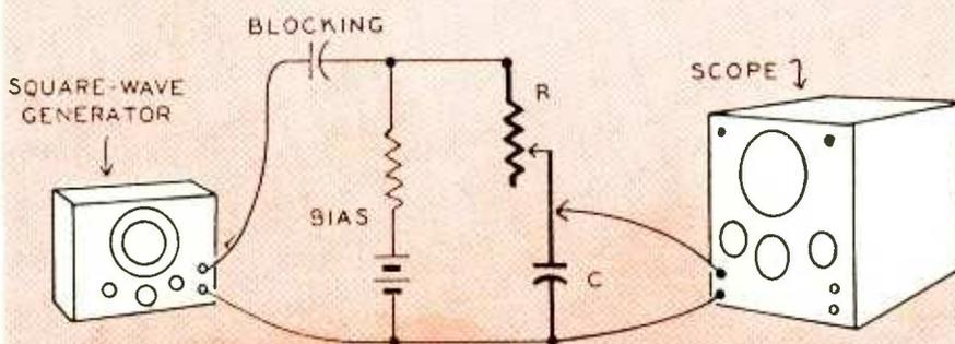
Fig. 1—Setup for time-constant study.
