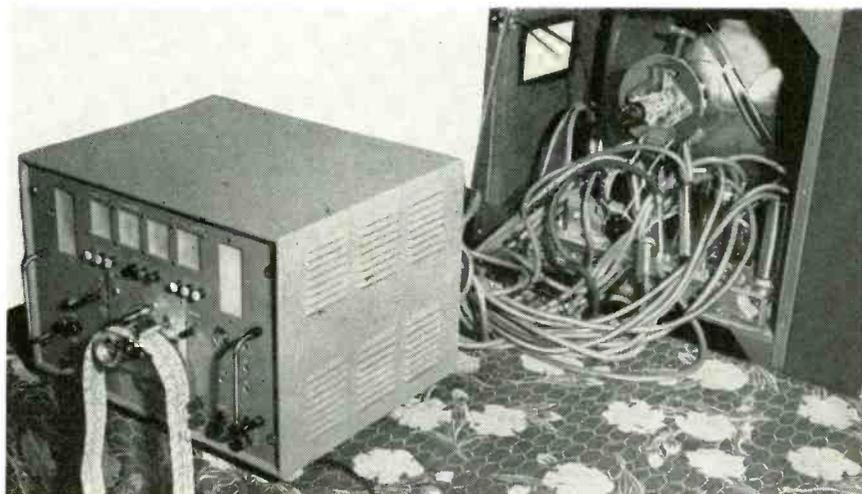
punched tape to program test points and parameters. It performs up to 120 complete circuit measurements per minute and has a capacity of 240 test points per setup. There are over 57,000 possible measurements or tests per setup. Excluding tubes or gross breakage through a dropped or smashed chassis, the instrument will pick up 70-90% of failures or defective parts.
