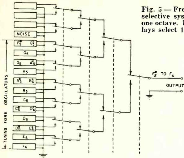
Fig. 5 — Frequency-selective system for one octave. Four relays select 12 notes.
