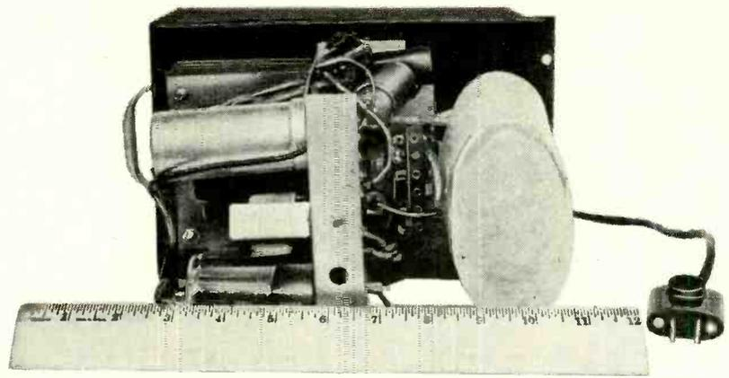
Fig. 2—Rear view shows plastic cover over the voltage-doubler assembly.
