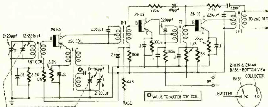
The 2N140 is mechanically like the 2N139 but has characteristics which especially meet the requirements of converter and mixer-oscillator applications in the standard AM broadcast band. In typical operation in a common-emitter circuit (see diagram) the 2N140 features a conversion power gain of 27 db at 1 mc. The circuit is sufficiently stable to permit changing transistors without readjusting the oscillator.
