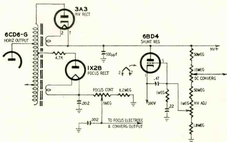
Fig. 1—Diagram of the high-voltage and focus adjustments in the RCA CTC2.
