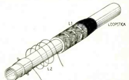
Fig. 2—Windings on the loopstick.
