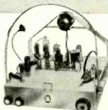
Super-selective 12-channel turret tuner • IF section completely wired and aligned • 9 microvolt sensitivity • 3-stage stagger-tuned IF • AGC • Synchro-guide AFC with horizontal hold • Ceramic core horizontal output xmfr with beam power amplifier. For L.V. electrostatic kines 17"—21".
