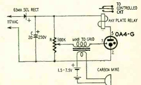
Fig. 1—Diagram of basic controller. Relay locks in when tube is fired.
