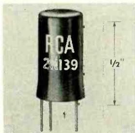
The 2N139 (see photo) designed especially for 455-kc applications, can provide a power gain of 30 db at 455 kc in suitable common-emitter circuits (see diagram). It has excellent stability, low collector cutoff current, is only 0.26 inch in diameter and has a seated height of 0.495 inch.
