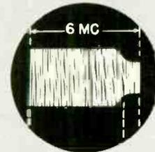
Note flatness throughout specified range; to 3.6 mc down 1.5 db, at 4.5 mc down 3 db, at 6 mc down 6 db.
