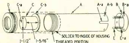
A—MAIN PROBE HOUSING; A-a—SLIT FOR COAX LEADS 1/8" X 15/16"; A-b—MOUNTING HOLES FOR COVER (3/12" TAP)
