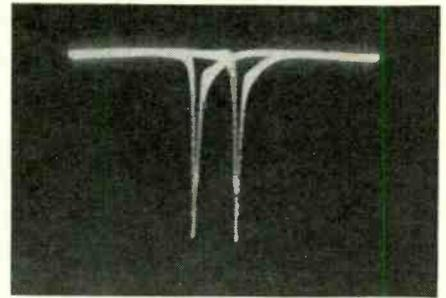
Fig. 7—Unblanking the retrace in Fig. 6 shows dissymmetry in the generator.
