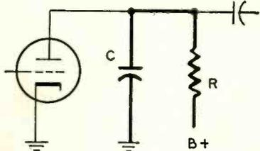
Fig. 10—A basic sawtooth generator.
