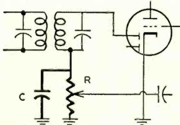
Fig. 7—Basic diode detector circuit.
