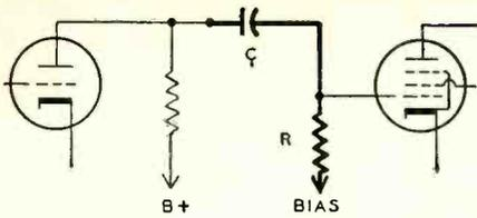
Fig. 6—A resistance-coupled amplifier.
