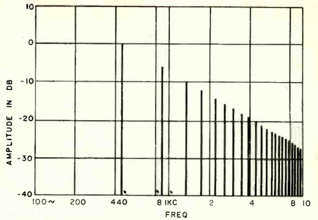
Fig. 6—Harmonics of 440-cycle sawtooth. Harmonics extend to infinity with ever-decreasing amplitudes.
