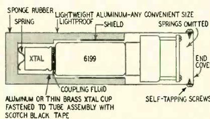
Fig. 3—Diagram of a simplified probe.
