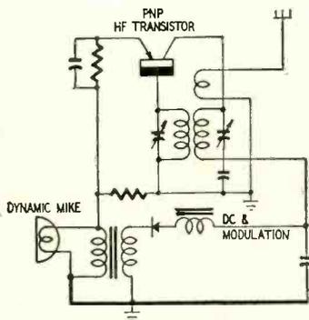
The microphone is a moving-coil or armature type, transformer-coupled to the tuned-base tuned-collector type rf oscillator. Operating voltage for the transistor is developed by rectifying the af signal at the secondary of the
