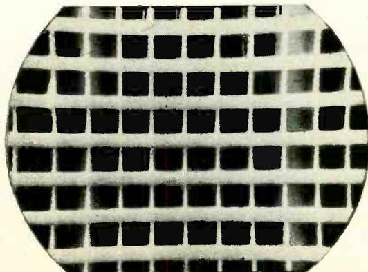
Fig. 9—Typical cross-hatch pattern.
