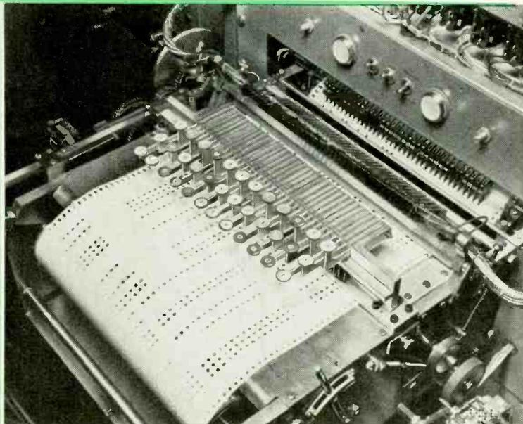
Fig. 2—Keyboard of the Electronic Music Synthesizer. Keys punch the tape. Brushes behind keys pick up music code.
