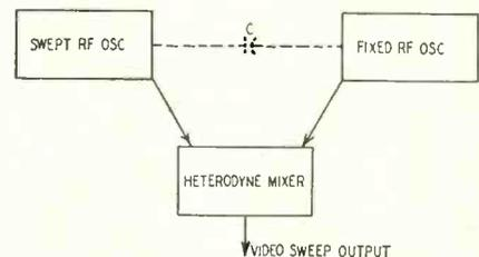
Fig. 9—Diagram shows basic arrangement for a beat-frequency sweep generator.
