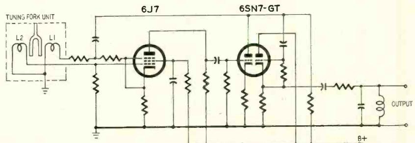
Fig. 4—The tuning-fork oscillator. L1 is the driver; L2 controls frequency.
