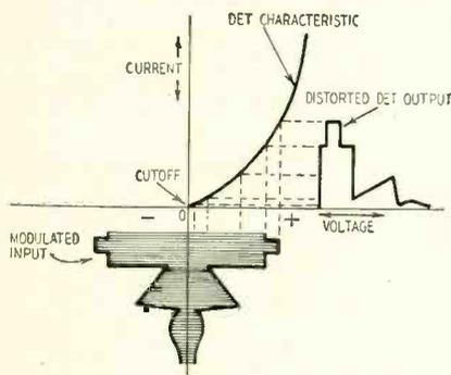
Fig. 1—Crystal detector characteristic.
