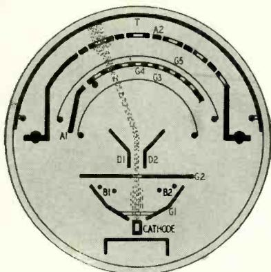
Fig. 1—Internal construction of EIT.
