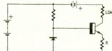
rent flowing through it. Therefore, in the diagram shown, the emitter-to-base bias on the transistor remains constant.
