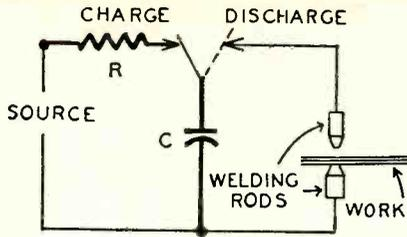
Fig. 12—An electronic spot welder.
