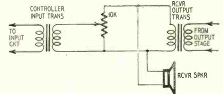
Fig. 4—Diagram shows controlling signal taken from radio or amplifier.
