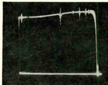
Fig. 3—Video sweep response. A 4.5-mc marker in center of pattern—spurious markers are above and below this point.
