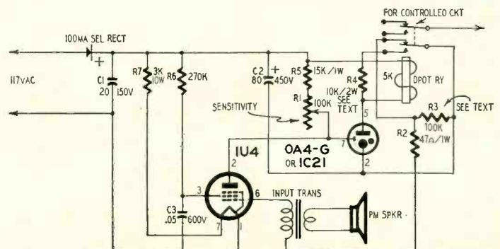
Right—Fig. 3—Circuit of Fig. 2 with a stage of amplification added to it.
