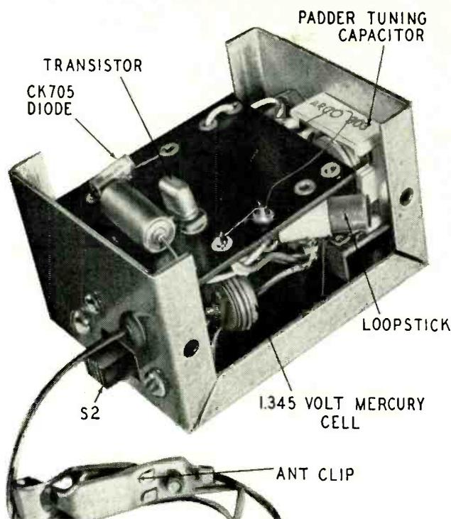
Internal view of solar-powered radio.
