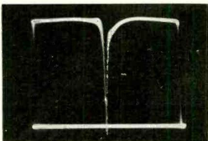
Fig. 6—The zero-frequency point is brought to center of the sweep trace.
