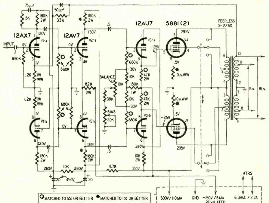
Fig 2—Schematic diagram of amplifier. Switch selects output tube operation.
