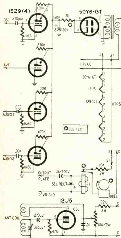
Schematic of set tester — instrument operates from an isolation transformer.
