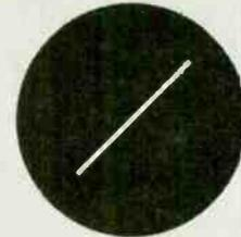
Phase shift between horizontal-vertical amplifiers, 0-500 kc-0°, to 1 mc within 2°; by internal adjustment with gain controls at max 0° phase shift possible on any specific frequency to 6 mc.
