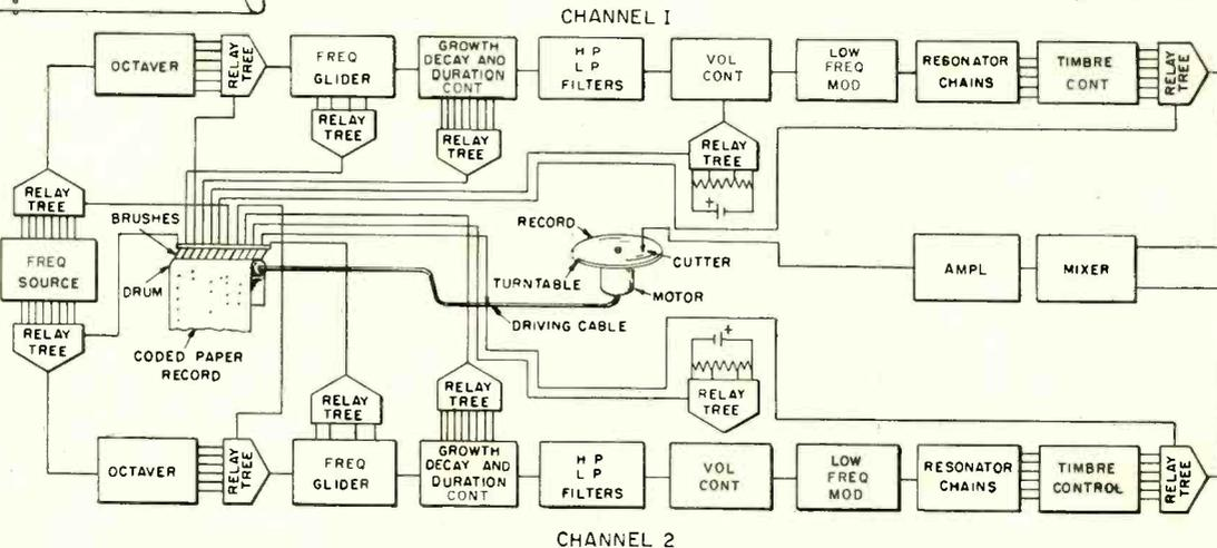
smooth glide is characteristic of some instruments (such as the trombone or violin). In others, the transition is made in a series of successive approximations. The instrument provides either type of portamento.
