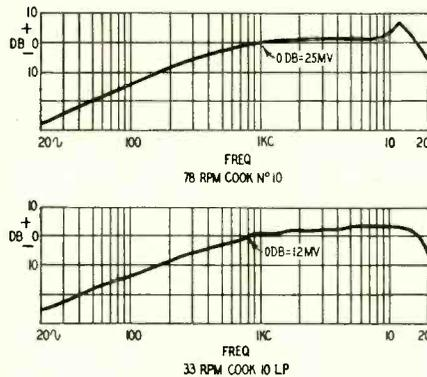
Fig. 2—Unequalized response of Recoton cartridge feeding an audio vtvm.
