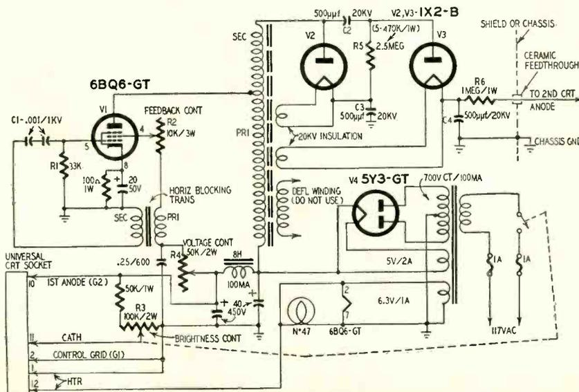
Fig. 1—Schematic diagram of complete supply—high voltage can be varied.
