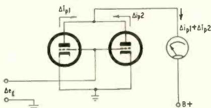
Fig. 5—Measuring  $g_m$  of dual tubes.
