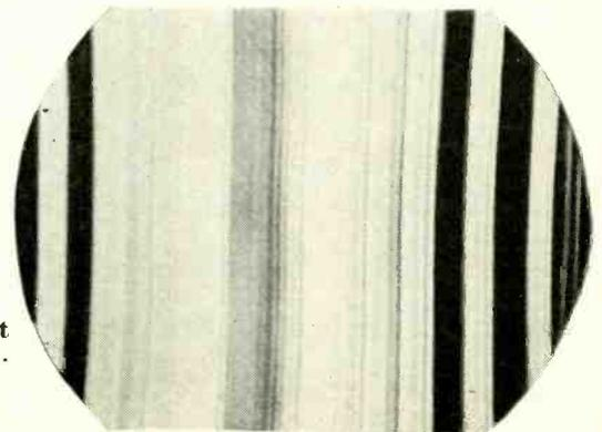
Fig. 8—Incorrect color bar pattern.
