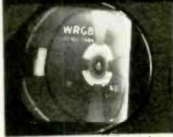
FAULT—Picture compression and stretching.
