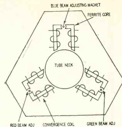
Fig. 4—A typical convergence yoke.
