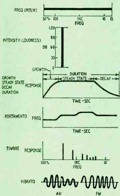
Fig. 1—All sounds can be broken down into components shown in the charts.
