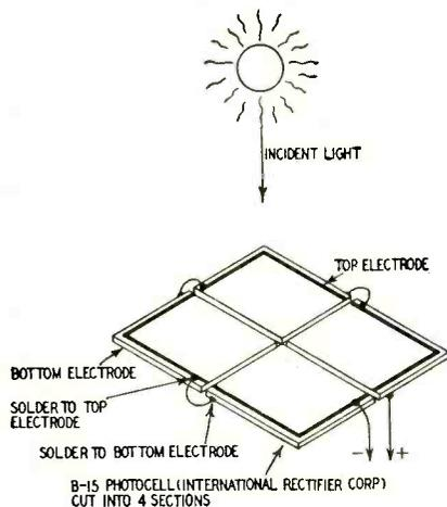
Fig. 3—Details of the solar cell.
