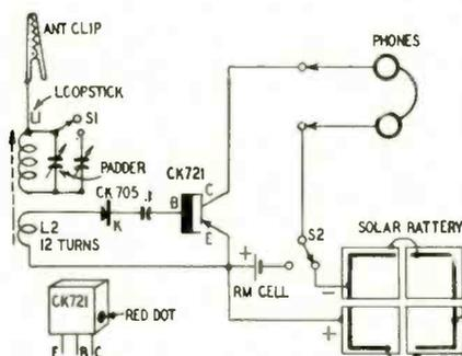
Fig. 1—Schematic of the receiver.
