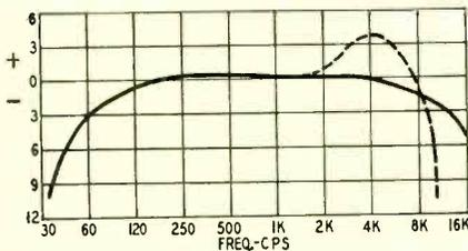
Fig. 1—Responsive curves. Solid line—authors circuit; dotted line—A.C.A.
