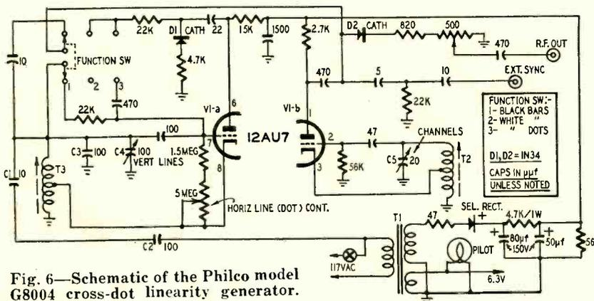
Fig. 6—Schematic of the Philco model G8004 cross-dot linearity generator.
