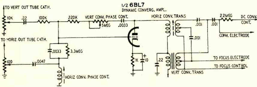
Fig. 10—Dynamic convergence circuit. Output is fed to convergence electrode.
