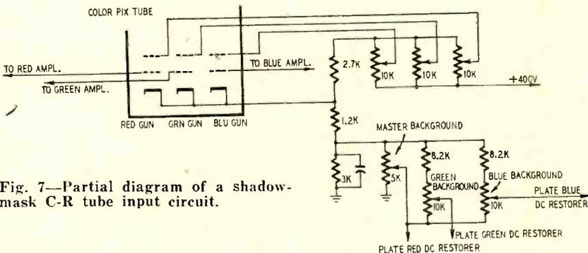
Fig. 7—Partial diagram of a shadow-mask C-R tube input circuit.
