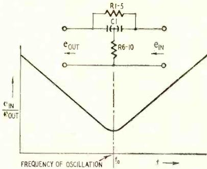
Fig. 2—Bridged-T characteristics.
