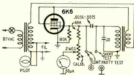
Fig. 4—Flyback transformer tester.
