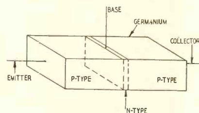
Fig. 1—A p-n-p junction transistor.
