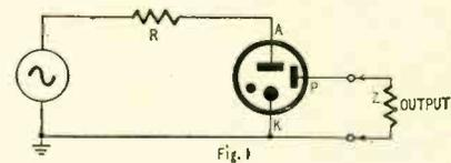
Fig. 1 shows a circuit using a triode gas tube. Input is applied between anode A and cathode K. A third element is shown at P, a probe which conducts the output current. The load is Z, a high impedance so that there will be negligible loading of the circuit. During nonconduction, P is at ground potential. When the tube is excited
