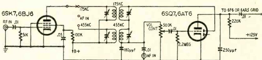
selector switch from the detector input to the plate of the single r.f. amplifier. I saved one switch section by connecting the transformer secondaries in series as shown. The changes in the audio circuit consisted of adding a .01-µF capacitor between the a.f. input jack and the volume control and bypassing the first a.f. amplifier plate
