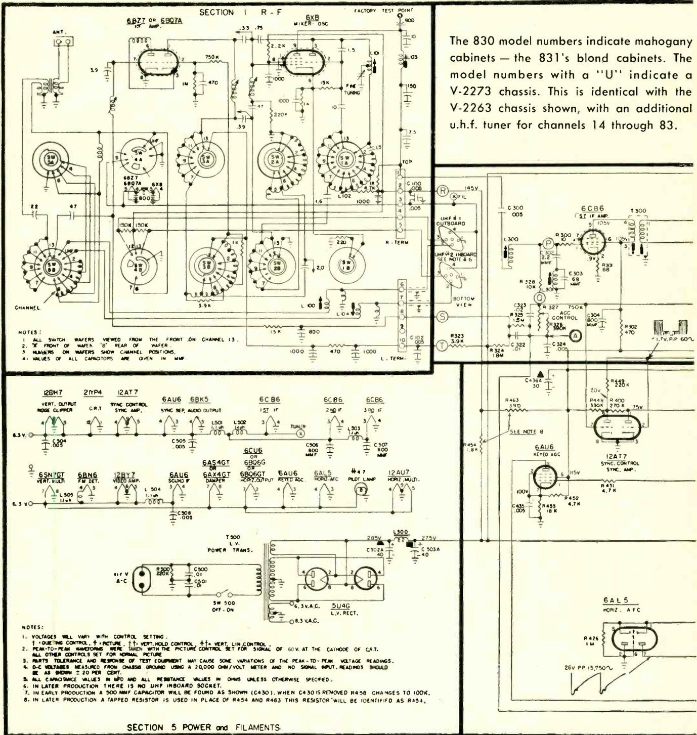
The 830 model numbers indicate mahogany cabinets — the 831's blond cabinets. The model numbers with a "U" indicate a V-2273 chassis. This is identical with the V-2263 chassis shown, with an additional u.h.f. tuner for channels 14 through 83.
