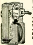
Sturdy shaded pole A.C. induction motor. 15 watts, 3000 rpm. 3 7/8" x 1 1/4". 4 mounting studs; 7/8" shaft, 3/16" diameter; 110-120 volts, 50-60 cycles. A.C. only. When geared down, this unit can operate an 18" turntable with a 200 lb. dead weight. Use it for fans, displays, timers and other purposes. Ship wt. 2 lbs.
