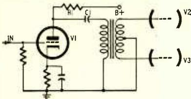
Fig. 2—Shunt-fed driver transformer.
