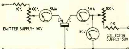
Fig. 9—"Tube tester" for transistors.
