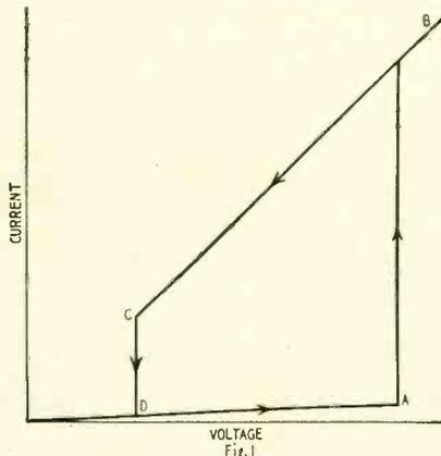
point C at which snap action again takes place. The current drops off sharply to the original point D.
