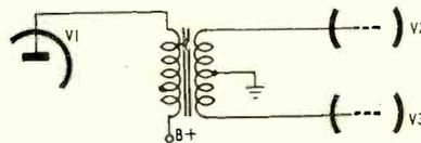
Fig. 1—Simple type of phase splitter—the center-tapped transformer.
