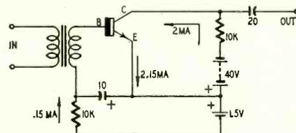
Fig. 4—Practical transistor hookup.
