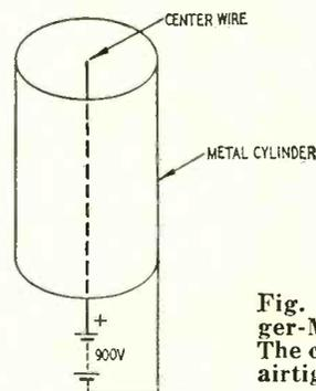
Fig. 1—Basic Geiger-Mueller tube. The cylinder has an airtight seal.
