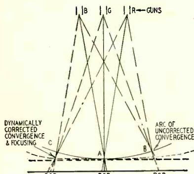
Fig. 9—Shadow-mask tube convergence.
