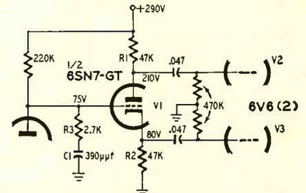
Fig. 4—Split-load phase splitter.
