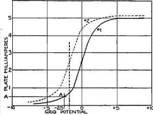
Figure 20.—Characteristic curve of vacuum tubes to show effect of biasing.
