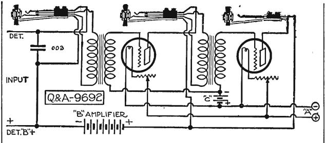
wave length range can be overcome by one hundred turn honeycomb coils in primary, secondary and tickler.
