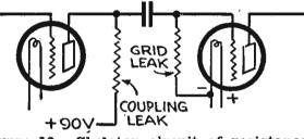
Figure 19.—Skeleton circuit of resistance coupled amplifier showing leaks used as coupling device as well as grid leak.
