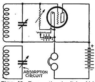
Figure 18.—Regenerative circuit in which leak must connect direct to filament since inductance is at plate potential.
