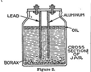
dissolve has settled on the bottom; this should be removed. Fill each jar to about one inch from the top and pour a small quantity of oil on to keep the water from evaporating too quickly.
