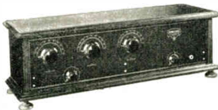
AMBU FIVE. Manufactured by the Ambu Engineering Institute, 2632 Prairie avenue, Chicago, Ill. Five tube receiving set with sub-panel inlaid with copper that has been shot into prepared grooves for automatic connections. Three sets of three interchangeable coils covering 40 to 550 meters. Three tuning dials and two filament controls. Loud speaker jack on front panel. List price $75.00.
