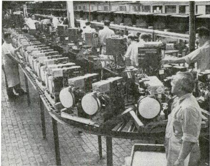
Partially completed television receivers travel down the factory production line.
