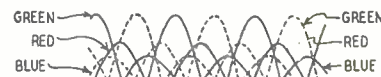
Fig. 9—Overlap of colors is shown here of the Du Mont Trichroscope 6 , a tube with three electron guns and a face made up of minute three-sided pyramids, each side of which is coated with a phosphor in one of the three
